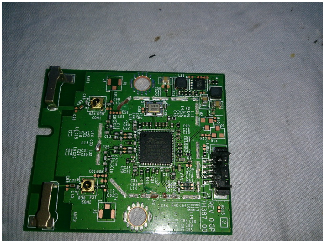
FIGURE 27 LED LCD TV (M/N: 75H9) RF BOARD (SHIELDED SHELL REMOVED)
