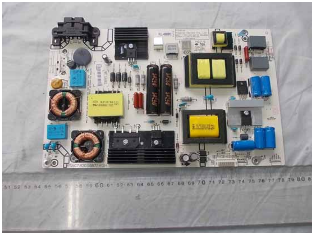
FIGURE 3 LED LCD TV (M/N: 50H5G) POWER BOARD (COMPONENT SIDE)
