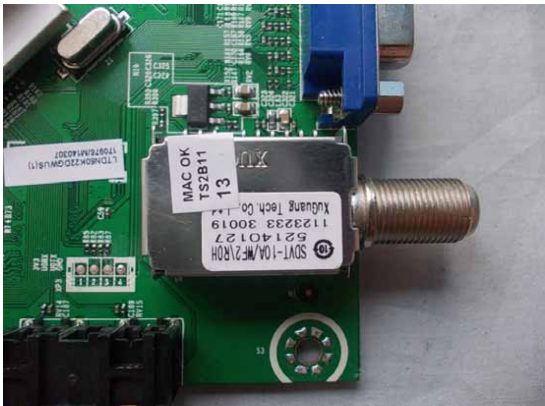
FIGURE 10 LED LCD TV (M/N: 50H5G) TUNER ON MAIN BOARD
