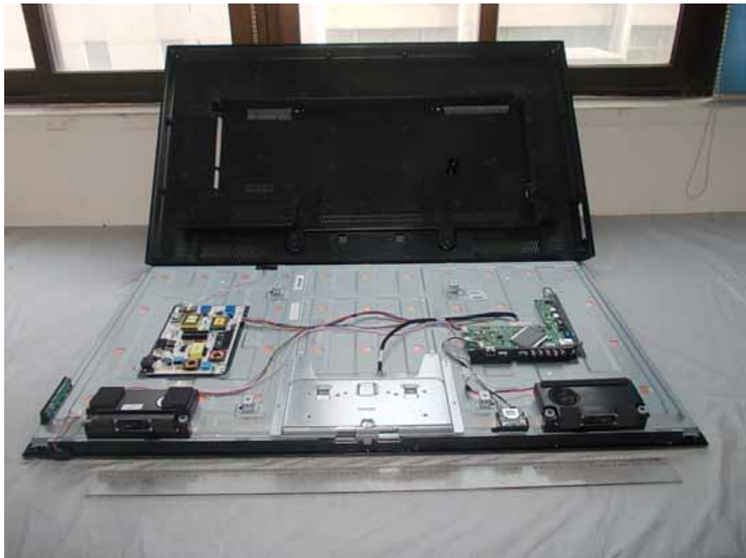
FIGURE 1 LED LCD TV (M/N: 50H5G) COVER REMOVED
