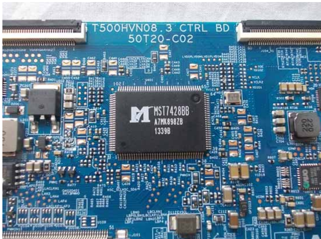
FIGURE 17 LED LCD TV(M/N: 50H5G) CHIP& CRYSTAL ON LCD PANEL CONTROL BOARD
