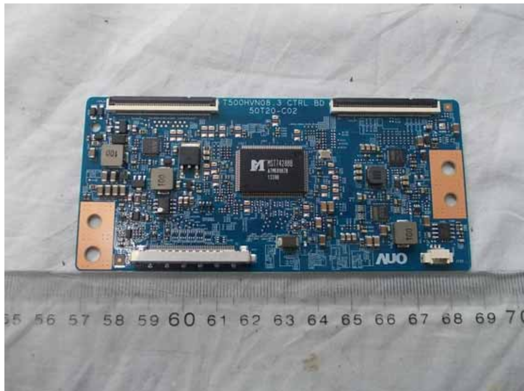
FIGURE 15 LED LCD TV (M/N: 50H5G) LCD PANEL CONTROL BOARD (COMPONENT SIDE)
