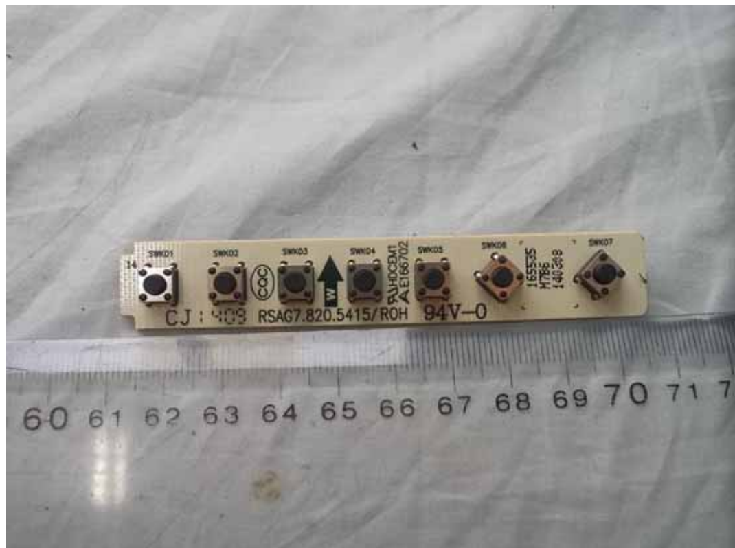
FIGURE 11 LED LCD TV (M/N: 50H5G) KEY BOARD (COMPONENT SIDE)
