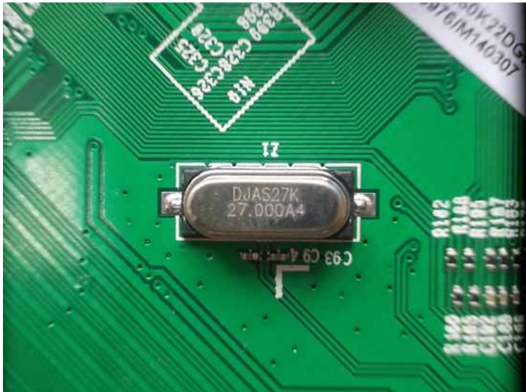
FIGURE 9 LED LCD TV (M/N: 50H5G) CRYSTAL #2 ON MAIN BOARD
