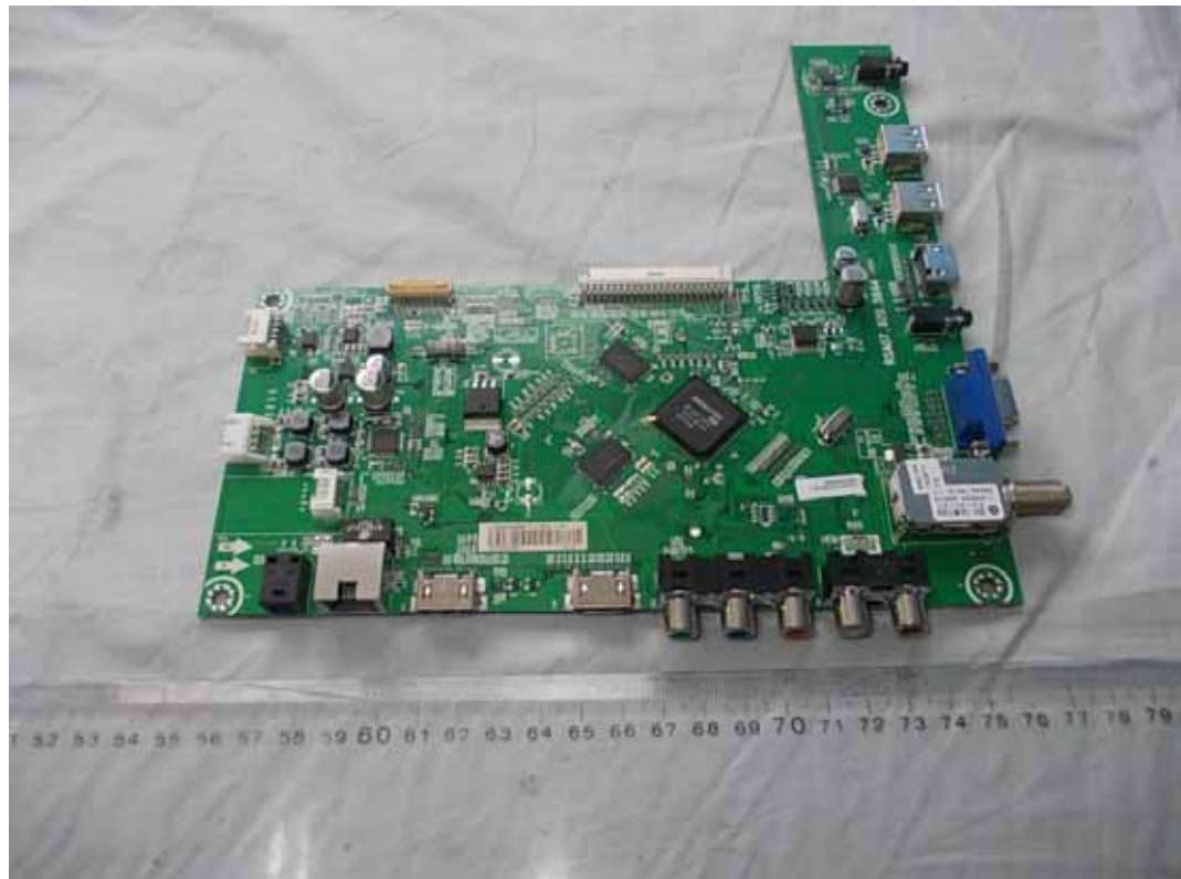
FIGURE 5 LED LCD TV (M/N: 50H5G) MAIN BOARD (COMPONENT SIDE)
