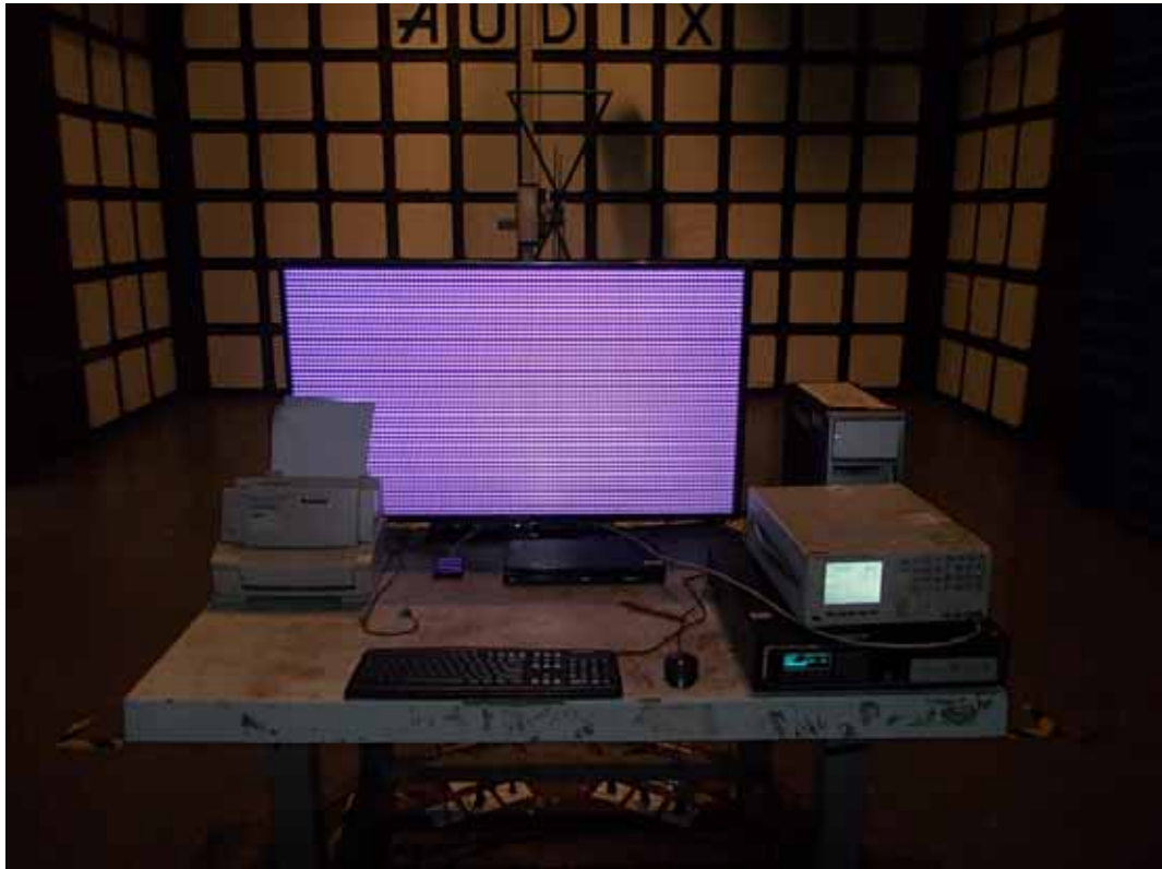
FRONT VIEW OF RADIATED EMISSION TEST
