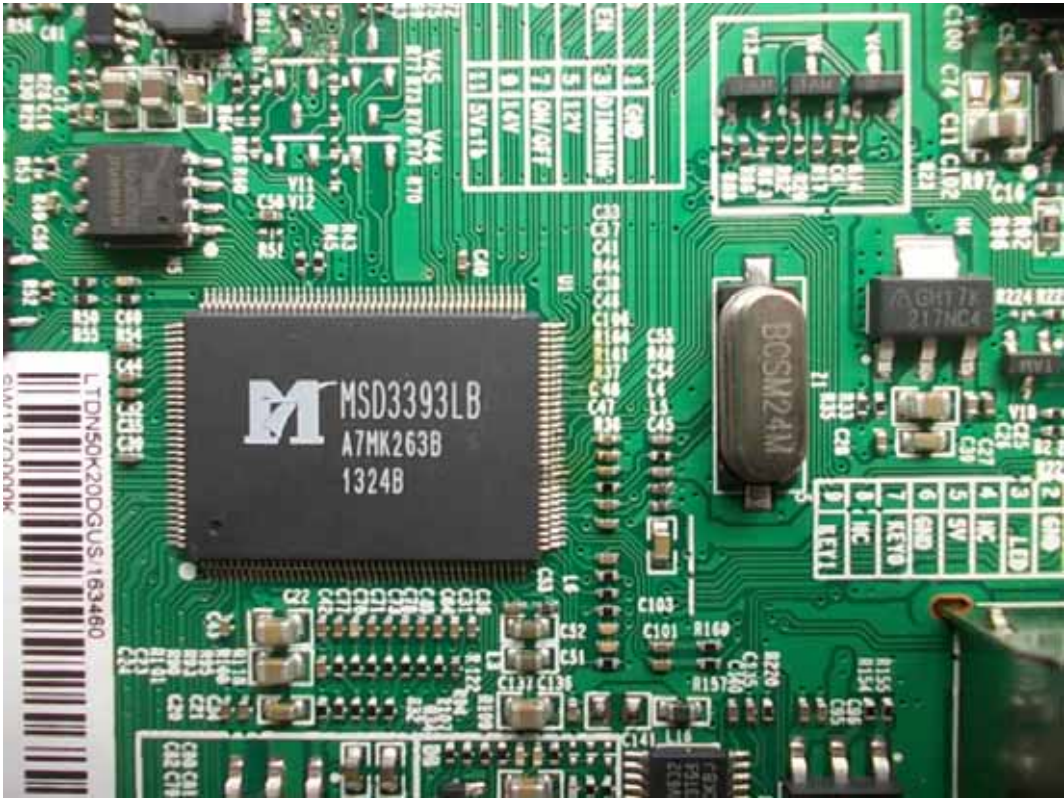
FIGURE 7 LED LCD TV (M/N: 50K20DG) CHIP & CRYSTAL ON MAIN BOARD
