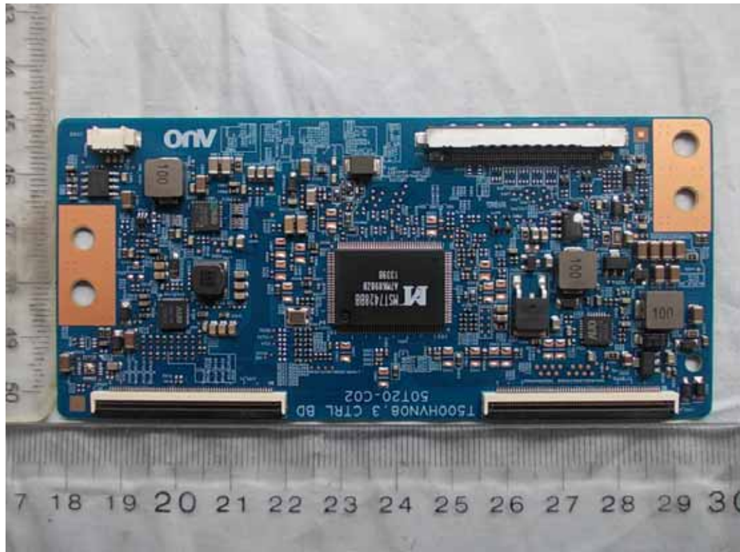
FIGURE 9 LED LCD TV (M/N: 50K20DG) LCD PANEL CONTROL BOARD (COMPONENT SIDE)
