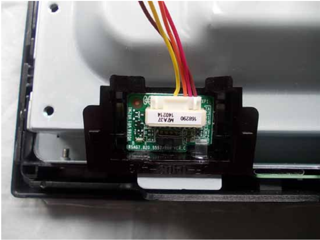
FIGURE 13 LED LCD TV (M/N: 50K20DG) IR BOARD (COMPONENT SIDE)
