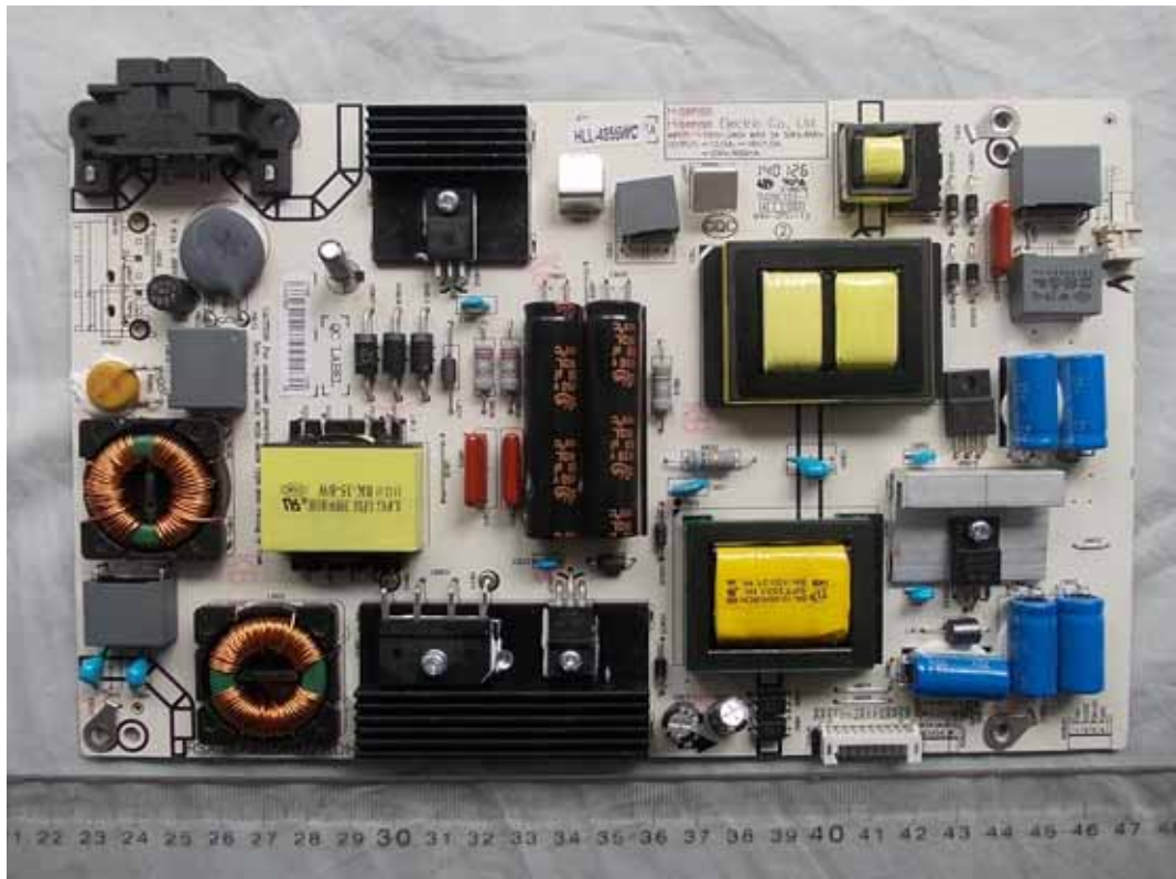
FIGURE 3 LED LCD TV (M/N: 50K20DG) POWER BOARD (COMPONENT SIDE)
