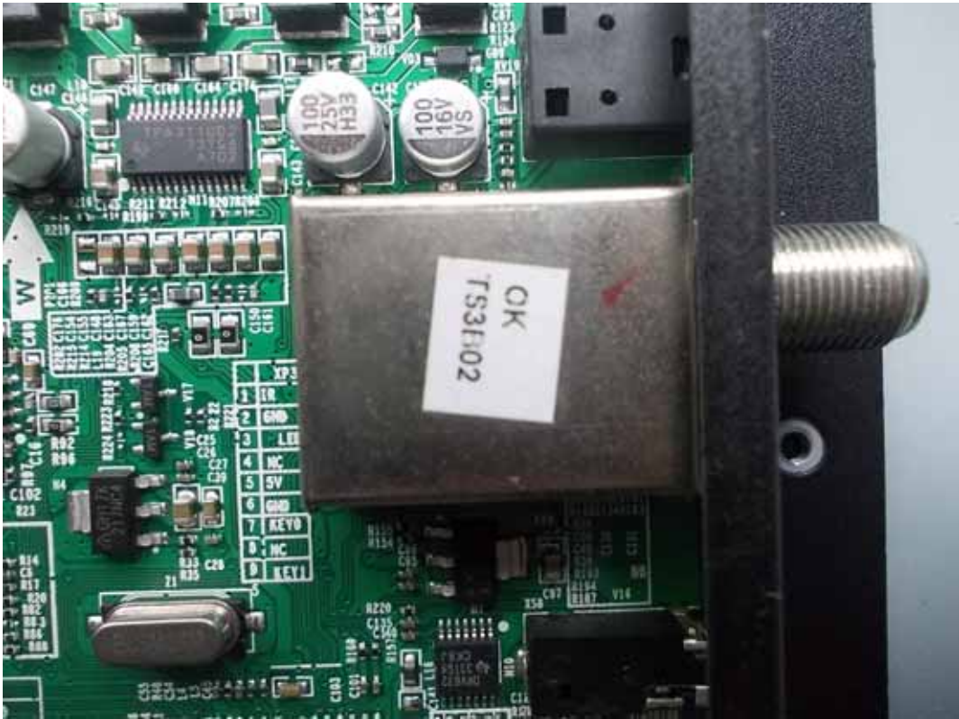
FIGURE 8 LED LCD TV (M/N: 50K20DG) TUNER ON MAIN BOARD
