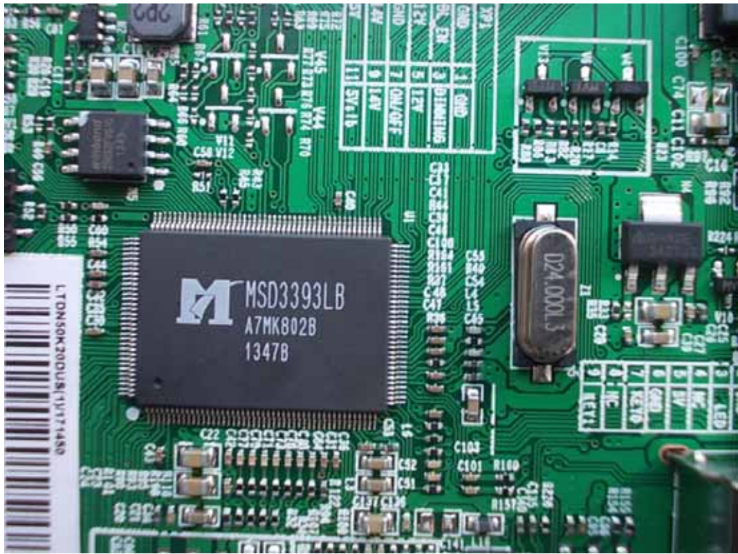
FIGURE 7 LED LCD TV (M/N: 50K20D) CHIP & CRYSTAL ON MAIN BOARD
