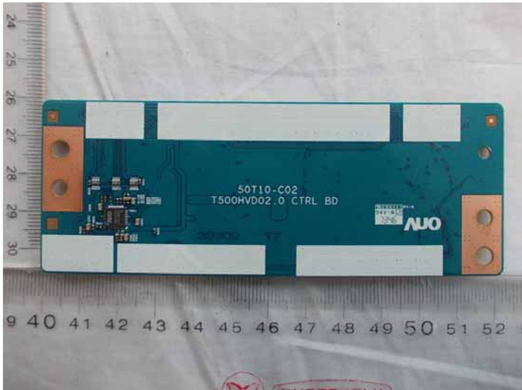
FIGURE 13 LED LCD TV (M/N: 50K20D) LED PANEL CONTROL BOARD (SOLDERED SIDE)
