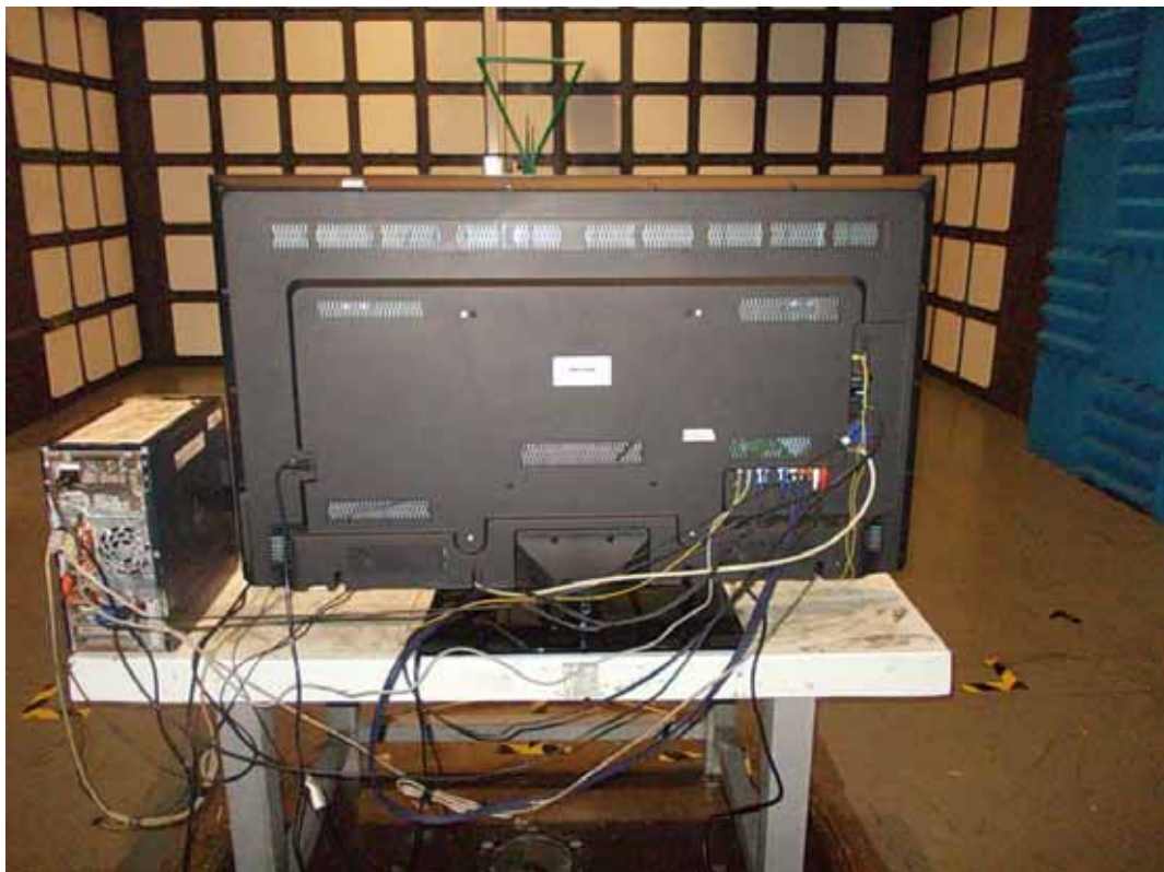
BACK VIEW OF RADIATED EMISSION TEST
