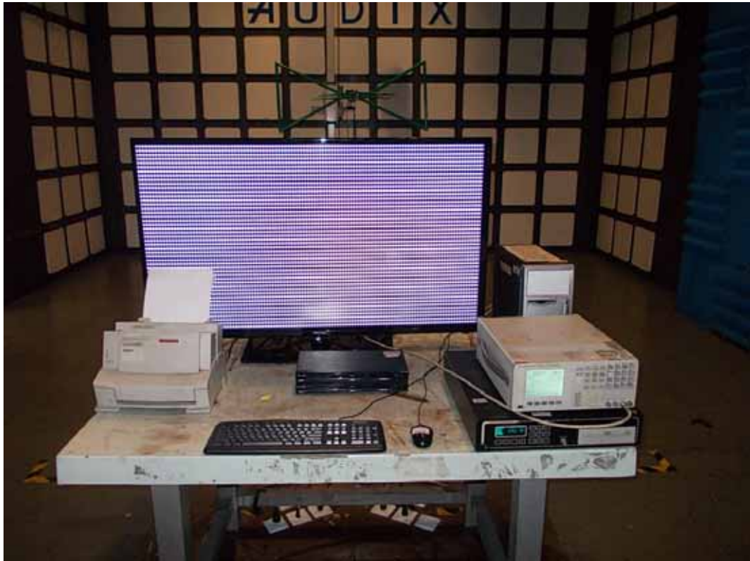
FRONT VIEW OF RADIATED EMISSION TEST
