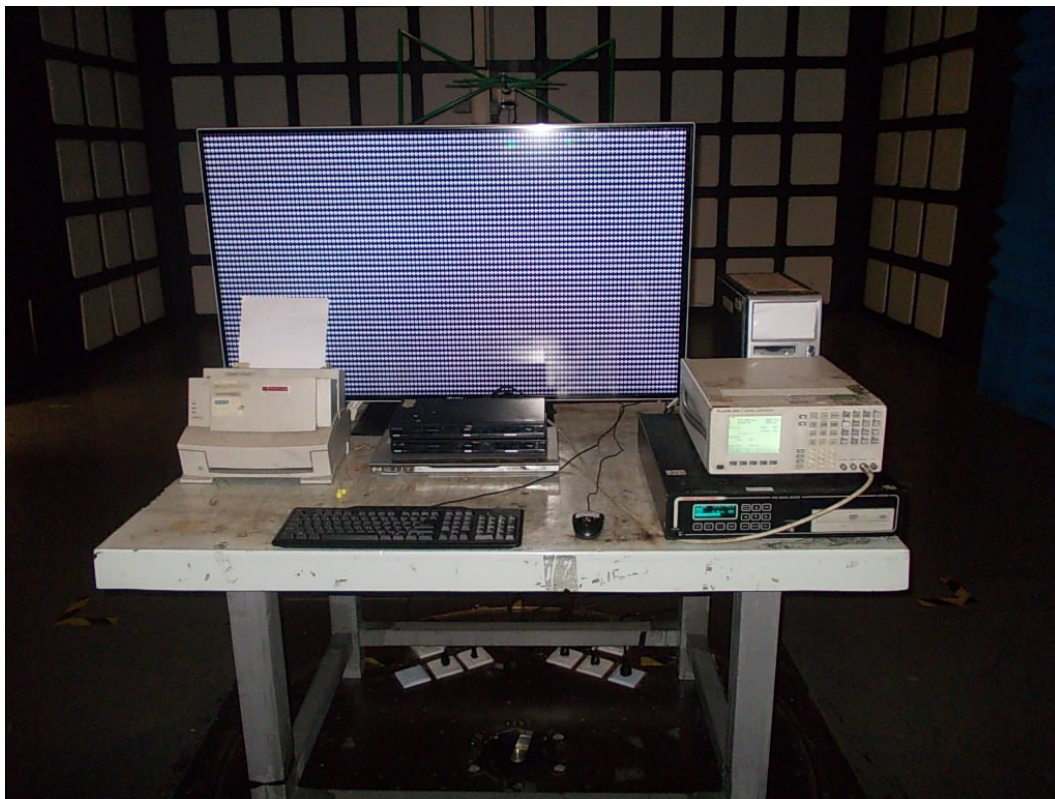
FRONT VIEW OF RADIATED EMISSION TEST
