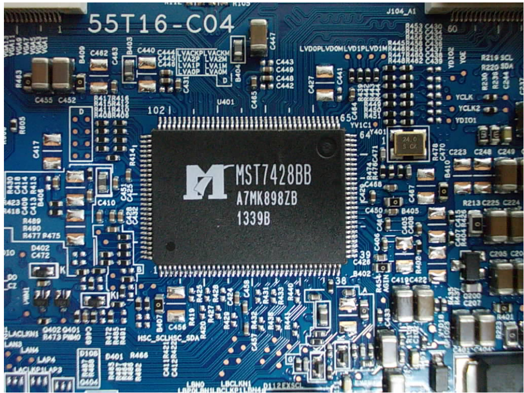
FIGURE 19 LED LCD TV (M/N: 55H6SG) CHIP & CRYSTAL ON LCD PANEL CONTROL BOARD
