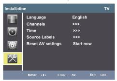
3 Press ▲ or ▼ to highlight an option, then press **ENTER** or ► to access the option, and press ⋖ or ► to adjust the option. You can select:
