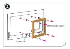
Place the provided spacers in the corresponding bracket holes. Attach purchased bracket (1.5mm to 2.5mm thickness) on the TV with 4 screws which are in the accessories bag. Follow instructions provided with the wall-mount bracket.
