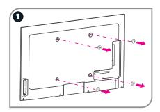
Make sure the TV is laid face-down on a clean, safe, and cushioned space, remove the holes on the TV back. (For 55") original screws in the bracket
