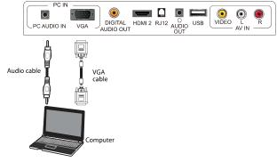
3 Connect one end of an audio cable with a stereo mini-plug (not included) to the PC AUDIO IN jack on the side of the TV, then connect the other end of the cable to the AUDIO OUT jack on the computer.
