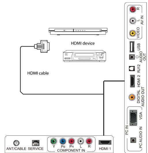
**Note:** To connect a DVI device, use a DVI to HDMI adapter cable to connect to the HDMI jack on the TV, then connect an audio cable to the PC AUDIO IN jack on the back of the TV.
