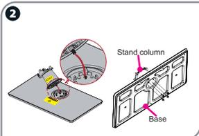
Insert the stand column into the base plate, aligning the ridge on the column with the groove in the base plate. Making sure the FRONT of stand column matched with the FRONT of base plate. Secure the stand column to the base plate with the 4 Screws (M4 × 12). (For 55": (M5×12))
