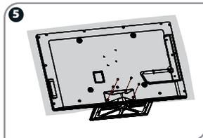
Secure the stand cover to the TV with the 4 screws (M5×12) provided.
