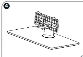
Secure the stand cover to the stand column horizontally with the 2 screws (ST4×14) provided.
