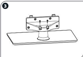
Secure the stand cover to the stand column vertically with the 2 screws (M4×12) provided. (For 55": (M5×12))
