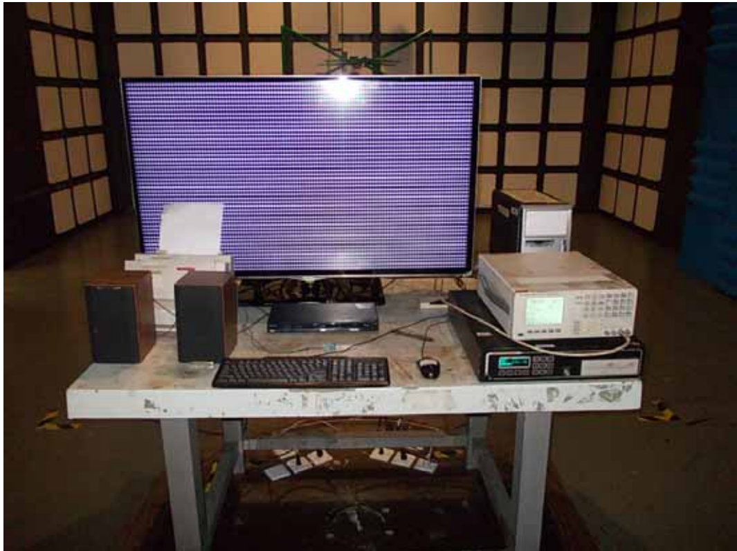
FRONT VIEW OF RADIATED EMISSION TEST
