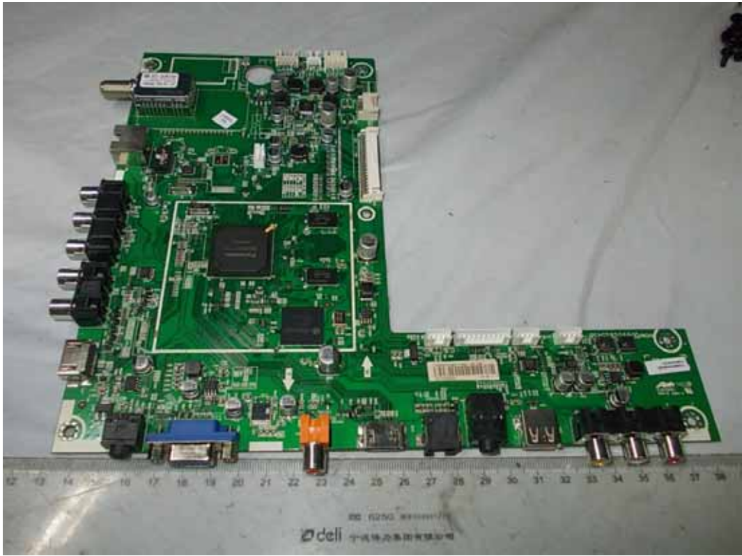
FIGURE 5 LED LCD TV (M/N: LTDN55K610GMH) MAIN BOARD (COMPONENT SIDE)
