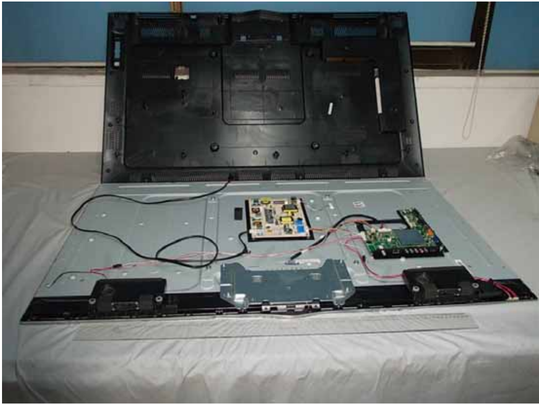
FIGURE 1 LED LCD TV (M/N: LTDN55K610GMH) COVER REMOVED
