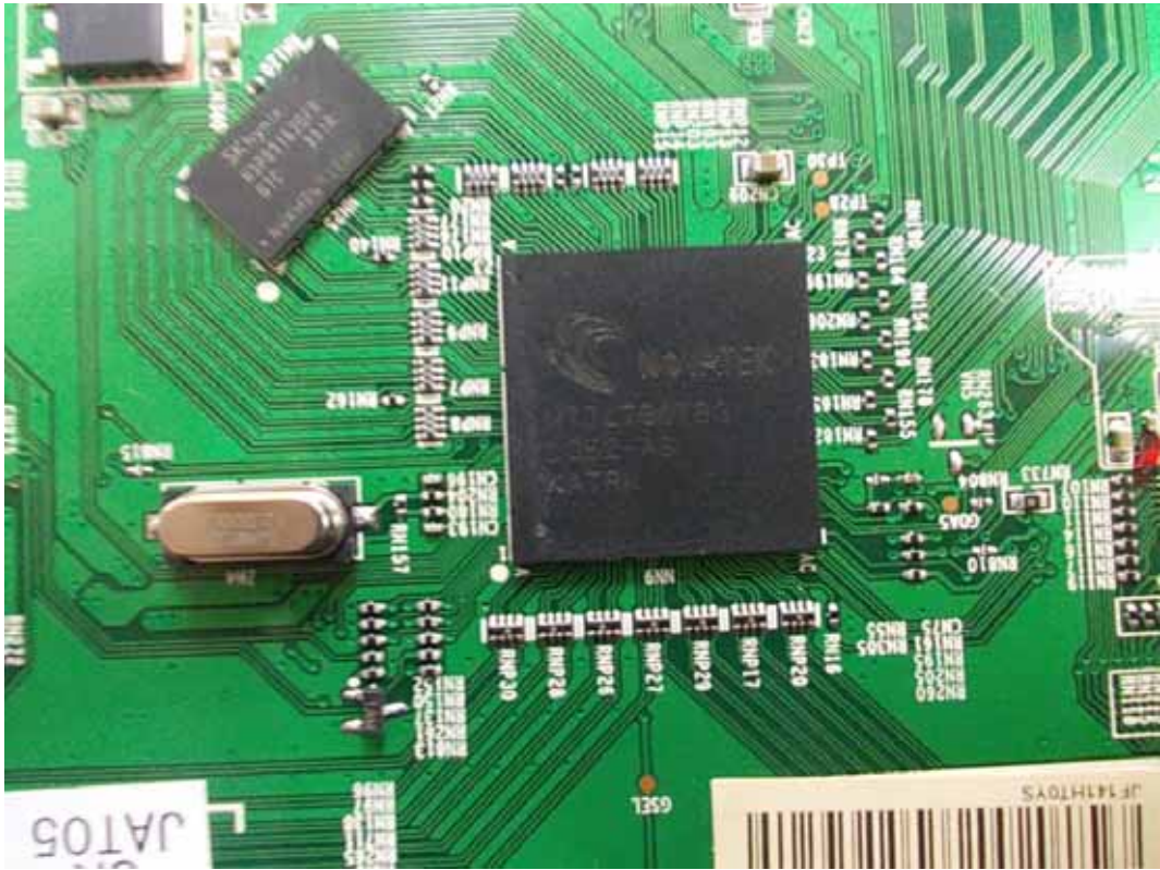
FIGURE 15 LED LCD TV (M/N: LTDN55K610GMH) CHIP & CRYSTAL ON LCD PANEL CONTROL BOARD
