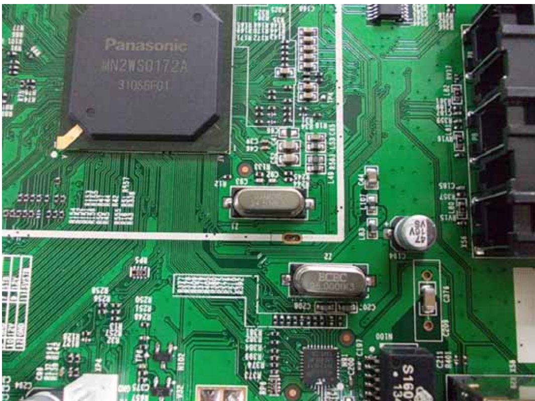
FIGURE 8 LED LCD TV (M/N: LTDN55K610GMH) CHIP & CRYSTAL #1 & #2 ON MAIN BOARD
