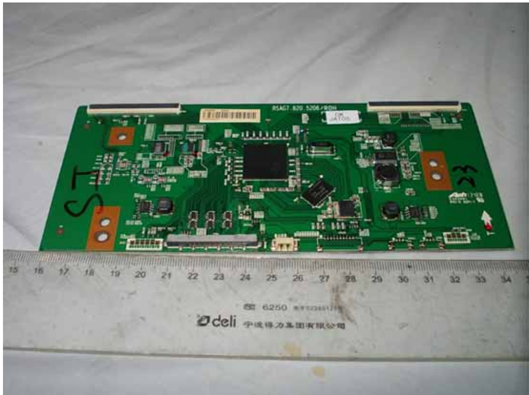
FIGURE 13 LED LCD TV (M/N: LTDN55K610GMH) LCD PANEL CONTROL BOARD (COMPONENT SIDE)
