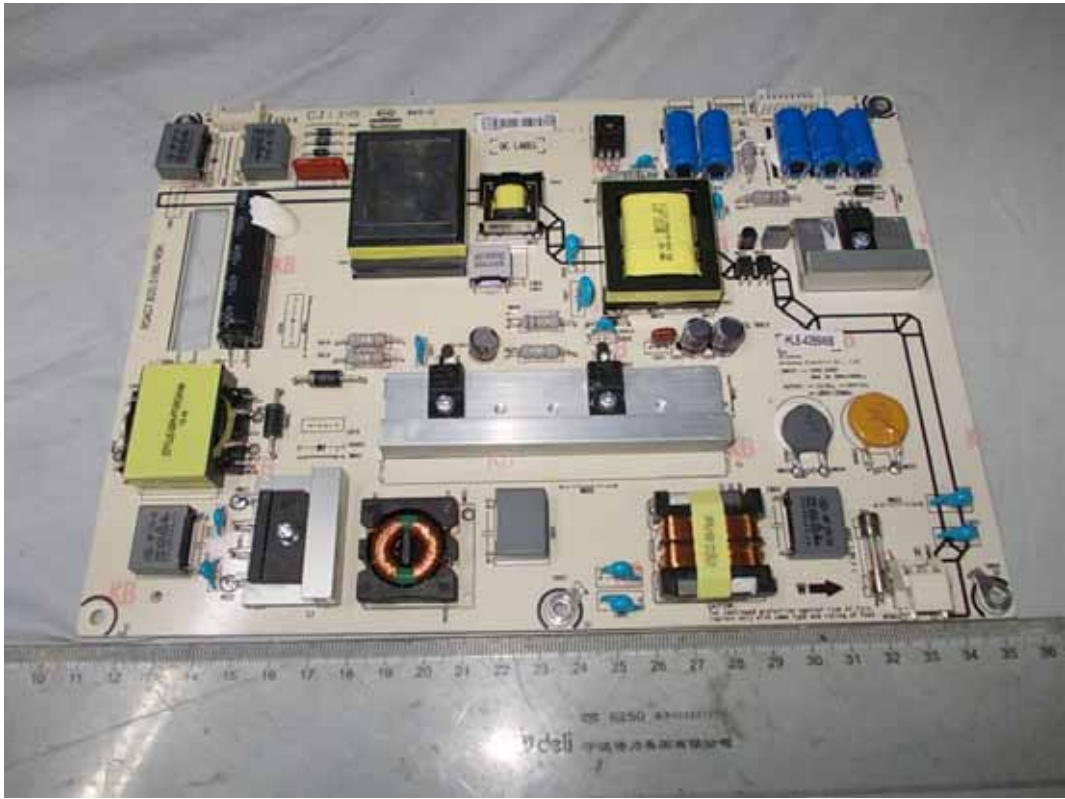
FIGURE 3 LED LCD TV (M/N: LTDN55K610GMH) POWER BOARD (COMPONENT SIDE)
