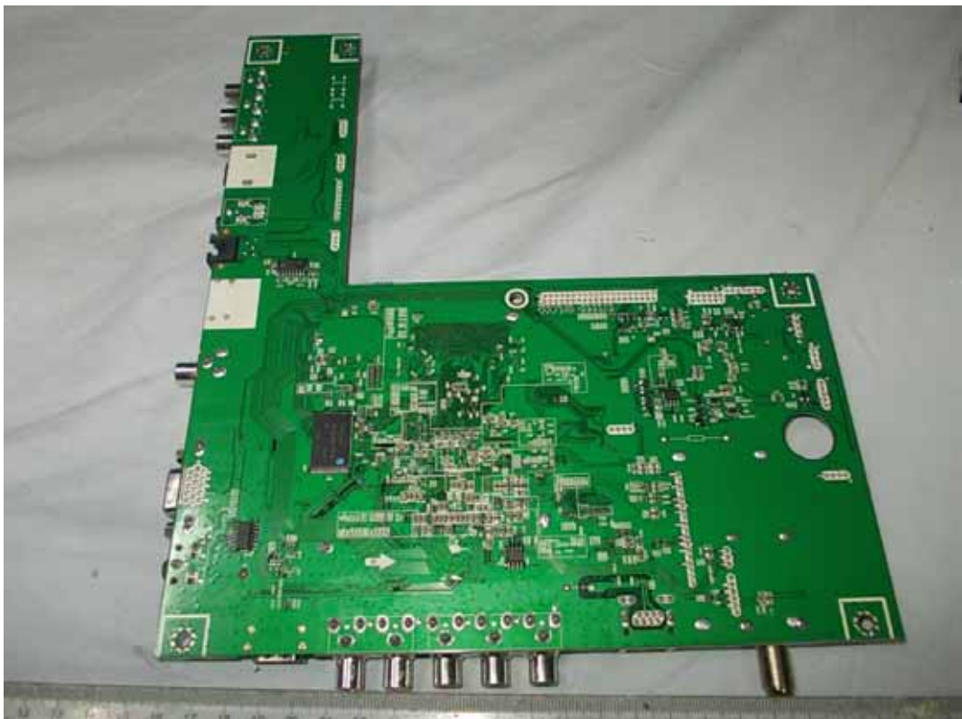
FIGURE 6 LED LCD TV (M/N: LTDN55K610GMH) MAIN BOARD (SOLDERED SIDE)
