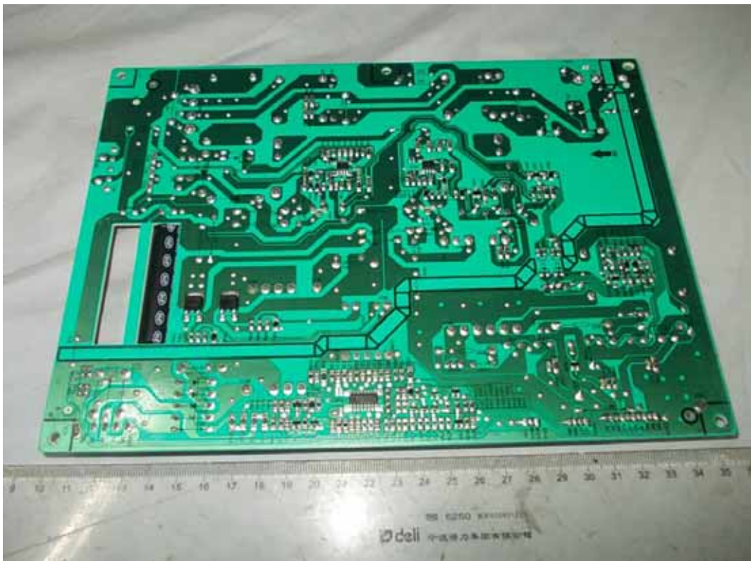
FIGURE 4 LED LCD TV (M/N: LTDN55K610GMH) POWER BOARD (SOLDERED SIDE)
