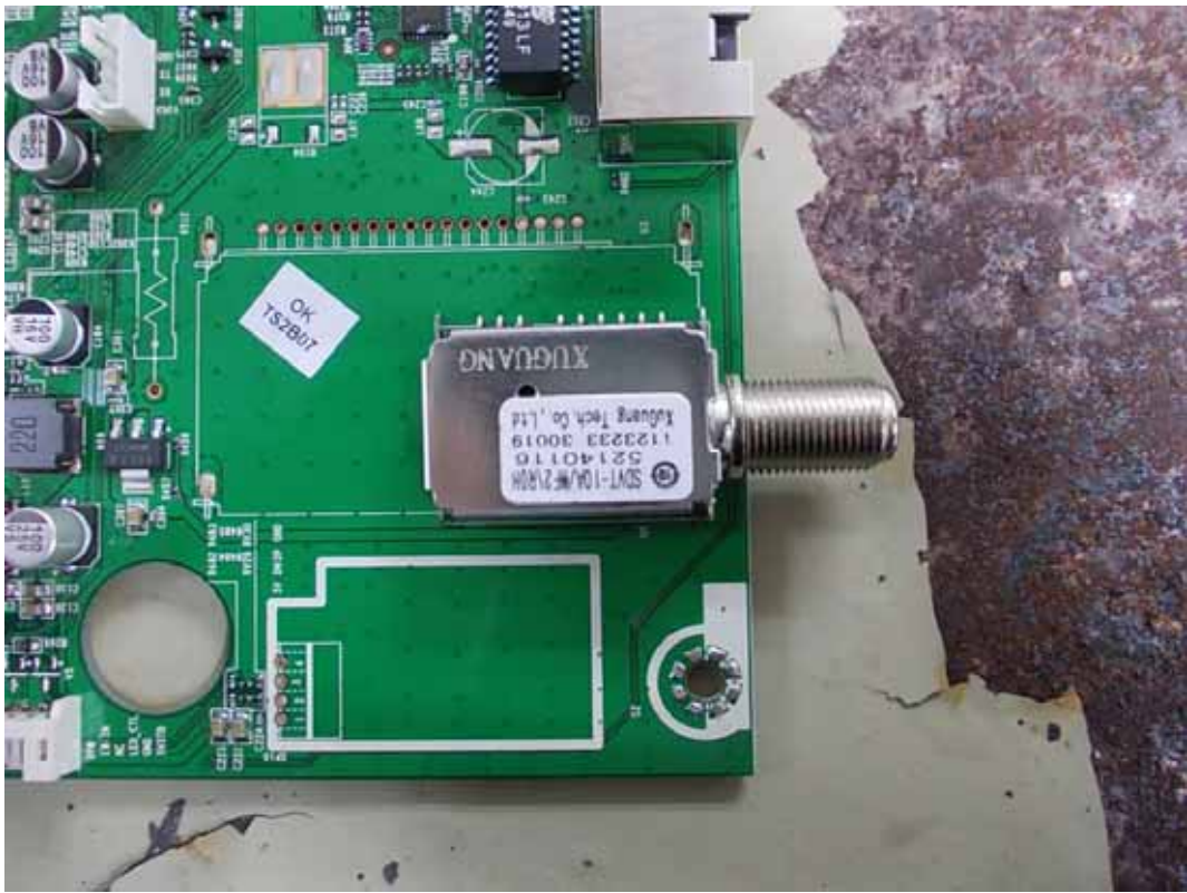
FIGURE 7 LED LCD TV (M/N: LTDN55K610GMH) TUNER ON MAIN BOARD
