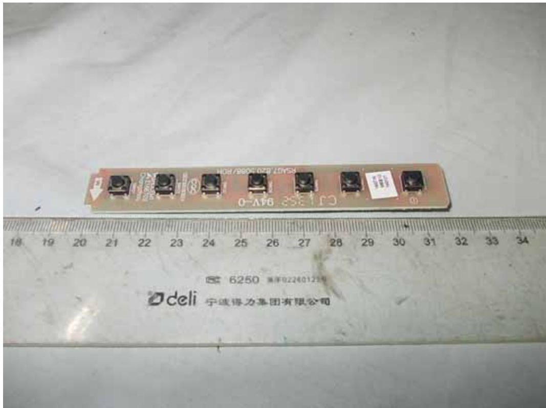
FIGURE 9 LED LCD TV (M/N: LTDN55K610GMH) KEY BOARD (COMPONENT SIDE)
