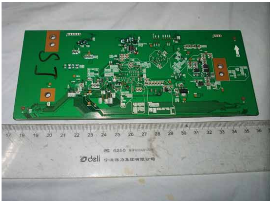
FIGURE 14 LED LCD TV (M/N: LTDN55K610GMH) LCD PANEL CONTROL BOARD (SOLDERED SIDE)
