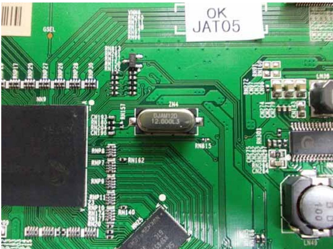
FIGURE 16 LED LCD TV (M/N: LTDN55K610GMH) CRYSTAL ON LCD PANEL CONTROL BOARD
