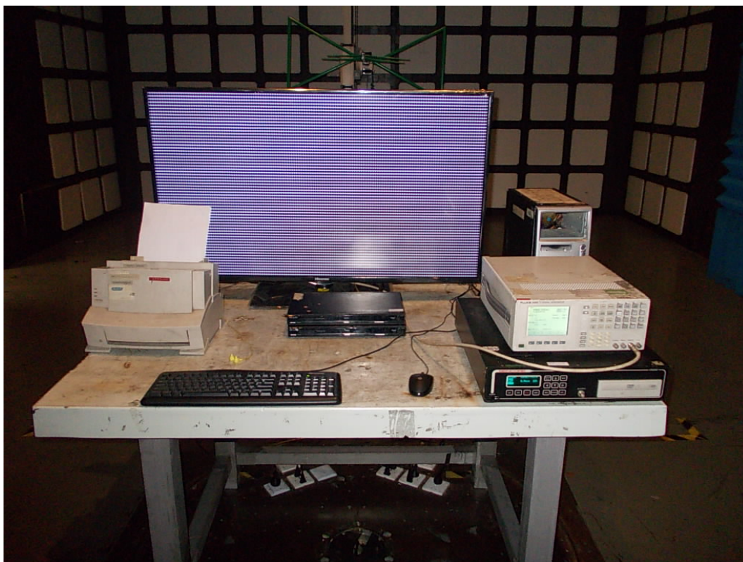
FRONT VIEW OF RADIATED EMISSION TEST
