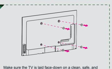
cushioned space, remove the original screws in the bracket Note: These 4 screws which got from back cover mount hole could not be used any more.
