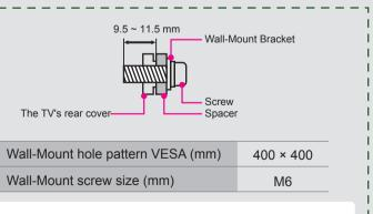
Follow instructions provided with the Wall-Mount bracket. If you are not sure of your ability to do complete the installation, contact a professional installer or service technician for assistance. The manufacturer is not responsible for any damages or injuries that occur due to mishandling or incorrect assembly. The selected screws are 9.5 ~ 11.5 mm in length when
