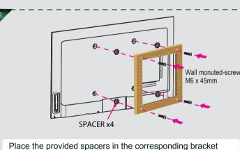
holes. Attach purchased bracket (1.5mm to 2.5mm thickness) on the TV with 4 screws which are in the accessories bag. Follow instructions provided with the wall-mount bracket.
