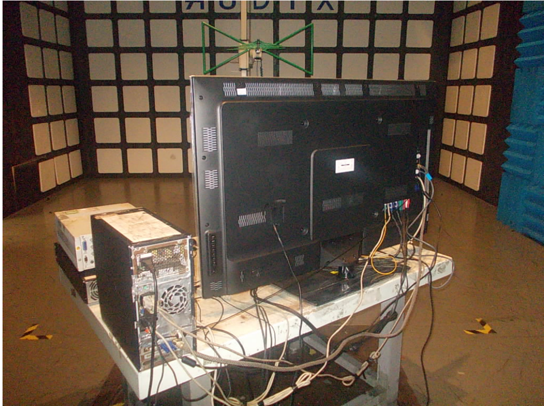
SETUP WITH MAXIMUM DETECTED EMISSION AT HORIZONTAL POLARIZATION (TEST MODE: HDMI 1024*768@60Hz)
