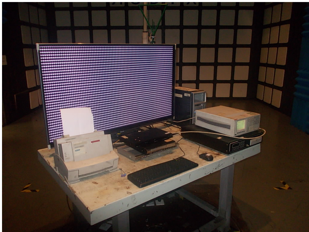
SETUP WITH MAXIMUM DETECTED EMISSION AT VERTICAL POLARIZATION (TEST MODE: HDMI 1024*768@60Hz)
