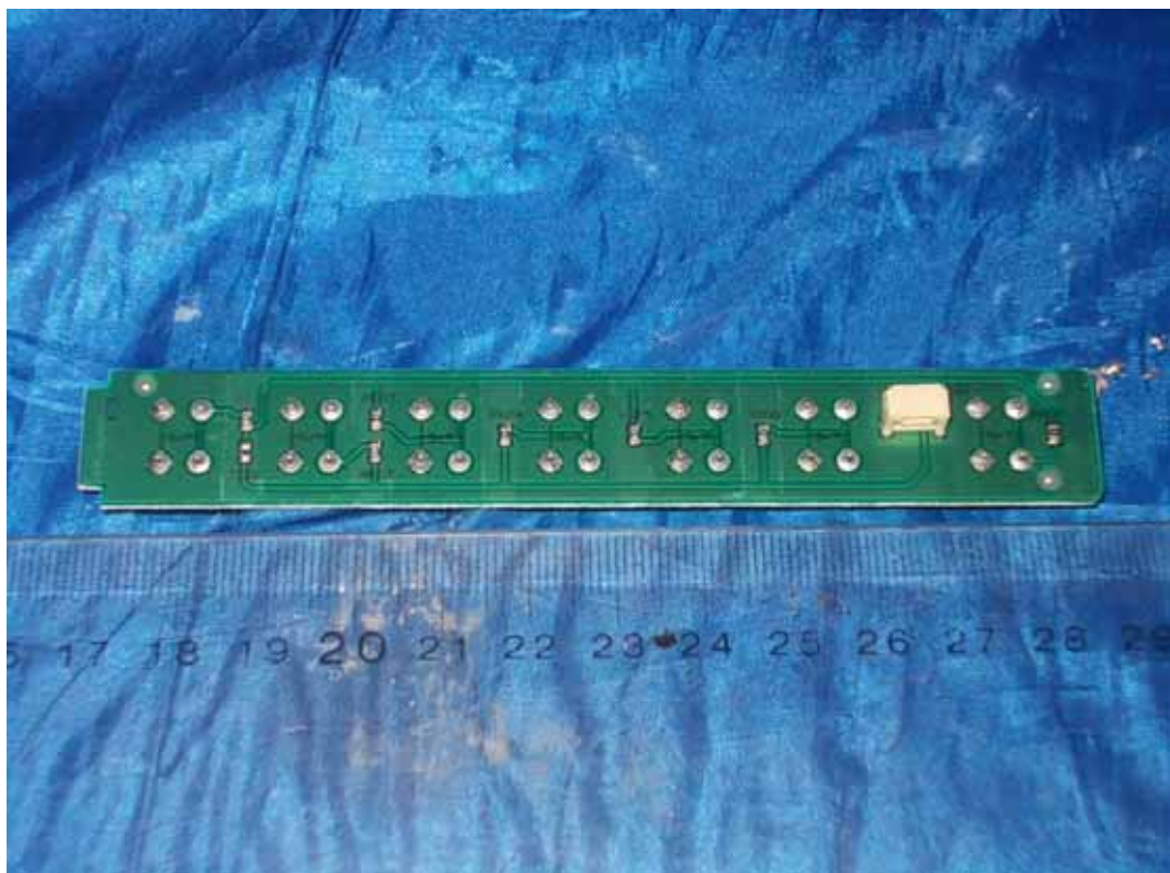
FIGURE 12 LED LCD TV (M/N: 55K610GWN) KEY BOARD (SOLDERED SIDE)
