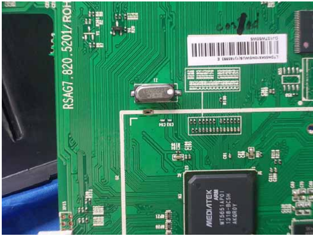
FIGURE 9 LED LCD TV (M/N: 55K610GWN) CHIP #1 & CRYSTAL #1 ON MAIN BOARD
