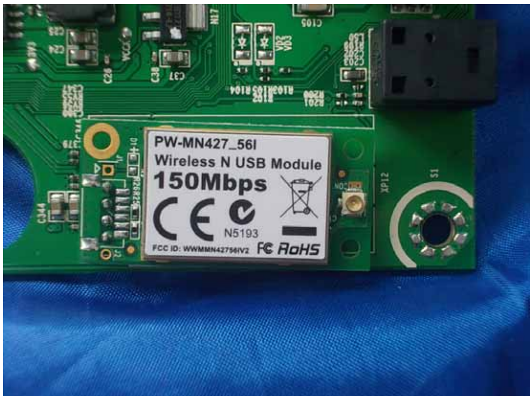
FIGURE 8 LED LCD TV (M/N: 55K610GWN) WIRELESS N USB MODULE
