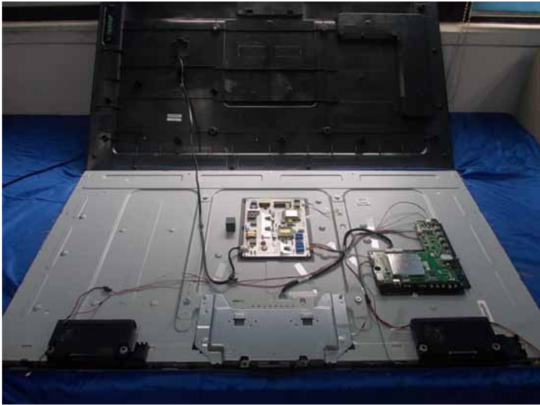
FIGURE 1 LED LCD TV (M/N: 55K610GWN) COVER REMOVED
