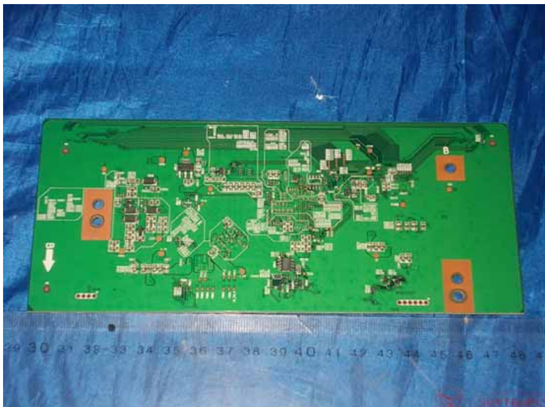
FIGURE 16 LED LCD TV (M/N: 55K610GWN) LCD PANEL CONTROL BOARD (SOLDERED SIDE)
