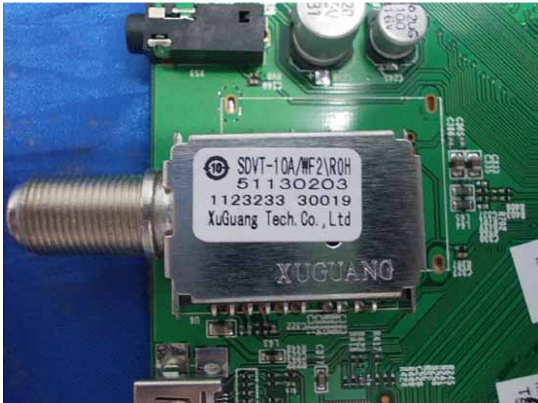
FIGURE 7 LED LCD TV (M/N: 55K610GWN) TUNER ON MAIN BOARD
