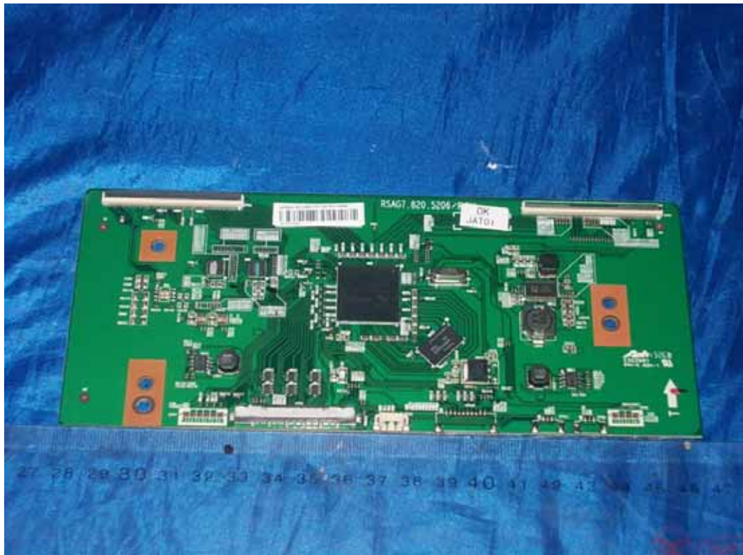
FIGURE 15 LED LCD TV (M/N: 55K610GWN) LCD PANEL CONTROL BOARD (COMPONENT SIDE)
