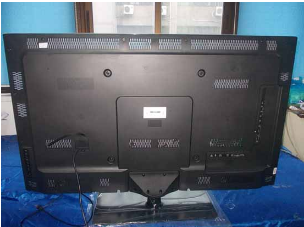
FIGURE 2 LED LCD TV (M/N: 55K610GWN) GENERAL APPEARANCE (BACK VIEW)
