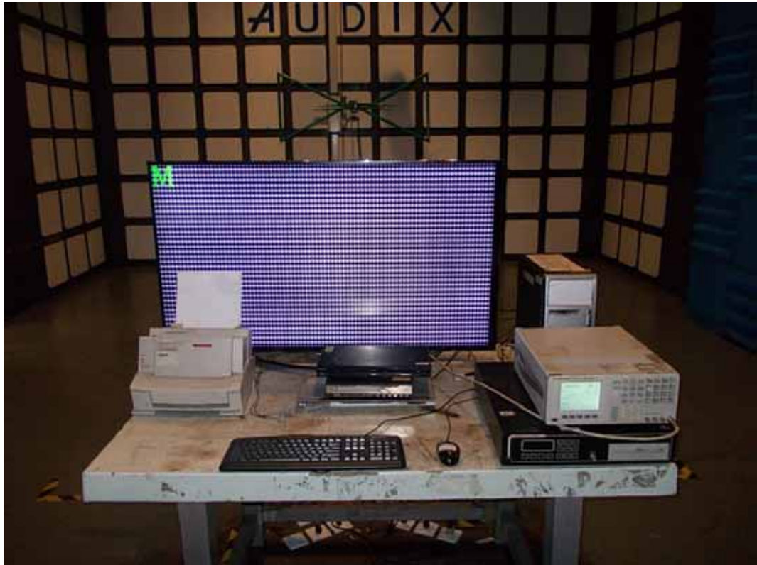
FRONT VIEW OF RADIATED EMISSION TEST
