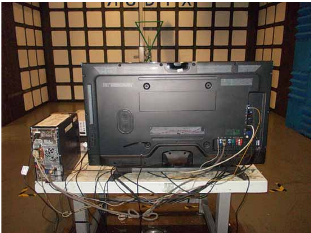
BACK VIEW OF RADIATED EMISSION TEST
