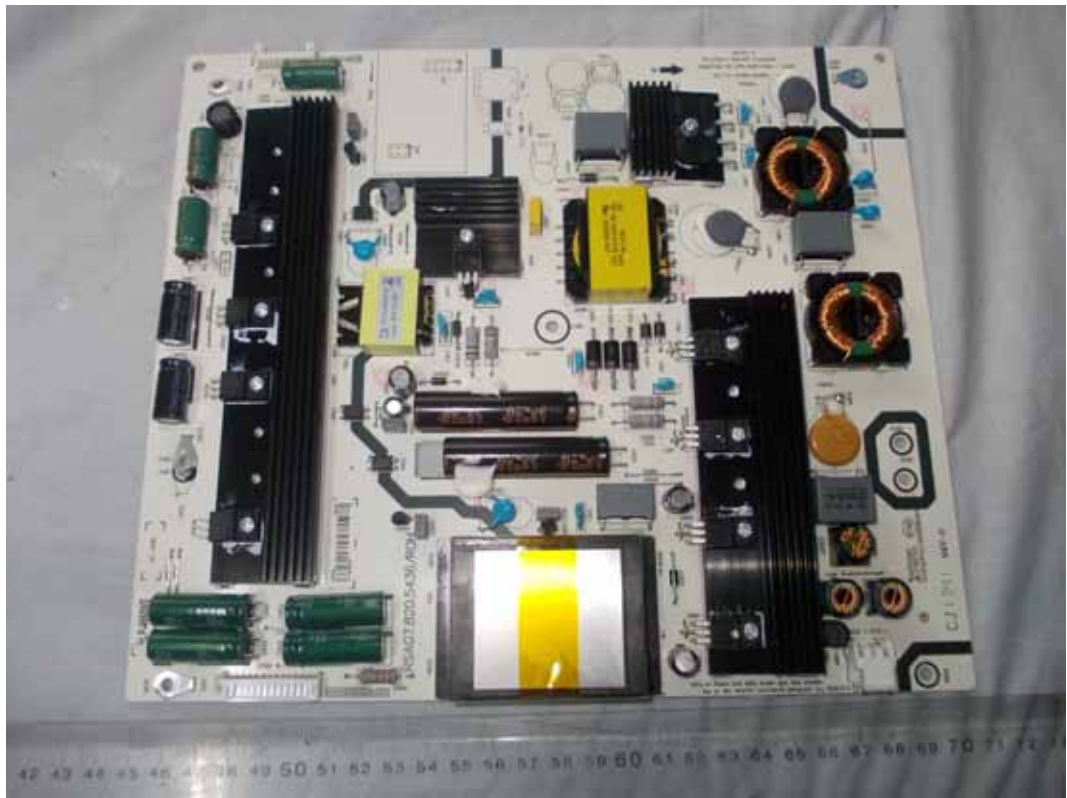
FIGURE 3 LED LCD TV (M/N: LTDN55XT880WUS) POWER BOARD (COMPONENT SIDE)
