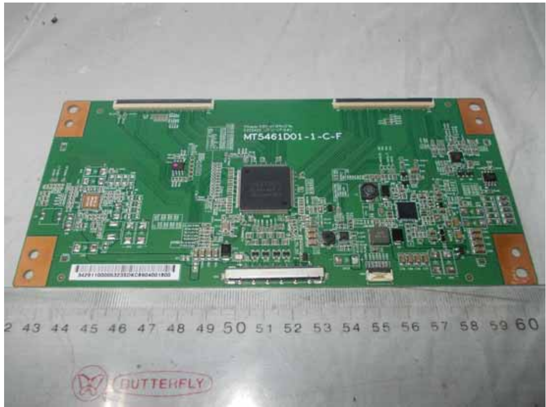
FIGURE 13 LED LCD TV (M/N: LTDN55XT880WUS) LCD PANEL CONTROL BOARD (COMPONENT SIDE)
