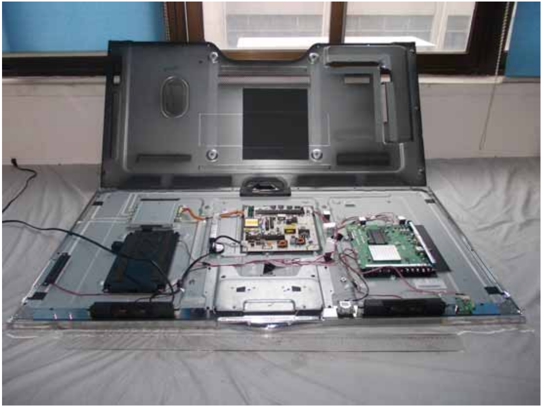
FIGURE 1 LED LCD TV (M/N: LTDN55XT880WUS) COVER REMOVED
