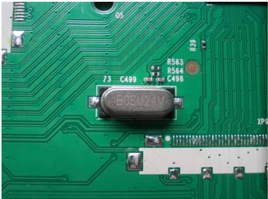
FIGURE 12 LED LCD TV (M/N: LTDN55XT880WUS) CRYSTAL #3 ON MAIN BOARD
