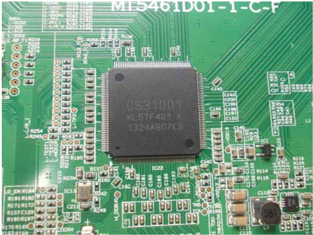
FIGURE 15 LED LCD TV (M/N: LTDN55XT880WUS) CHIP ON LCD PANEL CONTROL BOARD
