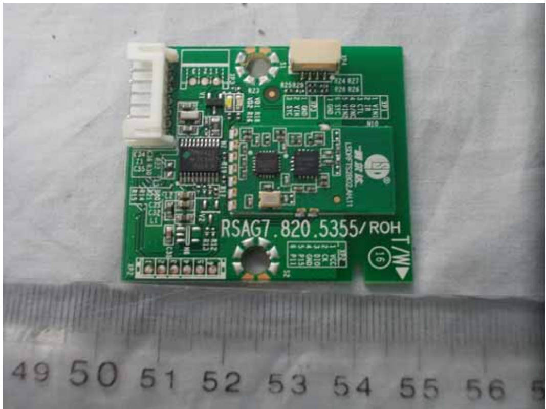
FIGURE 20 LED LCD TV (M/N: LTDN55XT880WUS) BOARD #1 (COMPONENT SIDE)
