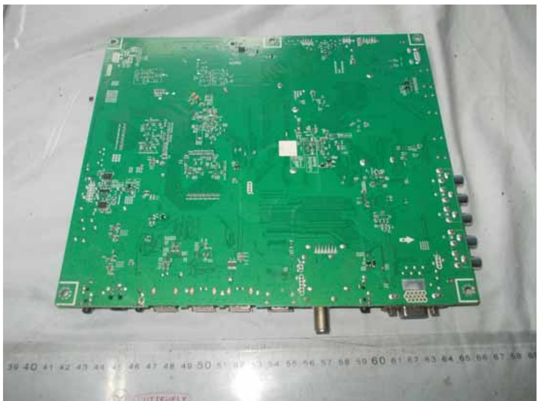
FIGURE 6 LED LCD TV (M/N: LTDN55XT880WUS) MAIN BOARD (SOLDERED SIDE)
