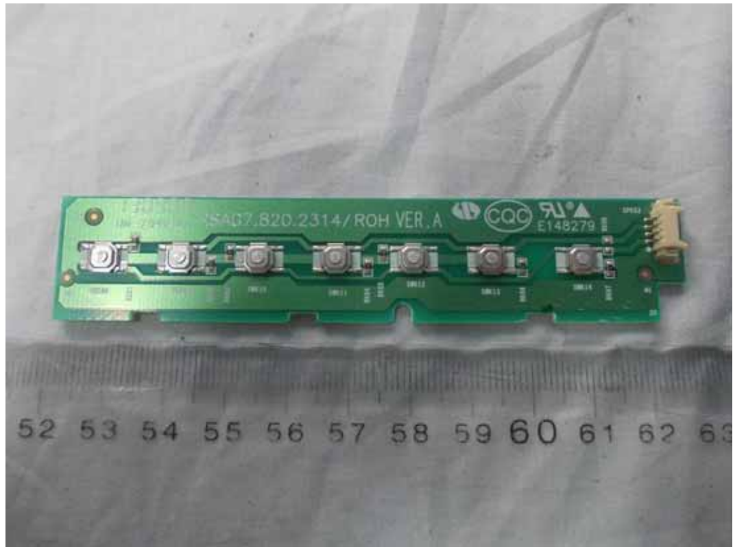
FIGURE 16 LED LCD TV (M/N: LTDN55XT880WUS) KEY BOARD (COMPONENT SIDE)
