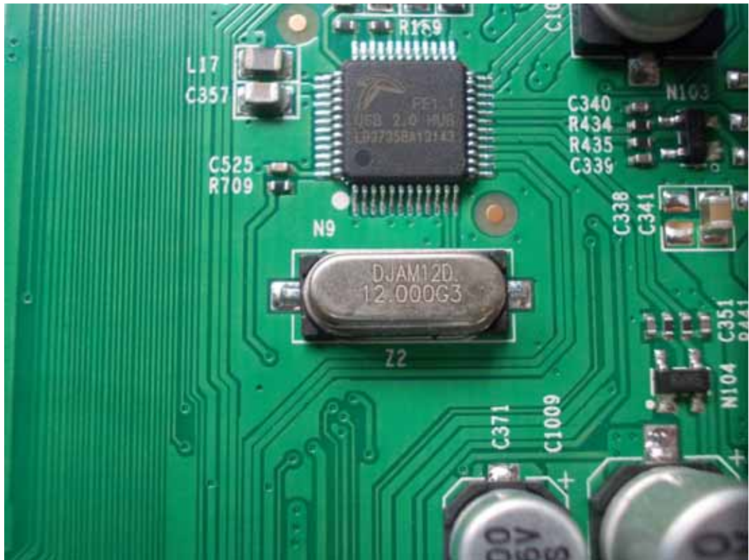
FIGURE 11 LED LCD TV (M/N: LTDN55XT880WUS) CHIP #3 & CRYSTAL #2 ON MAIN BOARD
