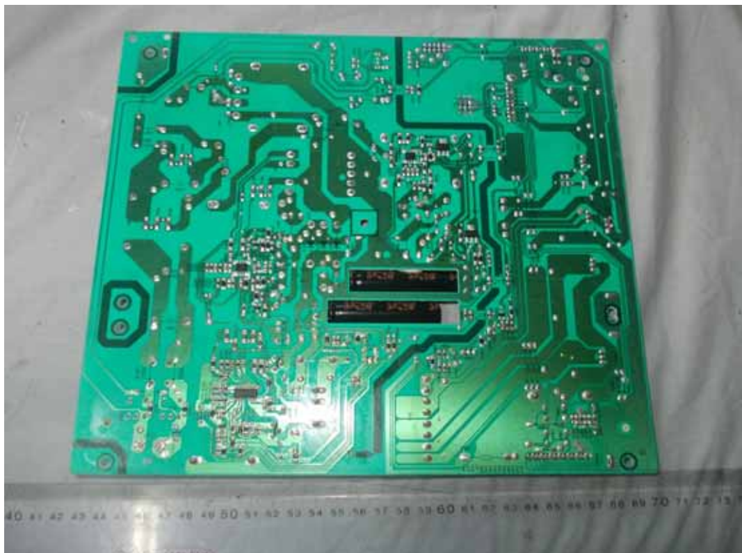
FIGURE 4 LED LCD TV (M/N: LTDN55XT880WUS) POWER BOARD (SOLDERED SIDE)
