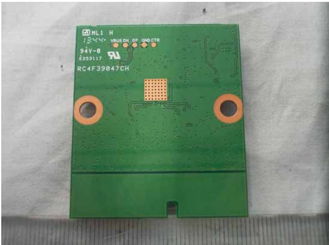
FIGURE 19 LED LCD TV (M/N: LTDN55XT880WUS) RF BOARD (SOLDERED SIDE)
