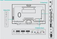
Check the jacks for position and type before making any connections. Loose connections can result in image or color problems. Make sure that all connections are tight and secure.
