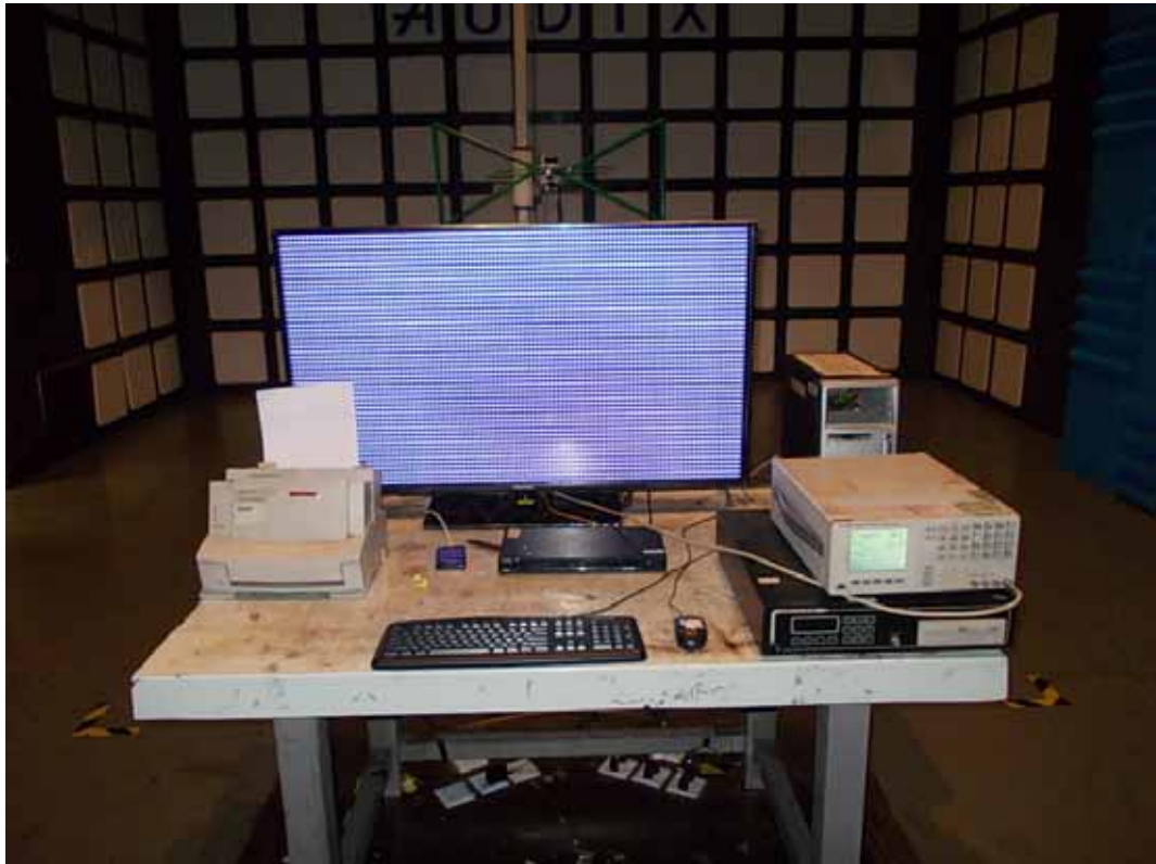
FRONT VIEW OF RADIATED EMISSION TEST
