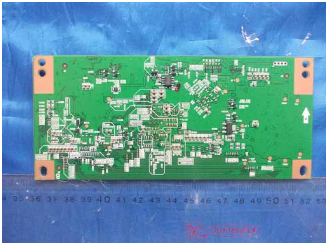
FIGURE 10 LED LCD TV (M/N: 50K20DG) LCD PANEL CONTROL BOARD (SOLDERED SIDE)
