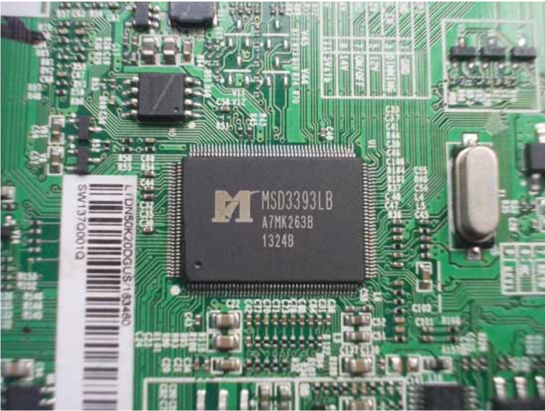
FIGURE 7 LED LCD TV (M/N: 50K20DG) CHIP ON MAIN BOARD
