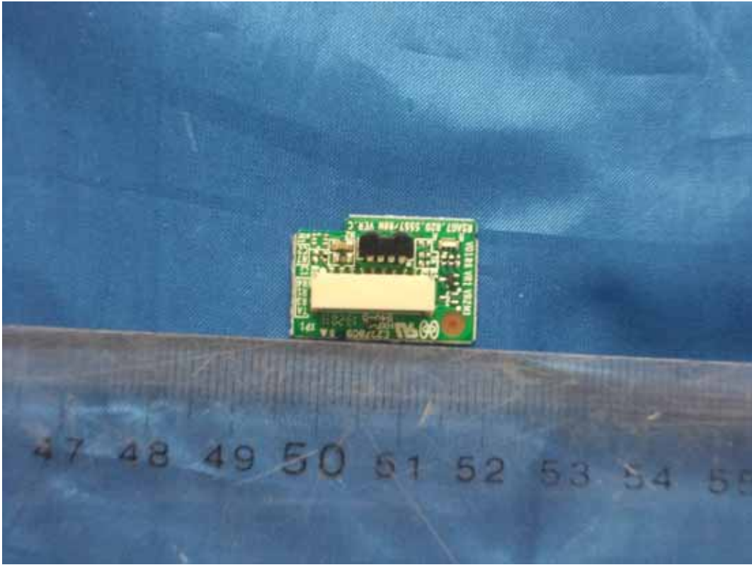
FIGURE 14 LED LCD TV (M/N: 50K20DG) IR BOARD (COMPONENT SIDE)
