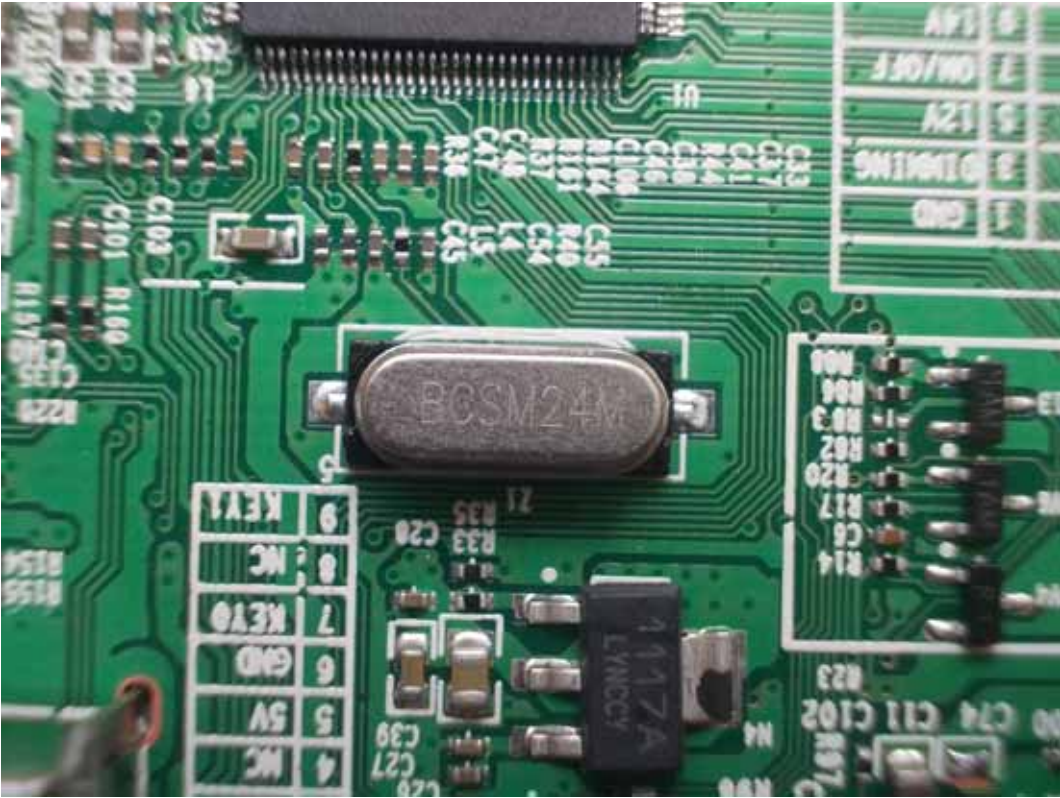
FIGURE 8 LED LCD TV (M/N: 50K20DG) CRYSTAL ON MAIN BOARD
