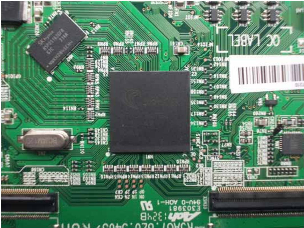
FIGURE 11 LED LCD TV (M/N: 50K20DG) CHIP & CRYSTAL ON LCD PANEL CONTROL BOARD
