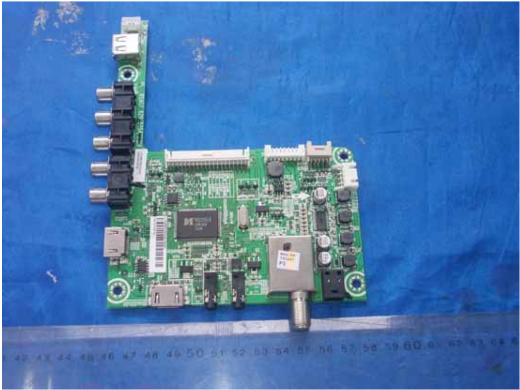
FIGURE 5 LED LCD TV (M/N: 50K20DG) MAIN BOARD (COMPONENT SIDE)
