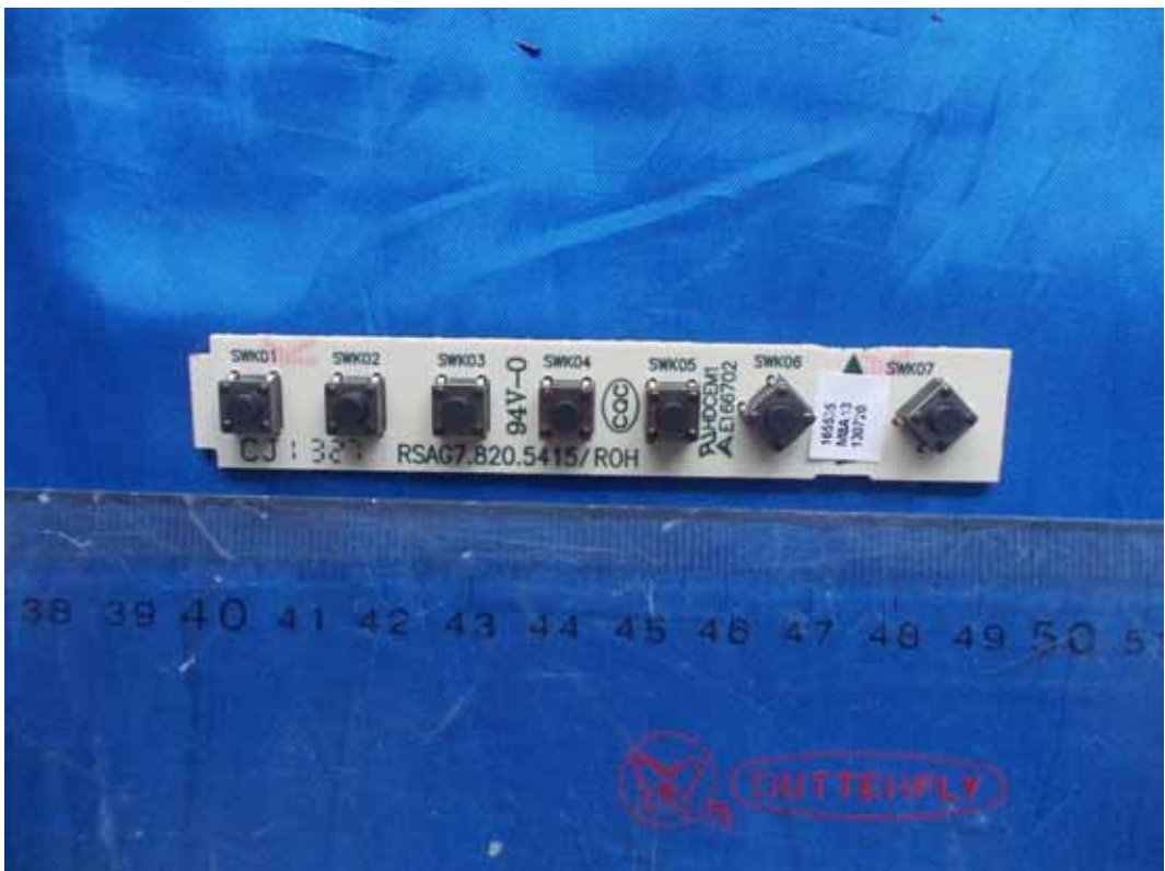
FIGURE 12 LED LCD TV (M/N: 50K20DG) KEY BOARD (COMPONENT SIDE)
