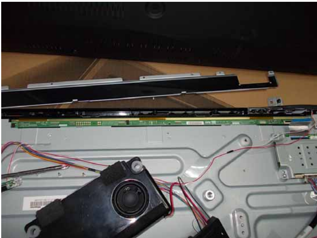
FIGURE 24 LED LCD TV (M/N: 50K366GW) LCD PANEL CONTROL BOARD #2
