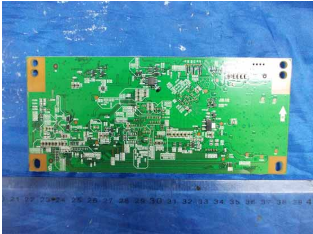
FIGURE 21 LED LCD TV (M/N: 50K366GW) LCD PANEL CONTROL BOARD #1 (SOLDERED SIDE)
