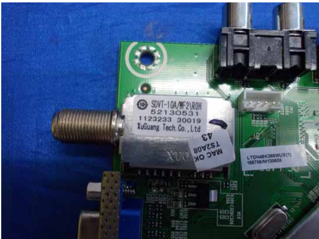
FIGURE 12 LED LCD TV (M/N: 50K366GW) TUNER ON MAIN BOARD
