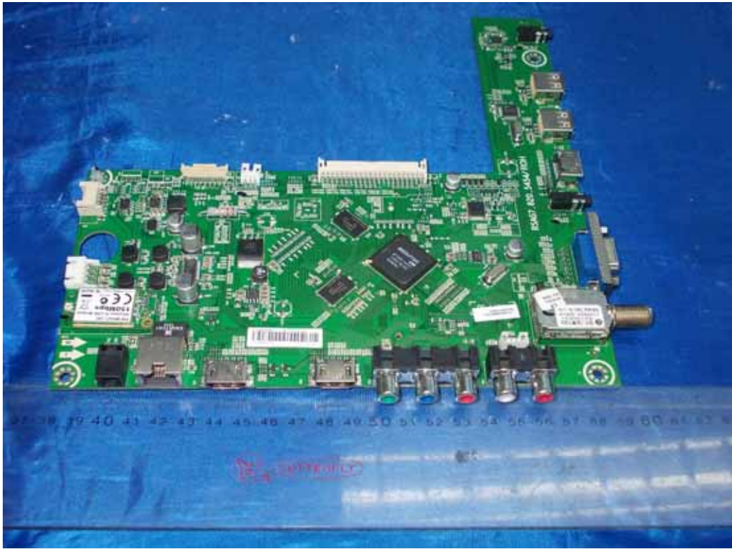
FIGURE 9 LED LCD TV (M/N: 50K366GW) MAIN BOARD (COMPONENT SIDE)
