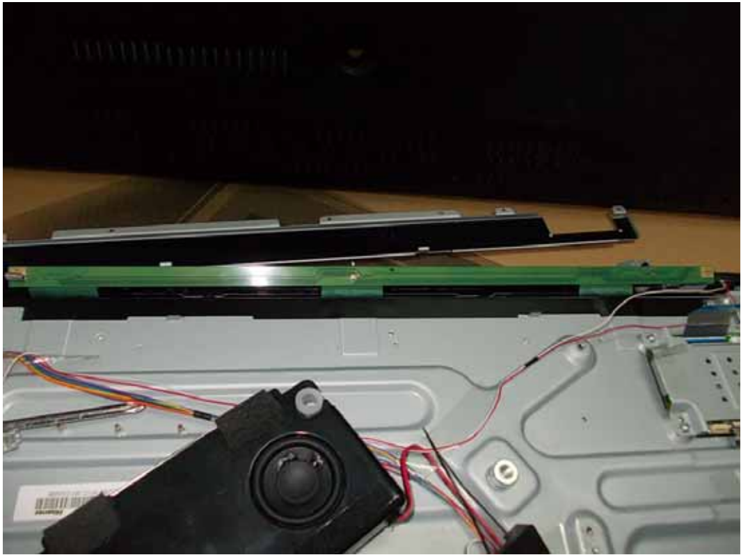
FIGURE 25 LED LCD TV (M/N: 50K366GW) LCD PANEL CONTROL BOARD #2
