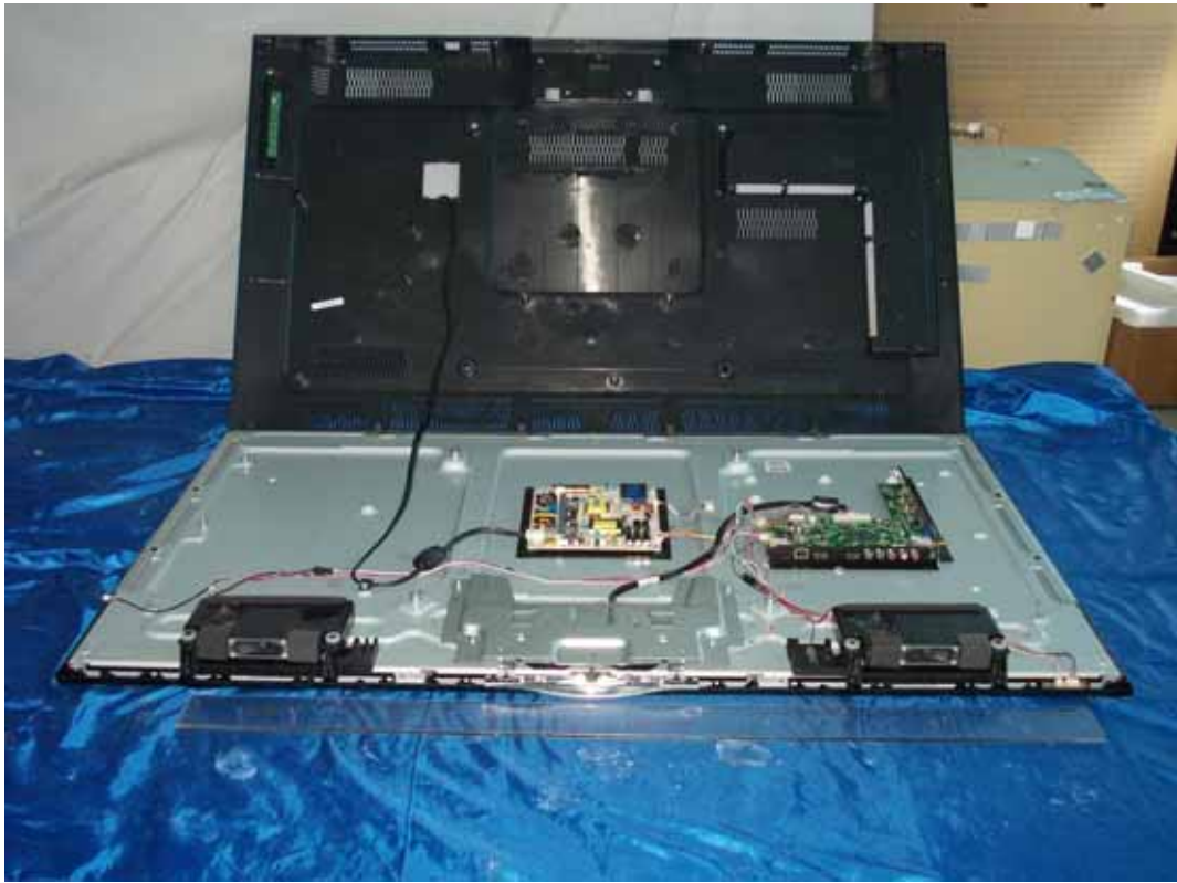
FIGURE 5 LED LCD TV (M/N: 50K366GW) COVER REMOVED
