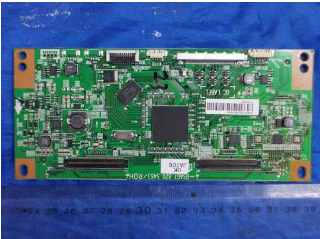
FIGURE 20 LED LCD TV (M/N: 50K366GW) LCD PANEL CONTROL BOARD #1 (COMPONENT SIDE)
