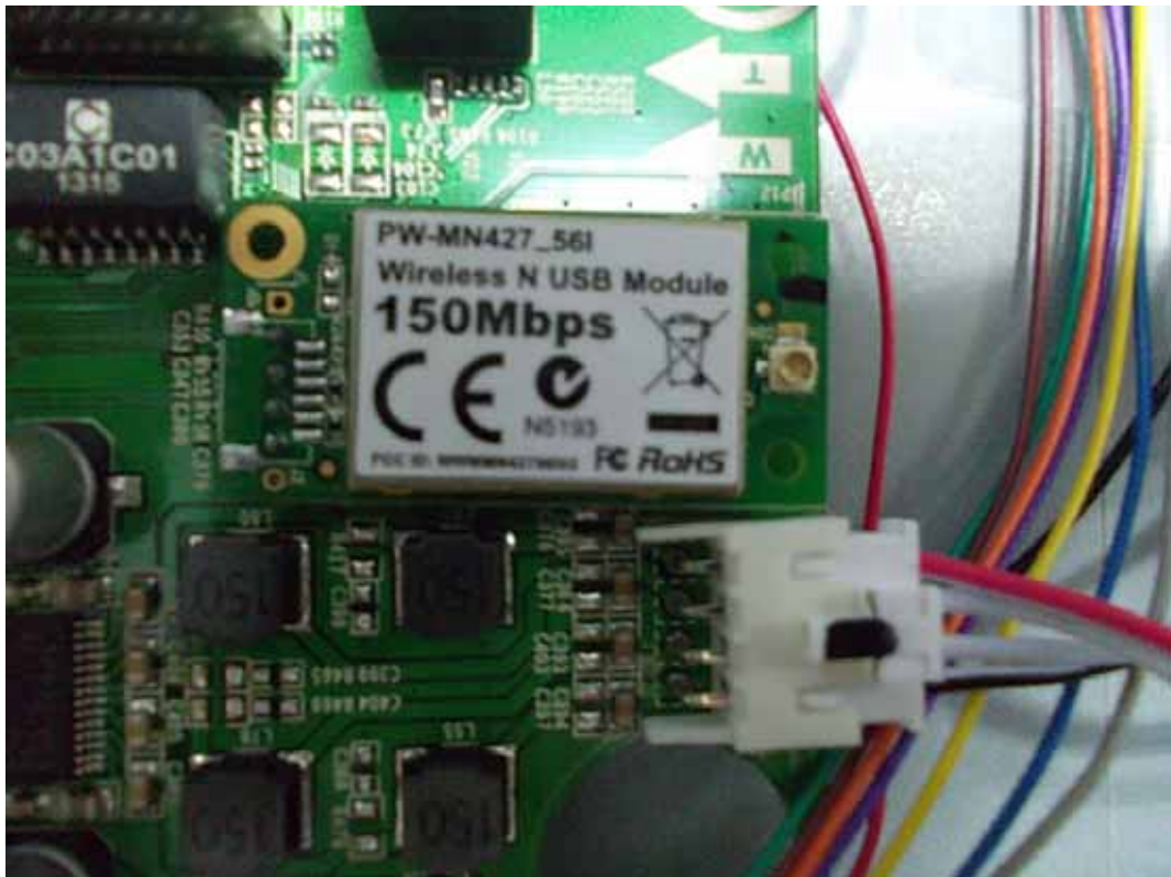
FIGURE 11 LED LCD TV (M/N: 50K366GW) WIFI MODULE ON MAIN BOARD
