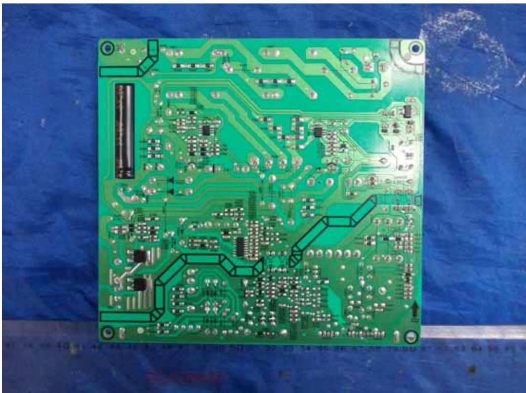
FIGURE 8 LED LCD TV (M/N: 50K366GW) POWER BOARD (SOLDERED SIDE)
