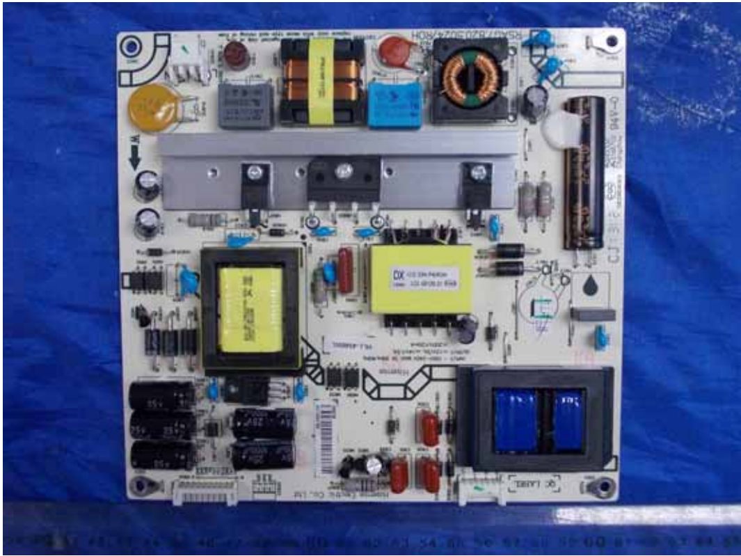
FIGURE 7 LED LCD TV (M/N: 50K366GW) POWER BOARD (COMPONENT SIDE)
