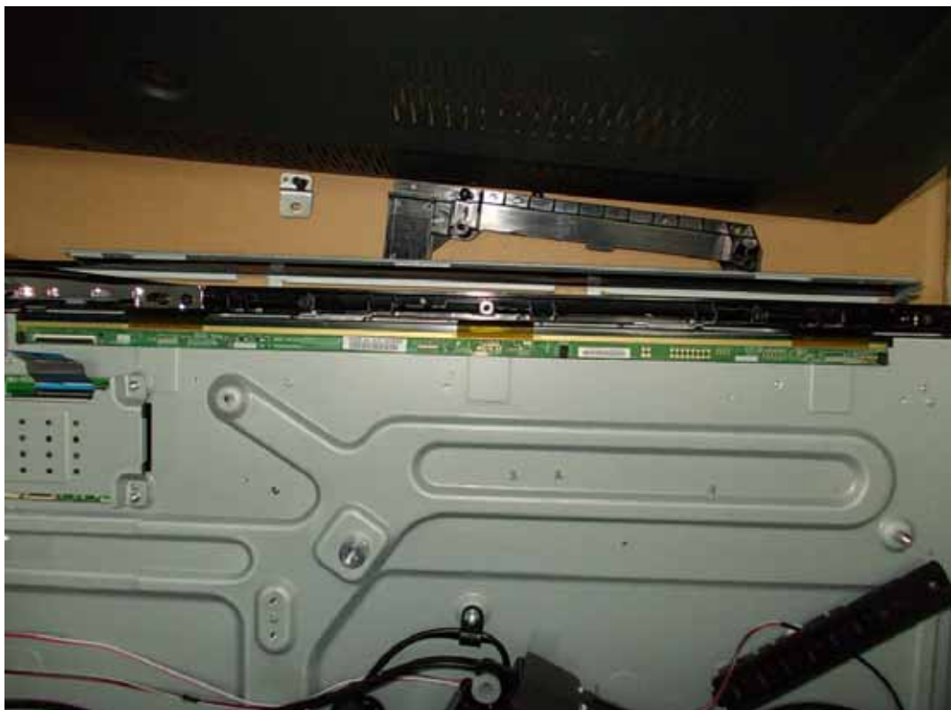
FIGURE 22 LED LCD TV (M/N: 50K366GW) LCD PANEL CONTROL BOARD #2
