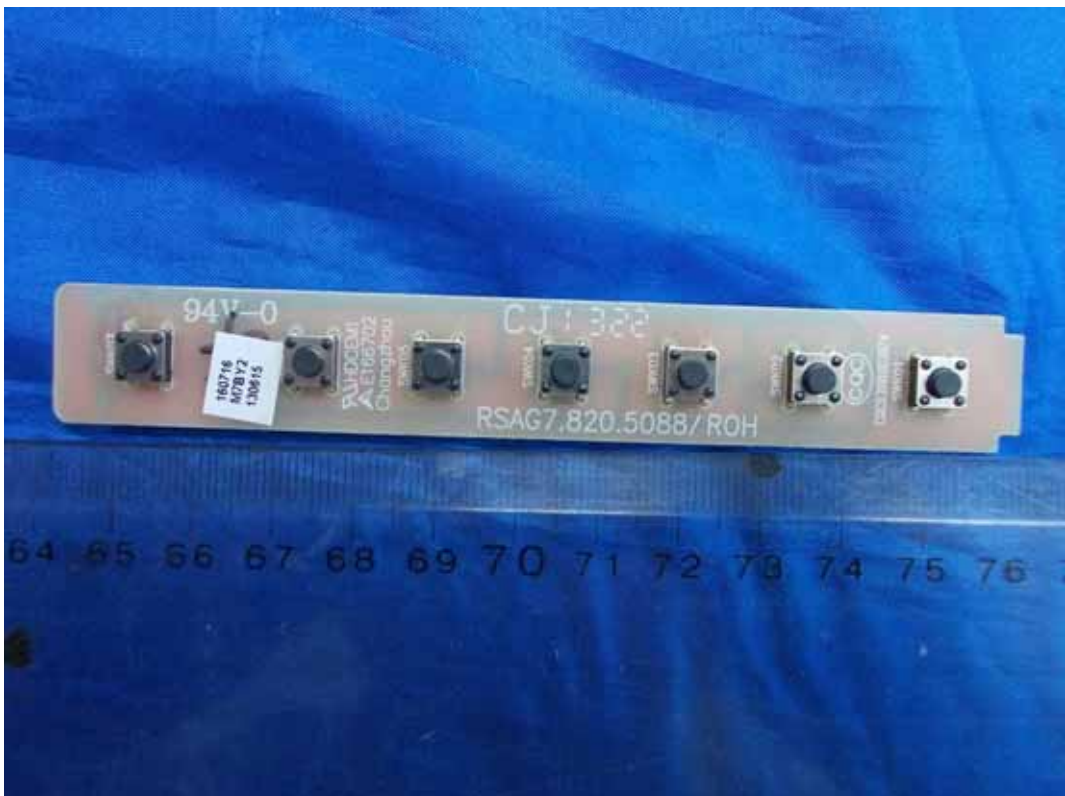
FIGURE 16 LED LCD TV (M/N: 50K366GW) KEY BOARD (COMPONENT SIDE)
