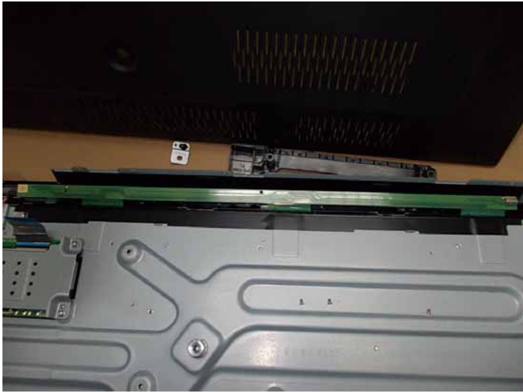
FIGURE 23 LED LCD TV (M/N: 50K366GW) LCD PANEL CONTROL BOARD #2
