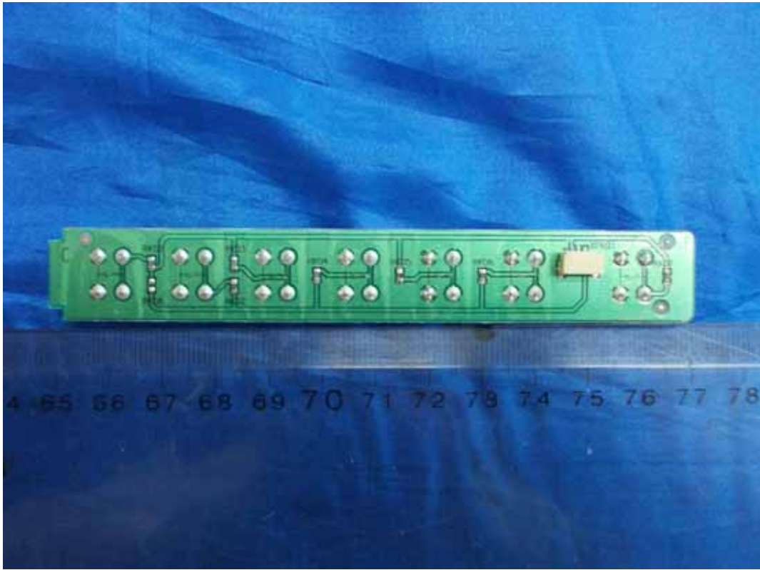
FIGURE 17 LED LCD TV (M/N: 50K366GW) KEY BOARD (SOLDERED SIDE)
