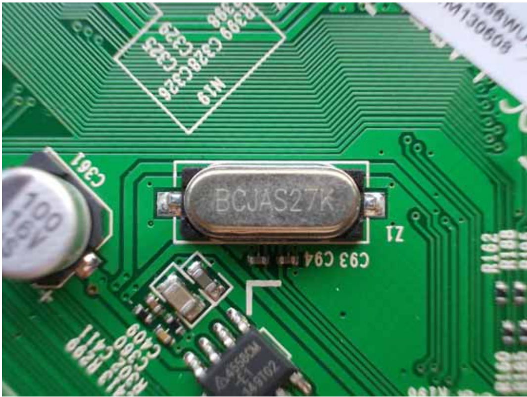
FIGURE 15 LED LCD TV (M/N: 50K366GW) CHIP #2 & CRYSTAL #1 ON MAIN BOARD
