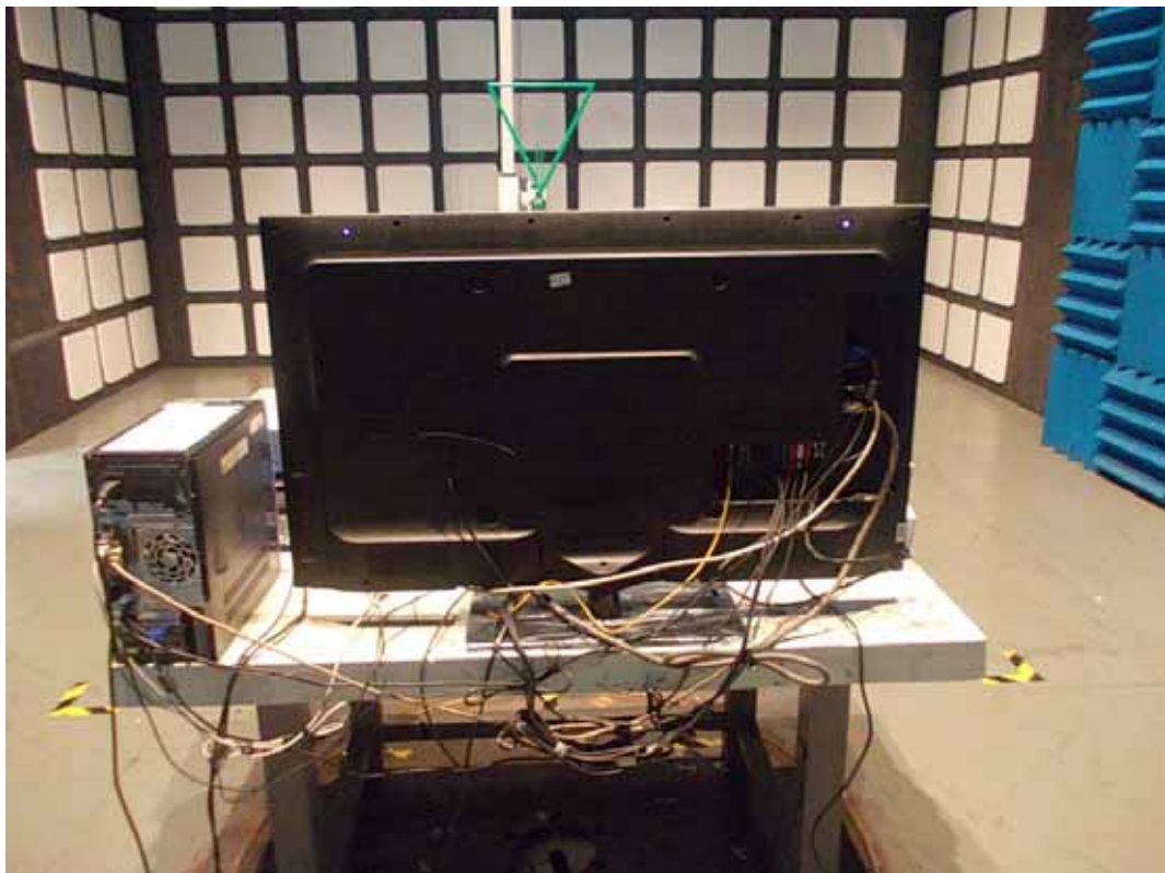
BACK VIEW OF RADIATED EMISSION TEST
