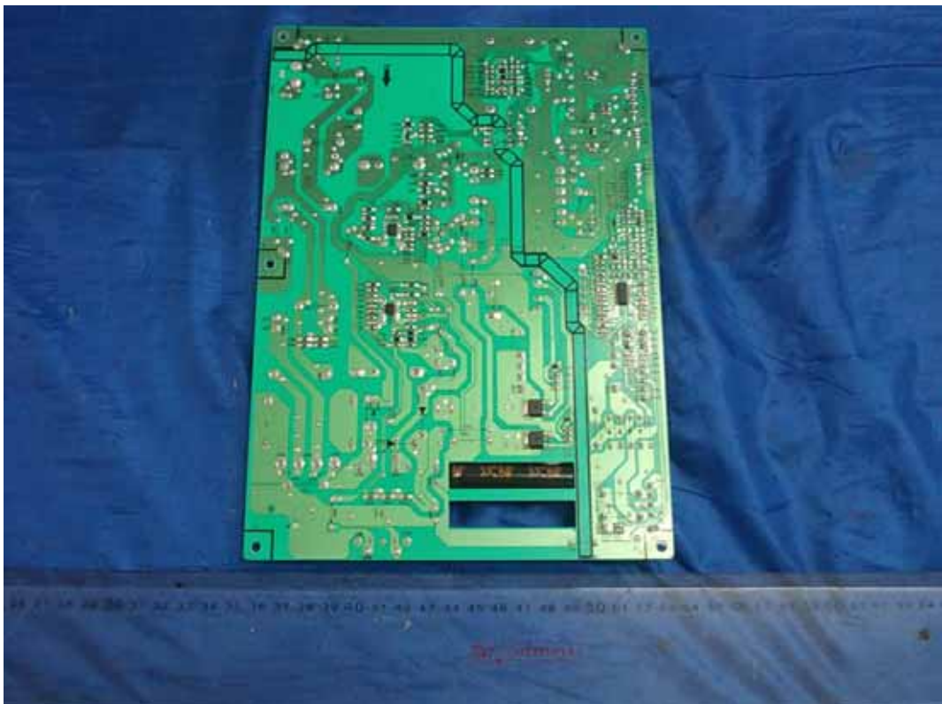
FIGURE 4 LED LCD TV (M/N: 55K610GWN) POWER BOARD (SOLDERED SIDE)
