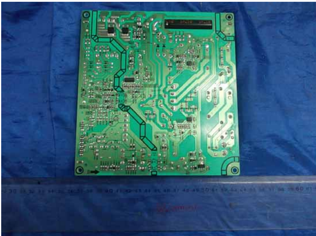
FIGURE 4 LED LCD TV (M/N: 50K610GWN) POWER BOARD (SOLDERED SIDE)
