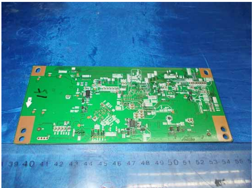
FIGURE 17 LED LCD TV (M/N: 50K610GWN) LCD PANEL CONTROL BOARD (SOLDERED SIDE)
