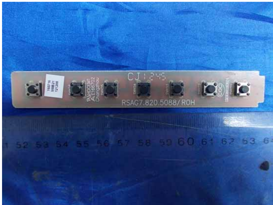
FIGURE 13 LED LCD TV (M/N: LTDN55K610GWUS) KEY BOARD (COMPONENT SIDE)
