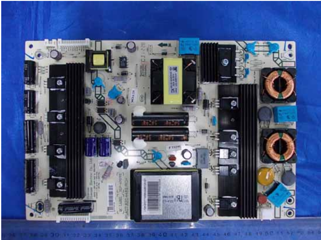
FIGURE 4 LED LCD TV (M/N: LTDN55XT710XWUS3D) POWER BOARD (COMPONENT SIDE)
