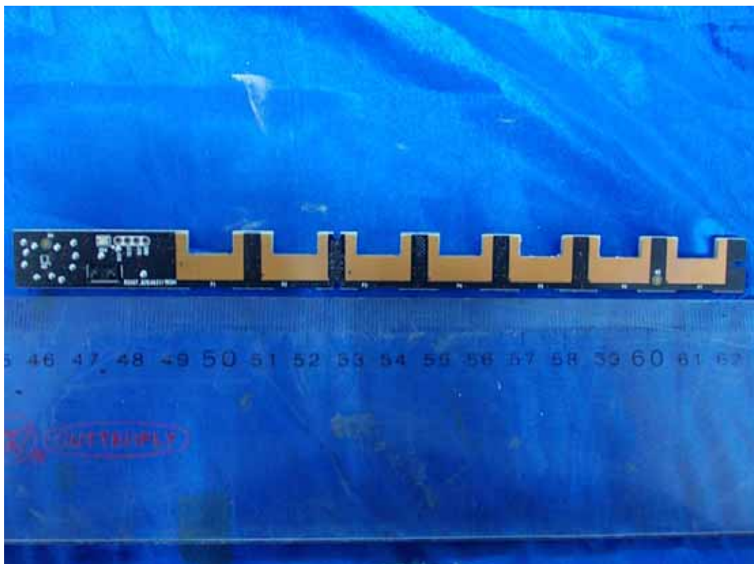
FIGURE 15 LED LCD TV (M/N: LTDN55XT710XWUS3D) KEY BOARD (SOLDERED SIDE)
