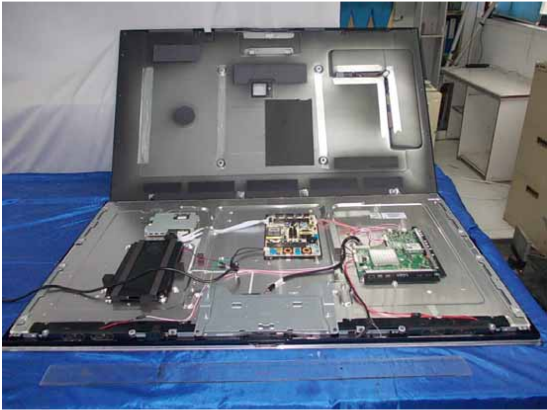
FIGURE 1 LED LCD TV (M/N: LTDN55XT710XWUS3D) COVER REMOVED
