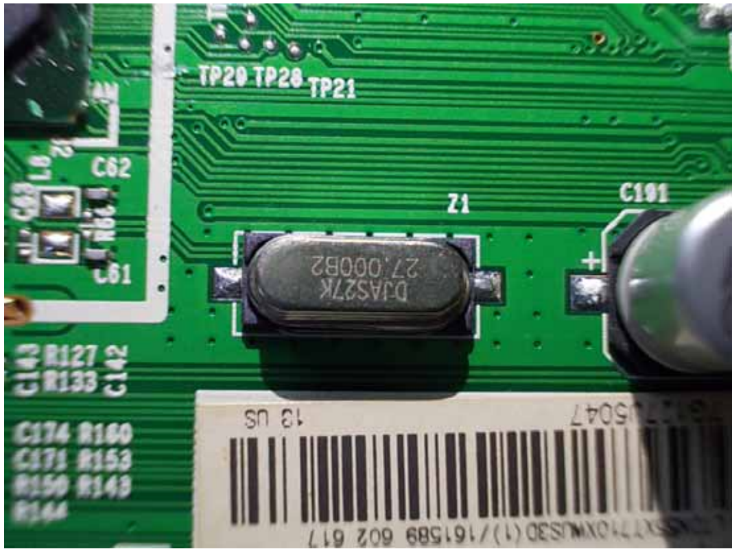
FIGURE 10 LED LCD TV (M/N: LTDN55XT710XWUS3D) CHIP #2 & CRYSTAL #2 ON MAIN BOARD
