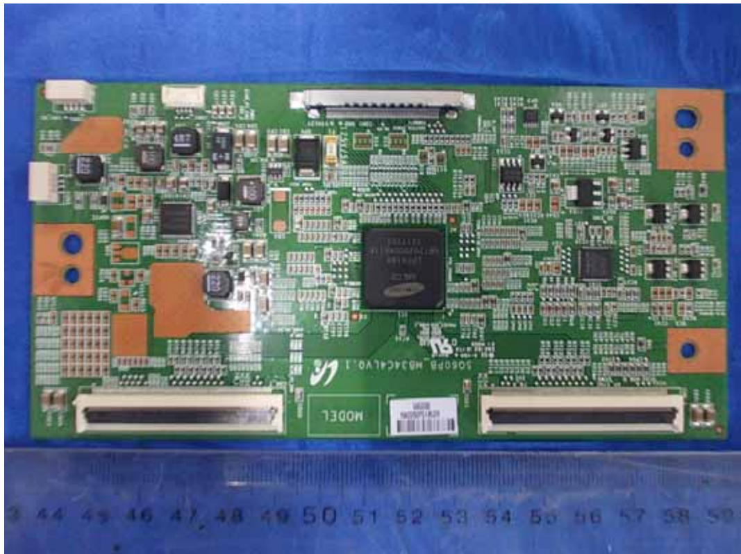
FIGURE 19 LED LCD TV (M/N: LTDN55XT710XWUS3D) LCD PANEL CONTROL BOARD (COMPONENT SIDE)
