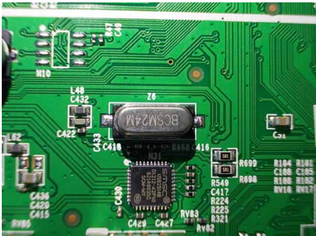
FIGURE 11 LED LCD TV (M/N: LTDN55XT710XWUS3D) CRYSTAL #3 ON MAIN BOARD
