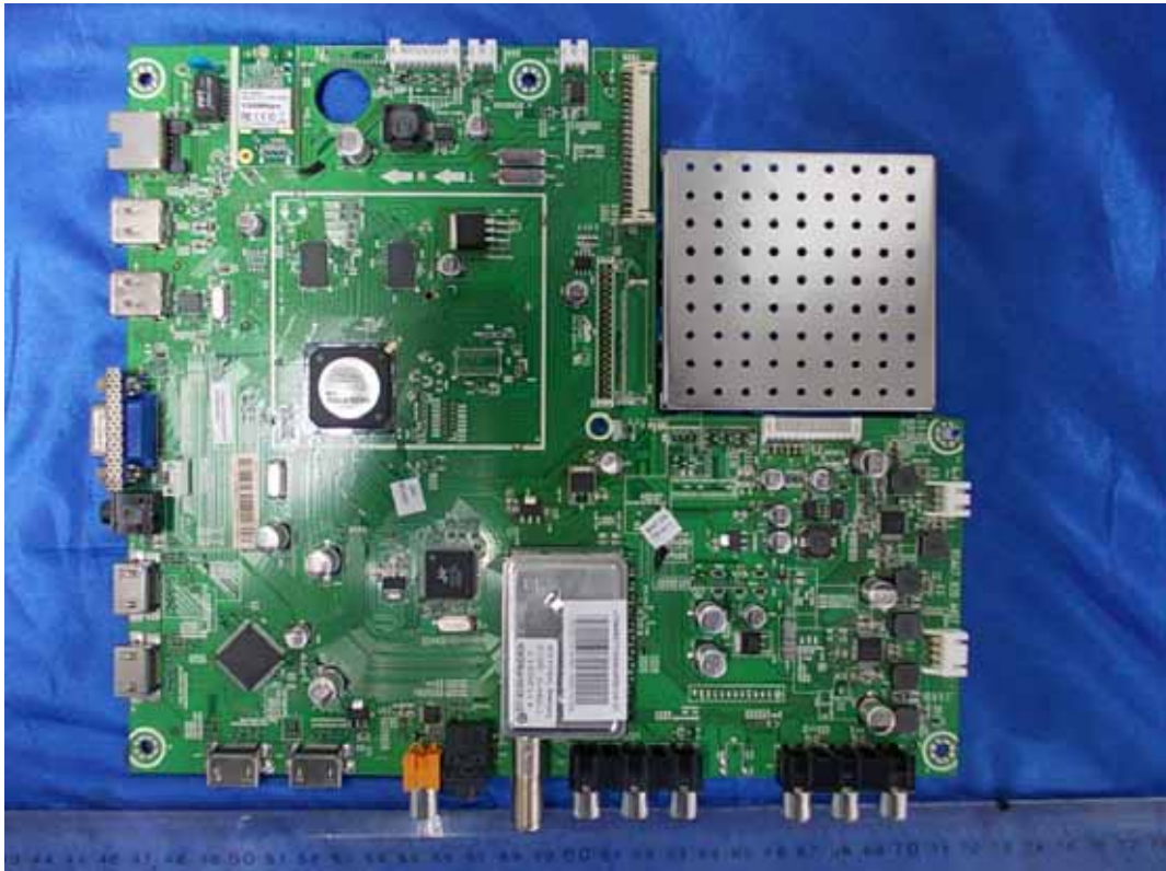
FIGURE 6 LED LCD TV (M/N: LTDN55XT710XWUS3D) MAIN BOARD (COMPONENT SIDE)
