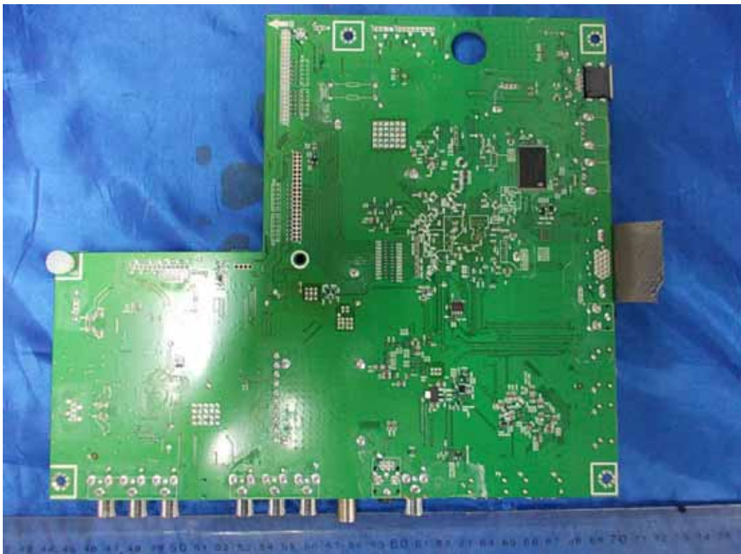
FIGURE 7 LED LCD TV (M/N: LTDN55XT710XWUS3D) MAIN BOARD (SOLDERED SIDE)
