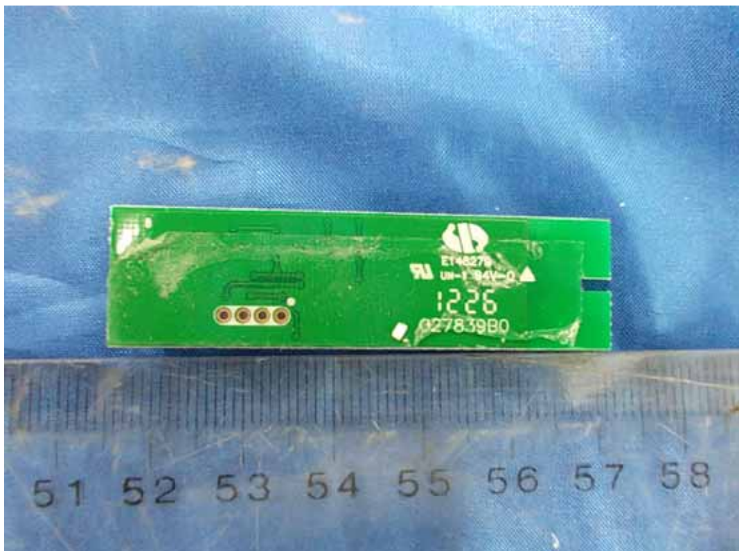
FIGURE 17 LED LCD TV (M/N: LTDN55XT710XWUS3D) RF BOARD (SOLDERED SIDE)
