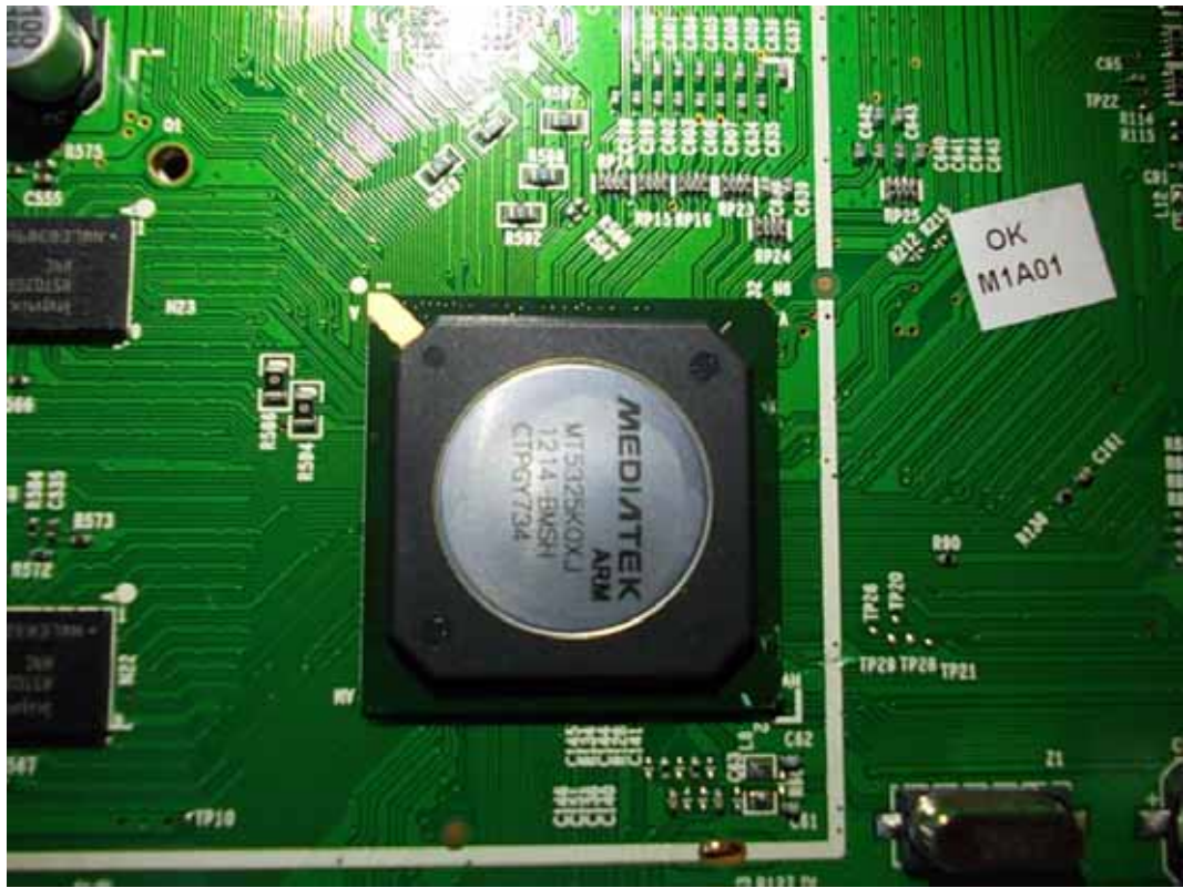
FIGURE 12 LED LCD TV (M/N: LTDN55XT710XWUS3D) CHIP #2 & CRYSTAL #2 ON MAIN BOARD
