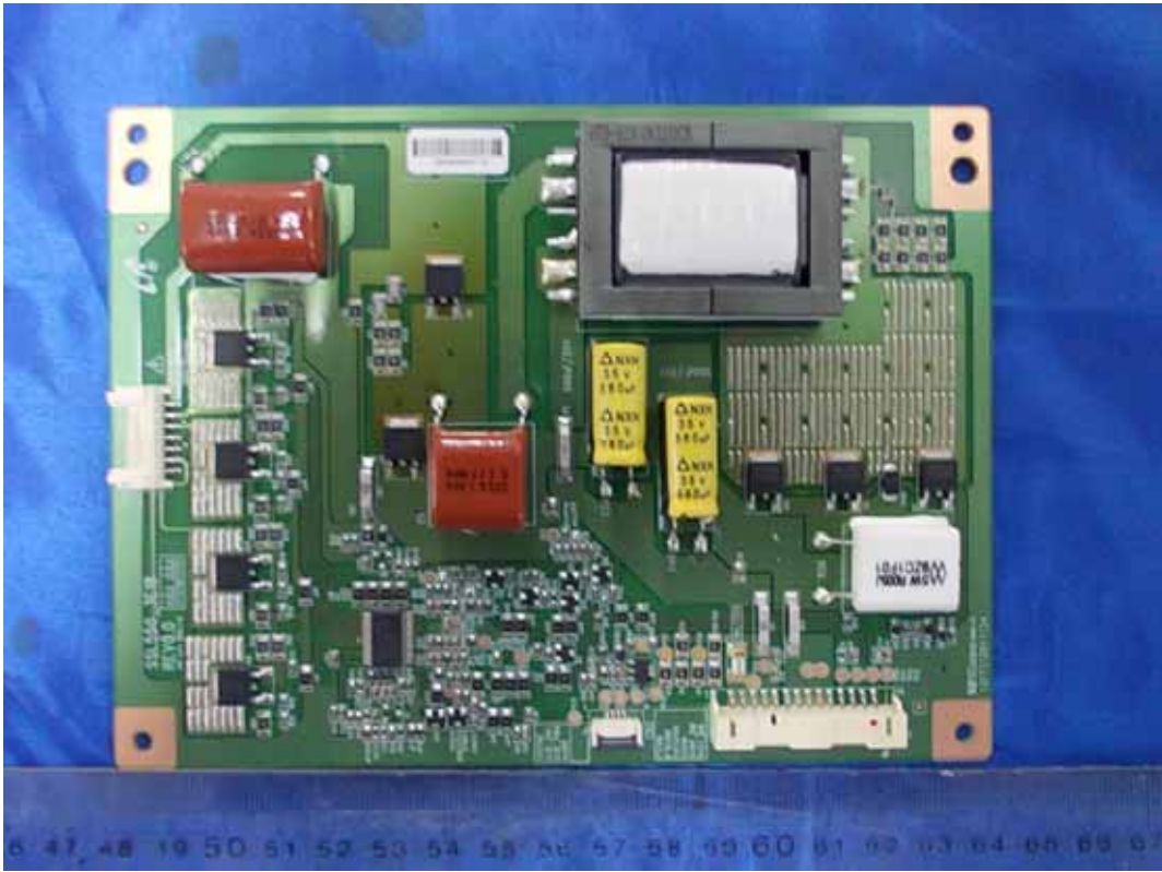
FIGURE 21 LED LCD TV (M/N: LTDN55XT710XWUS3D) HIGH VOLTAGE SIGNAL BOARD (COMPONENT SIDE)
