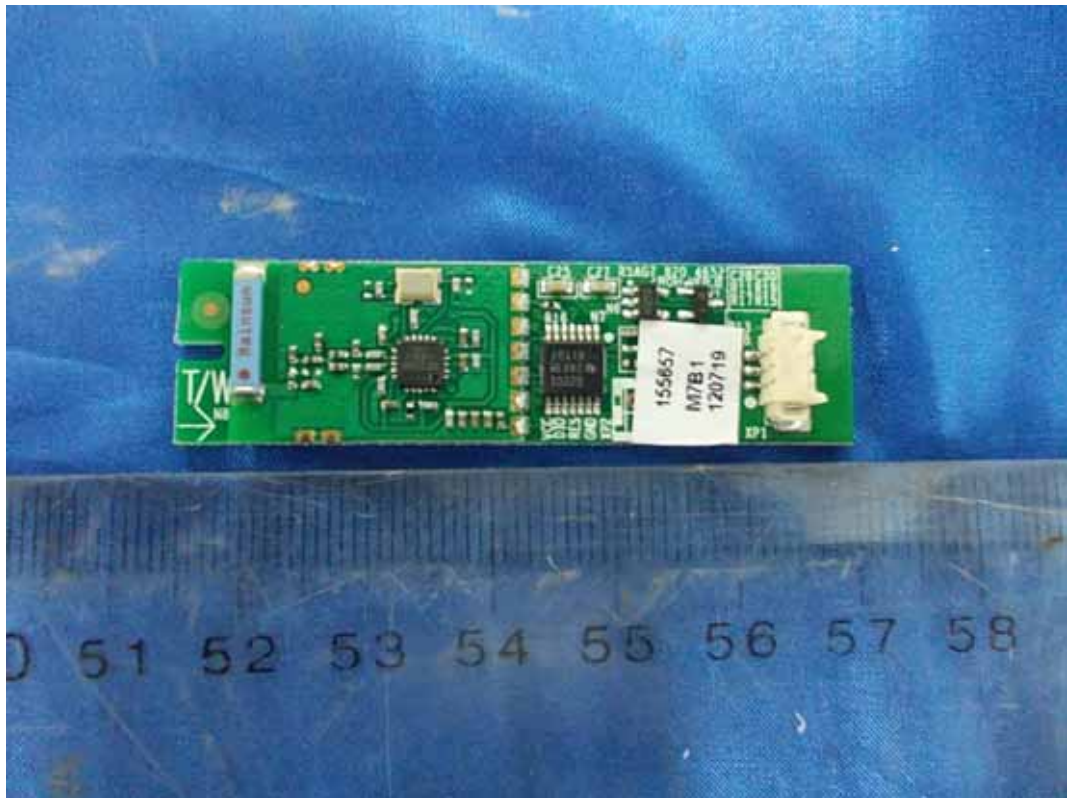
FIGURE 16 LED LCD TV (M/N: LTDN55XT710XWUS3D) RF BOARD (COMPONENT SIDE)
