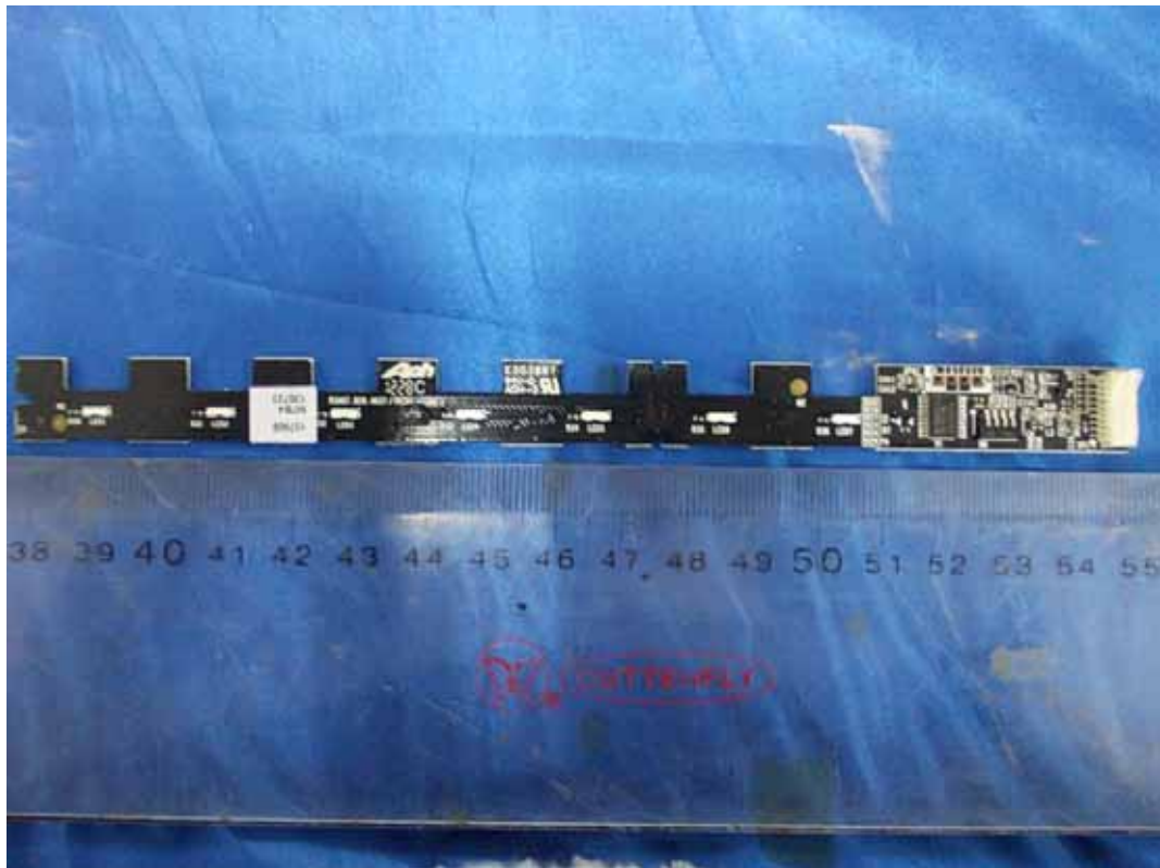
FIGURE 14 LED LCD TV (M/N: LTDN55XT710XWUS3D) KEY BOARD (COMPONENT SIDE)
