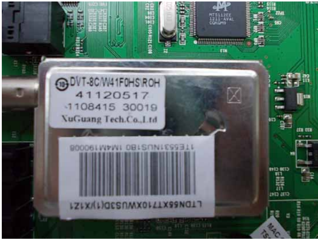
FIGURE 8 LED LCD TV (M/N: LTDN55XT710XWUS3D) TUNER ON MAIN BOARD
