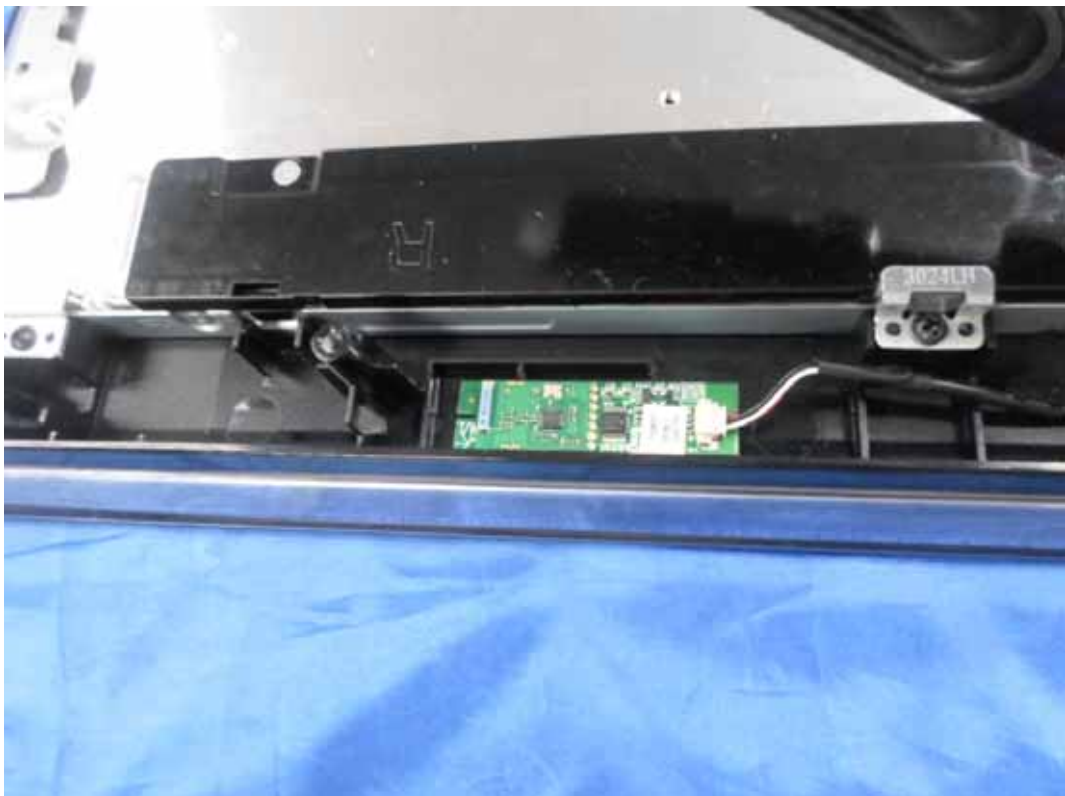
FIGURE 2 LED LCD TV (M/N: LTDN46K316XWUS3D) RF BOARD POSITION
