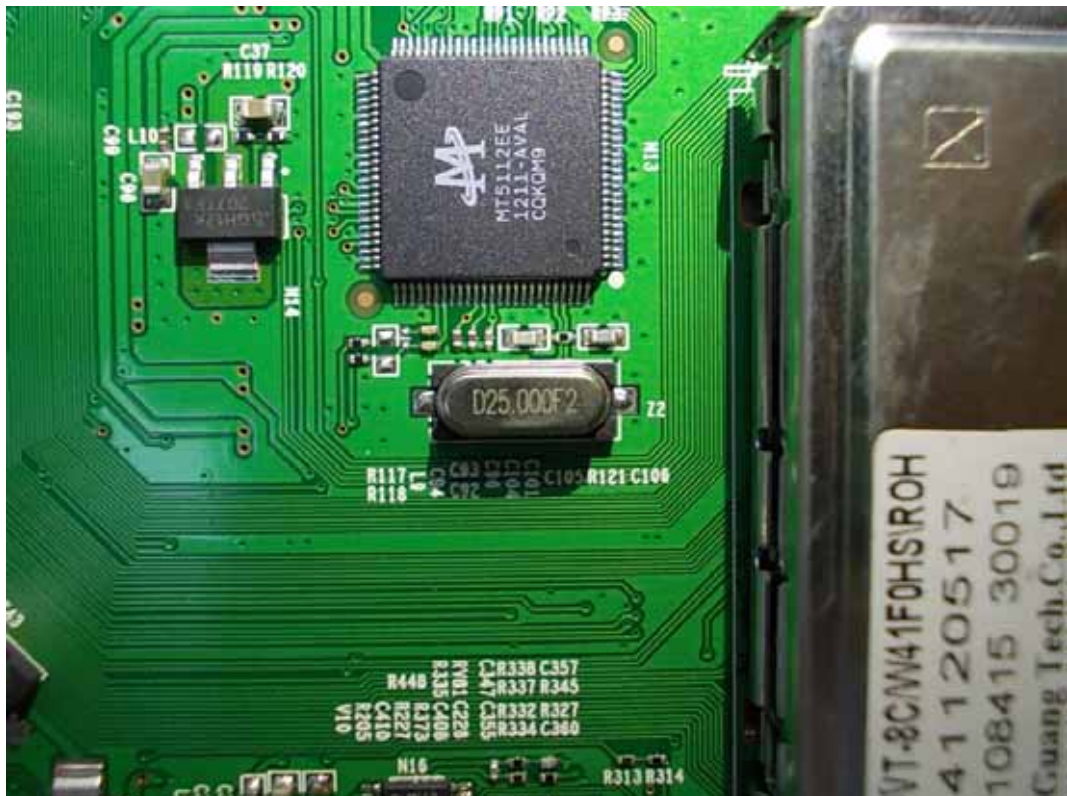
FIGURE 9 LED LCD TV (M/N: LTDN55XT710XWUS3D) CHIP #1 & CRYSTAL #1 ON MAIN BOARD
