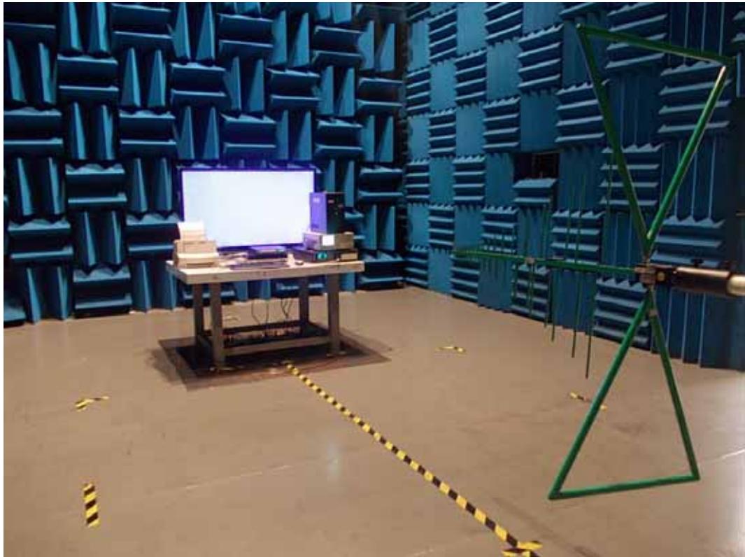
FRONT VIEW OF RADIATED EMISSION TEST
