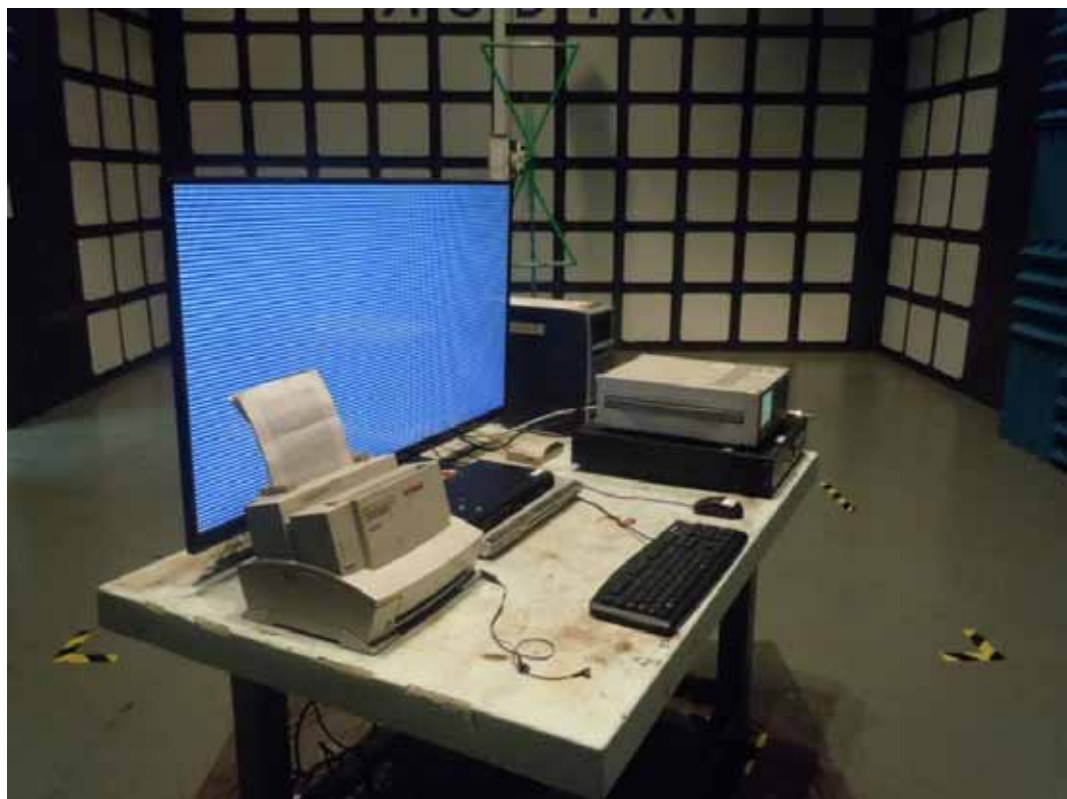
SETUP WITH MAXIMUM DETECTED EMISSION AT VERTICAL POLARIZATION (TEST MODE: D-SUB 1024*768@60Hz)
