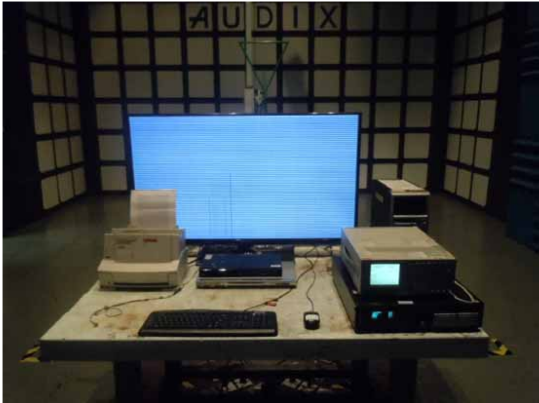
FRONT VIEW OF RADIATED EMISSION TEST
