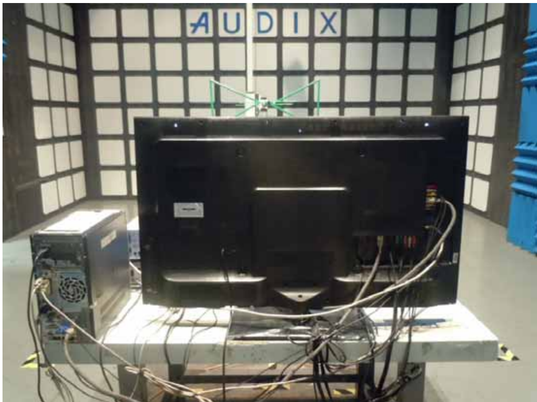
BACK VIEW OF RADIATED EMISSION TEST
