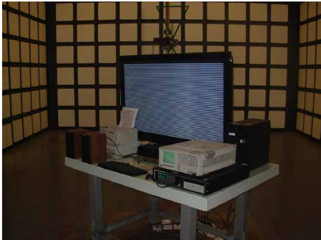
SETUP WITH MAXIMUM DETECTED EMISSION AT VERTICAL POLARIZATION (HDMI 640*480@60Hz)
