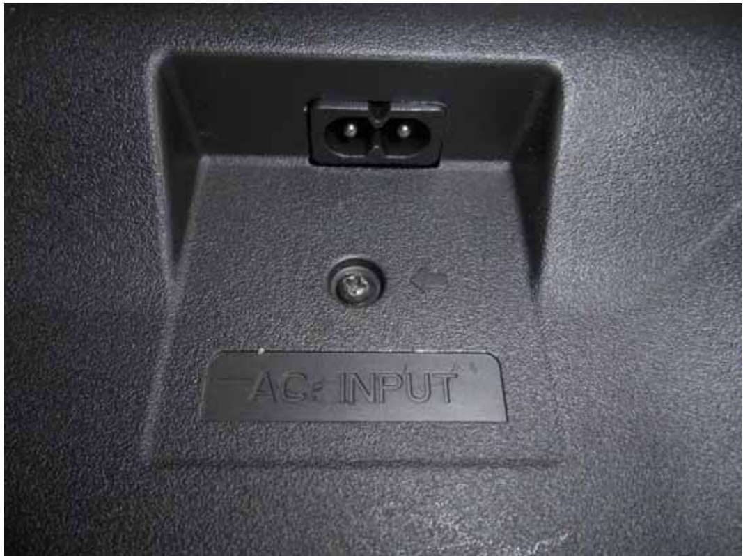
FIGURE 3 LED LCD TV (M/N: 48H4C) AC PORTS #1
