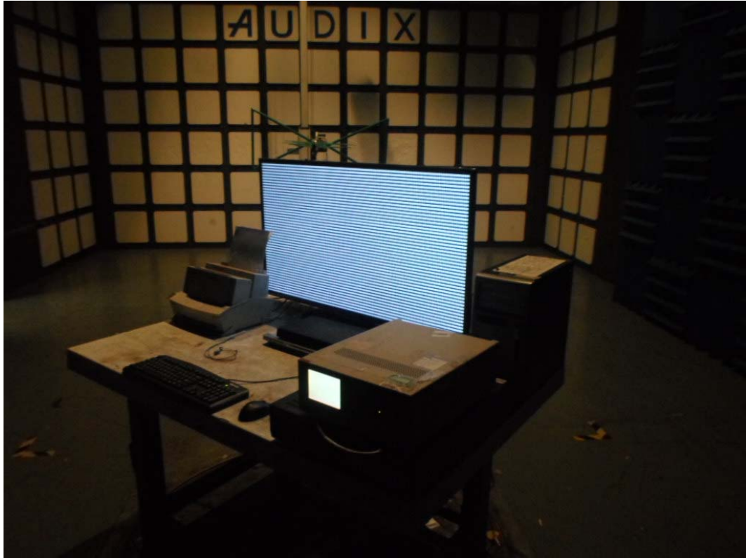
SETUP WITH MAXIMUM DETECTED EMISSION AT HORIZONTAL POLARIZATION (TEST MODE: HDMI 1280*1024@60Hz)
