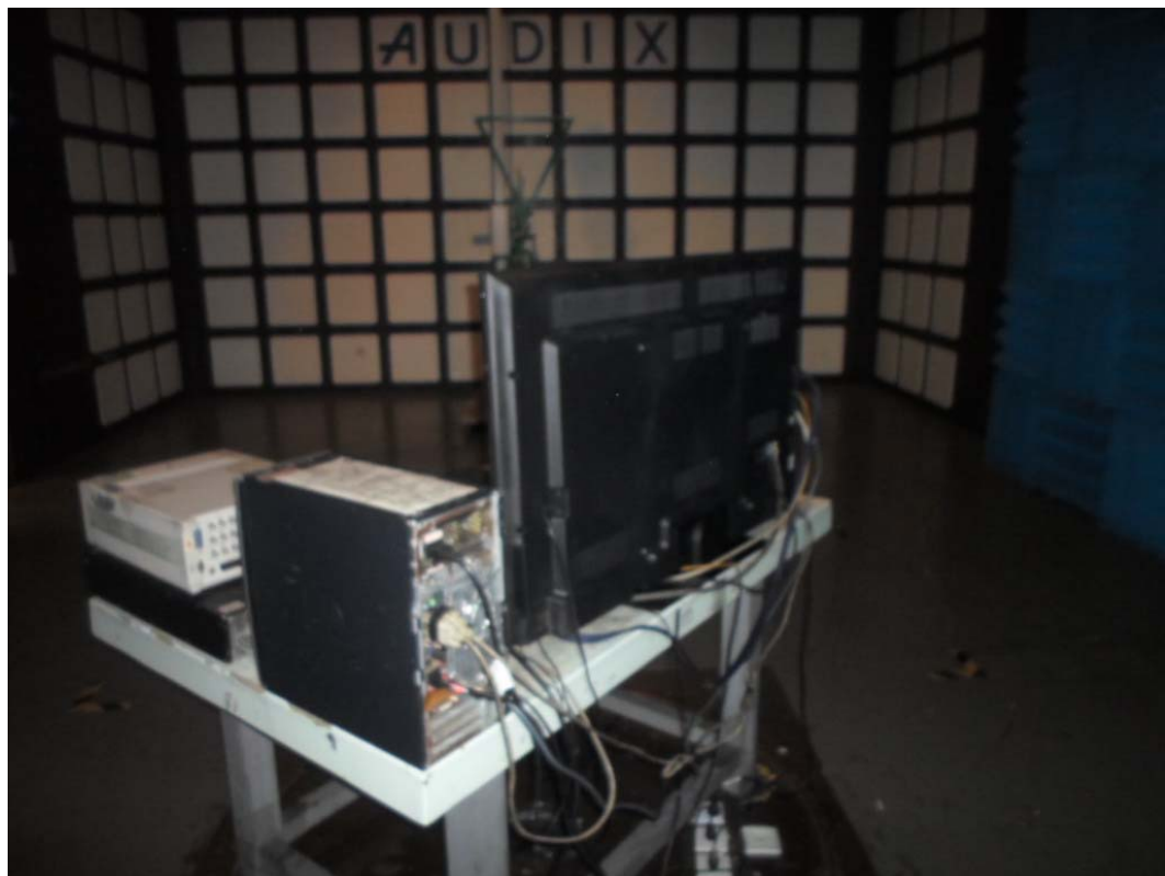
SETUP WITH MAXIMUM DETECTED EMISSION AT VERTICAL POLARIZATION (TEST MODE: HDMI 1280*1024@60Hz)
