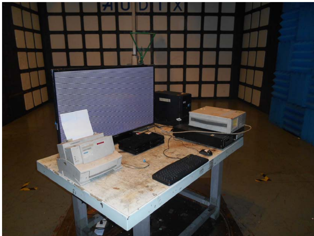
SETUP WITH MAXIMUM DETECTED EMISSION AT VERTICAL POLARIZATION (TEST MODE: D-SUB 1024*768@60Hz & 1 kHz PLAYING)
