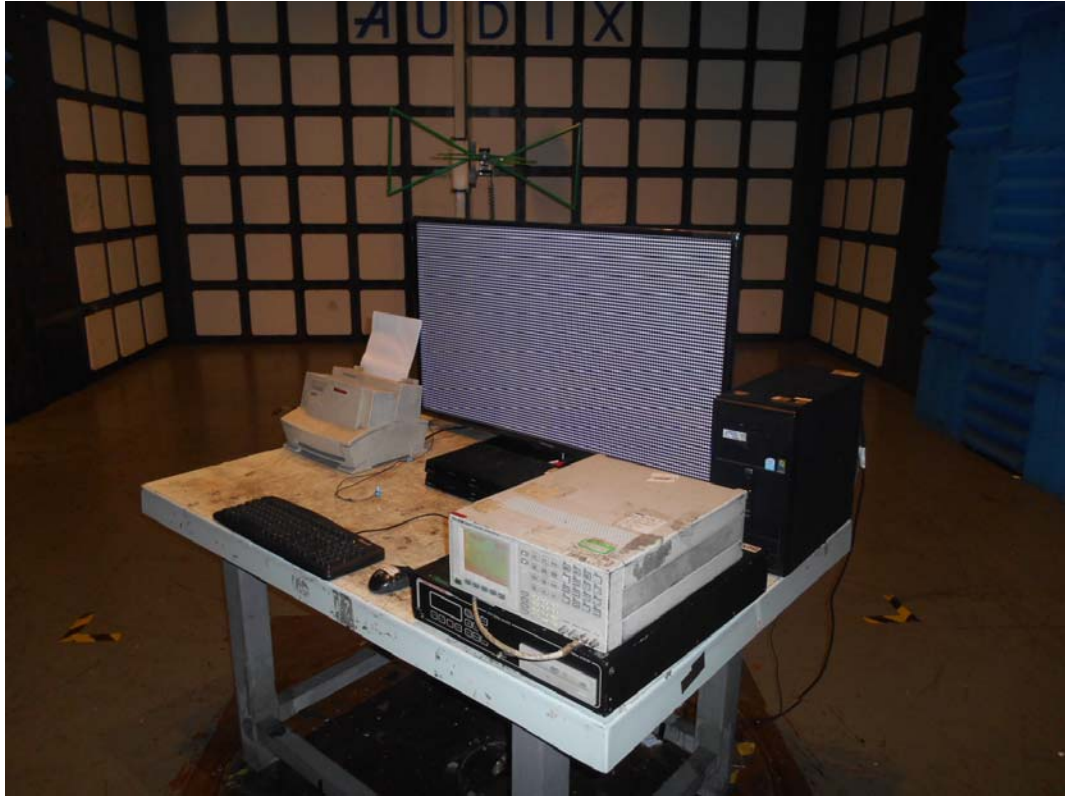
SETUP WITH MAXIMUM DETECTED EMISSION AT HORIZONTAL POLARIZATION (TEST MODE: D-SUB 1024*768@60Hz & 1 kHz PLAYING)
