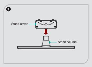
Align the stand cover with the stand column. Make sure that the bottom of the stand cover is flush against screw (M5×12). the top of the stand column.
