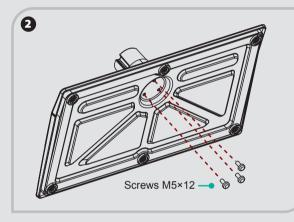
Secure the stand column to the base with 3 screws
