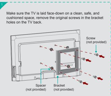
Place the spacers (not provided) in the corresponding bracket holes Follow the instructions provided with the wall-mount bracket to attach the bracket on the TV.
