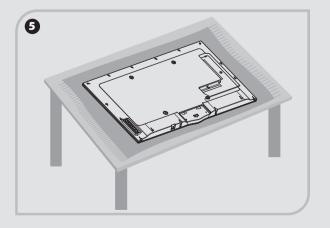
Carefully place your TV facedown on a soft, cushioned After pre-installing the stand, secure the stand to the surface to prevent damage to the TV or scratching to TV with the 4 screws (M5×12). the screen.
