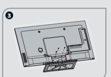
Secure the stand to the TV with the 4 Screws A (M5 x 12).
