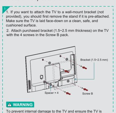
mounted securely, use only the 4 screws in the Screw B pack.
