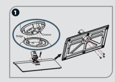
Align the front of the stand column with the front of the base, then insert the stand column into the base making sure that the groove in the stand column aligns with the ridge in the base. Secure the stand column to the base with 3 Screws A (M5 x 12)
