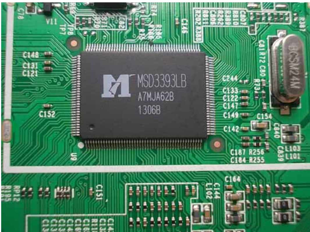
FIGURE 8 LED LCD TV (M/N: 46K360MN) CRYSTAL & CHIP ON MAIN BOARD
