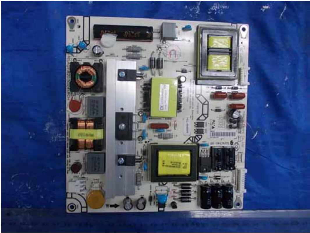
FIGURE 3 LED LCD TV (M/N: 46K360MN) POWER BOARD (COMPONENT SIDE)
