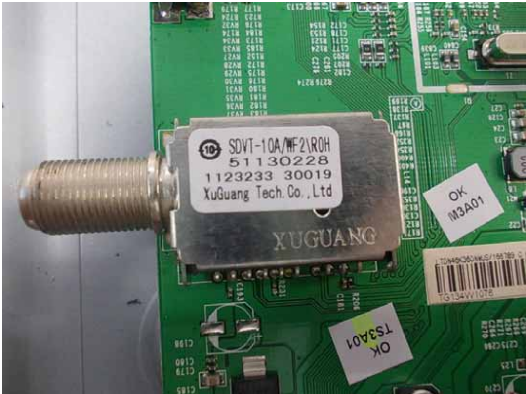
FIGURE 7 LED LCD TV (M/N: 46K360MN) TUNER ON MAIN BOARD
