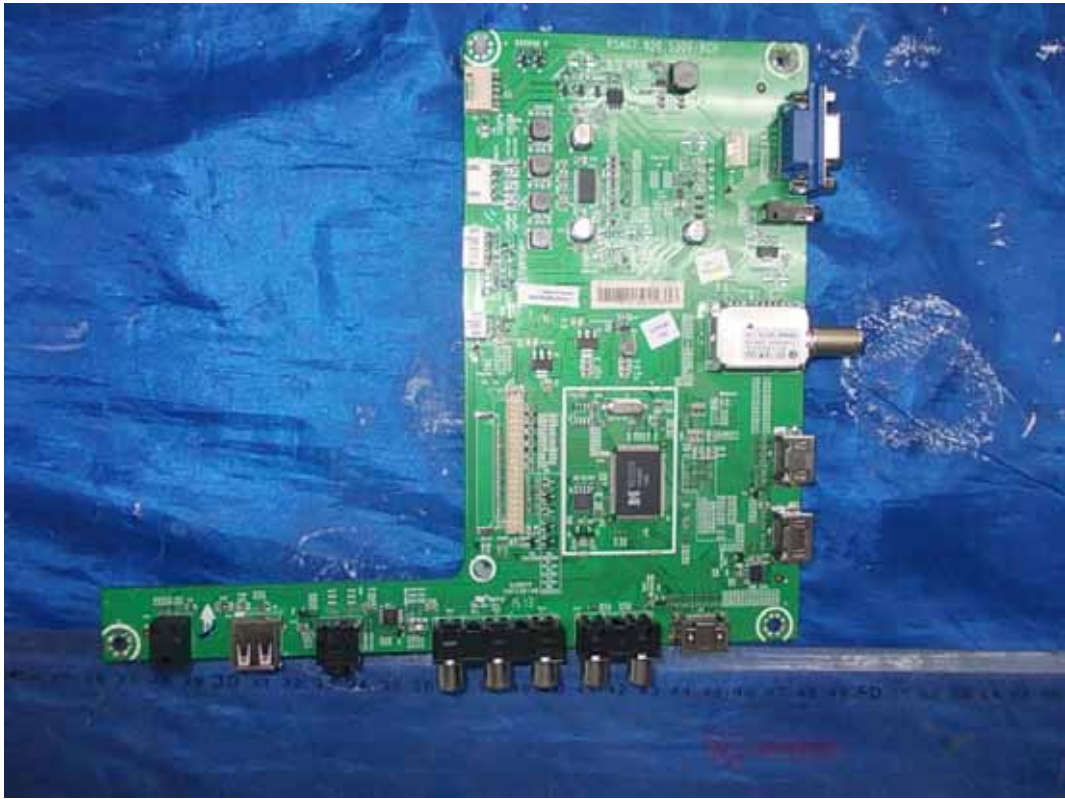
FIGURE 5 LED LCD TV (M/N: 46K360MN) MAIN BOARD (COMPONENT SIDE)
