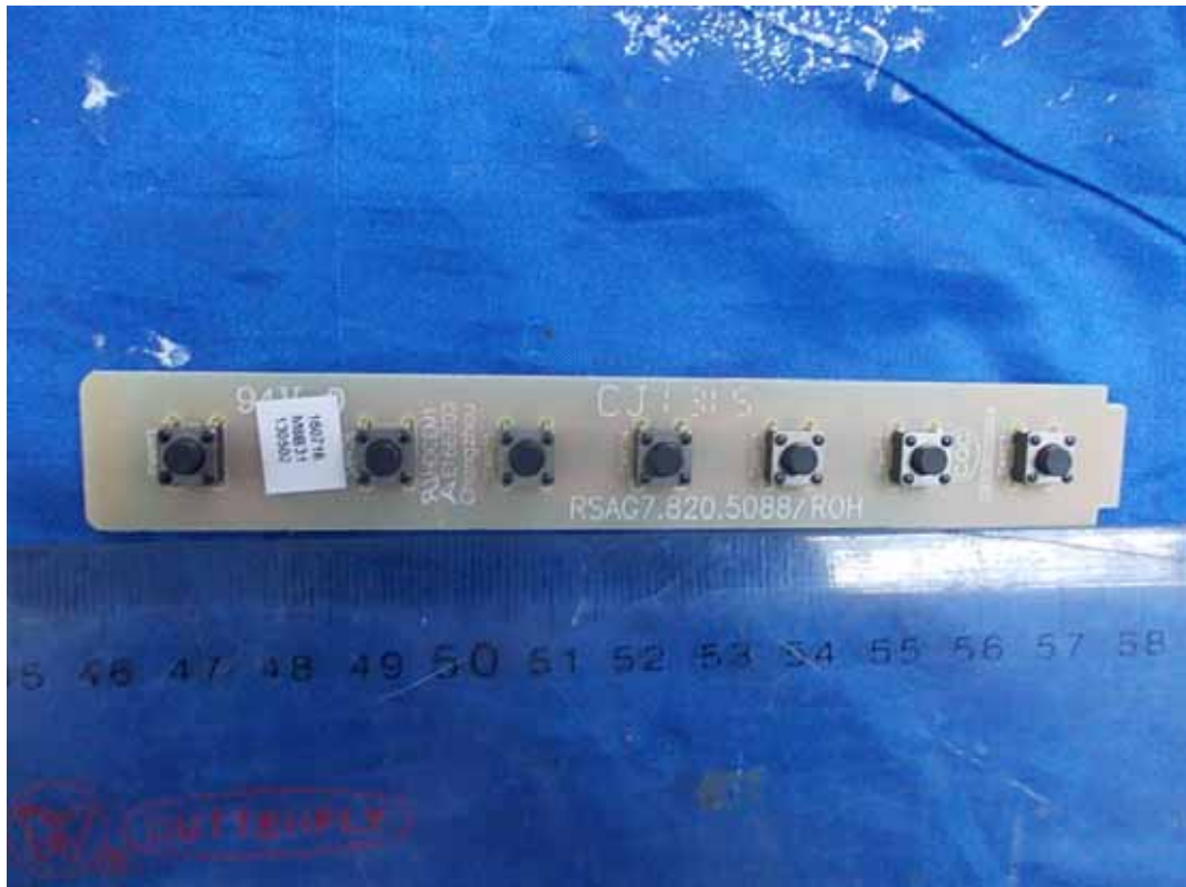
FIGURE 9 LED LCD TV (M/N: 46K360MN) KEY BOARD (COMPONENT SIDE)
