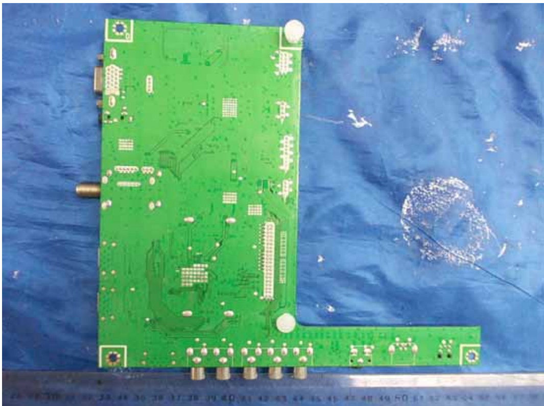
FIGURE 6 LED LCD TV (M/N: 46K360MN) MAIN BOARD (SOLDERED SIDE)
