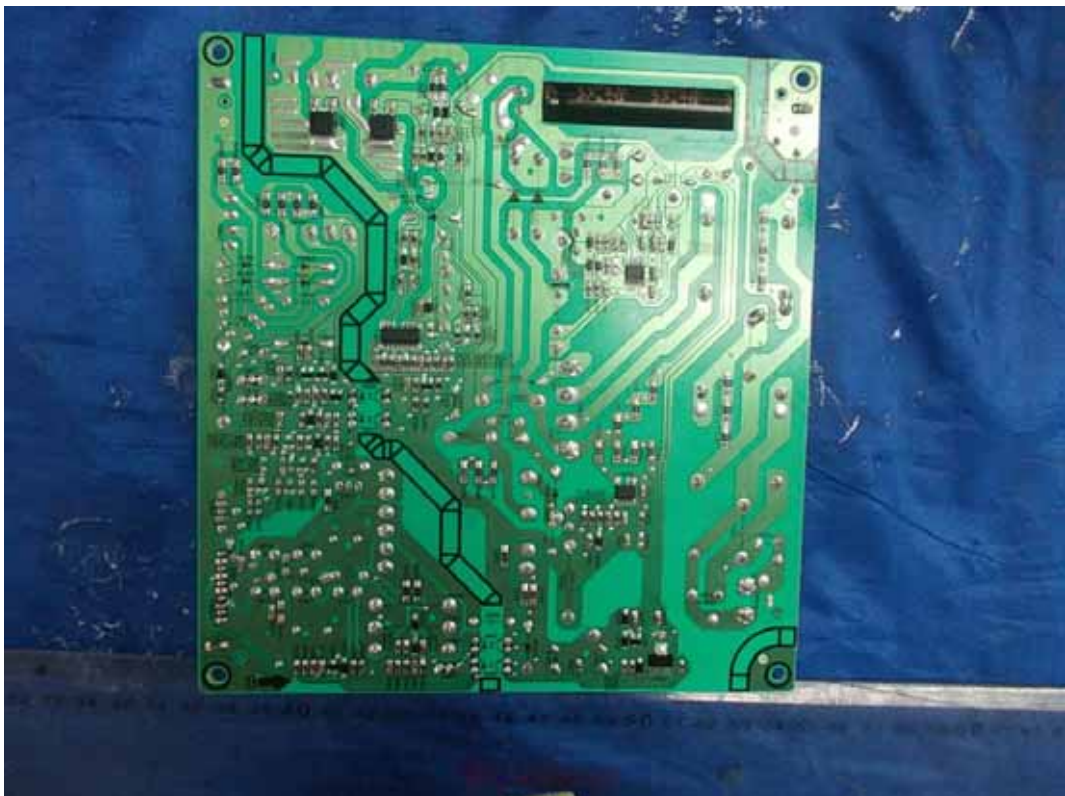
FIGURE 4 LED LCD TV (M/N: 46K360MN) POWER BOARD (SOLDERED SIDE)
