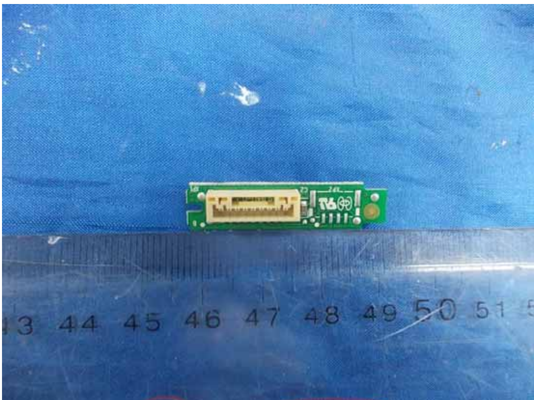
FIGURE 14 LED LCD TV (M/N: 46K360MN) IR BOARD (SOLDERED SIDE)
