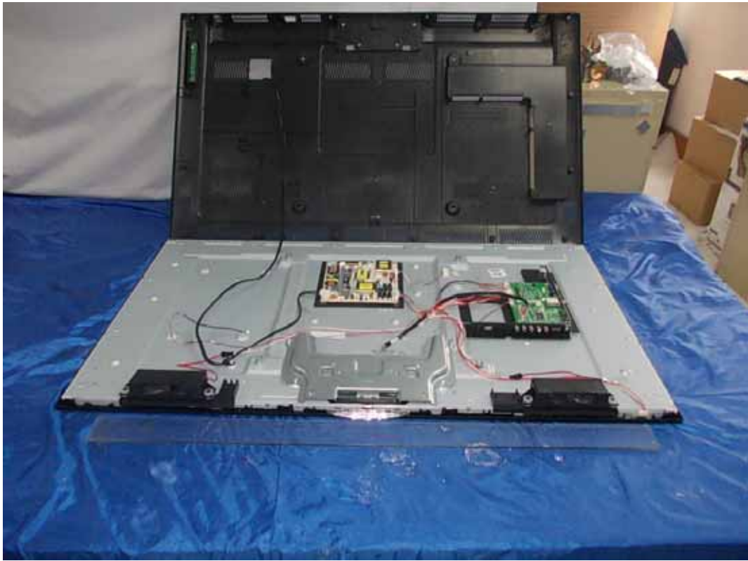
FIGURE 1 LED LCD TV (M/N: 46K360MN) COVER REMOVED
