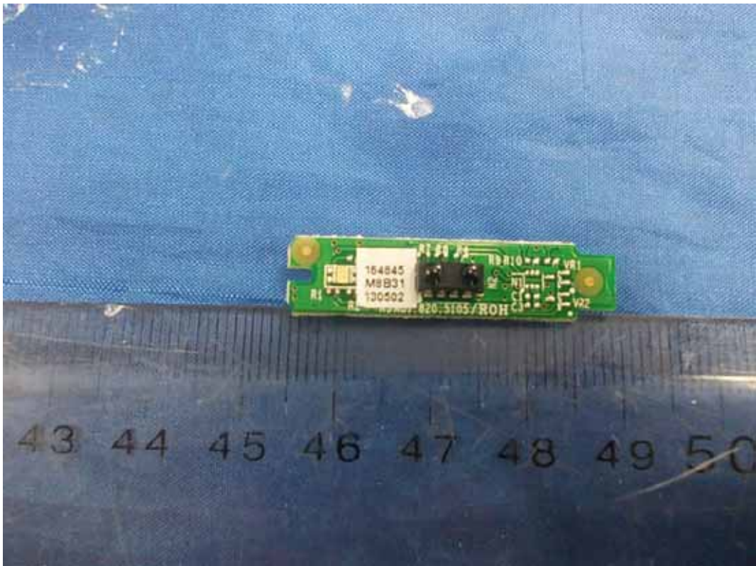
FIGURE 13 LED LCD TV (M/N: 46K360MN) IR BOARD (COMPONENT SIDE)
