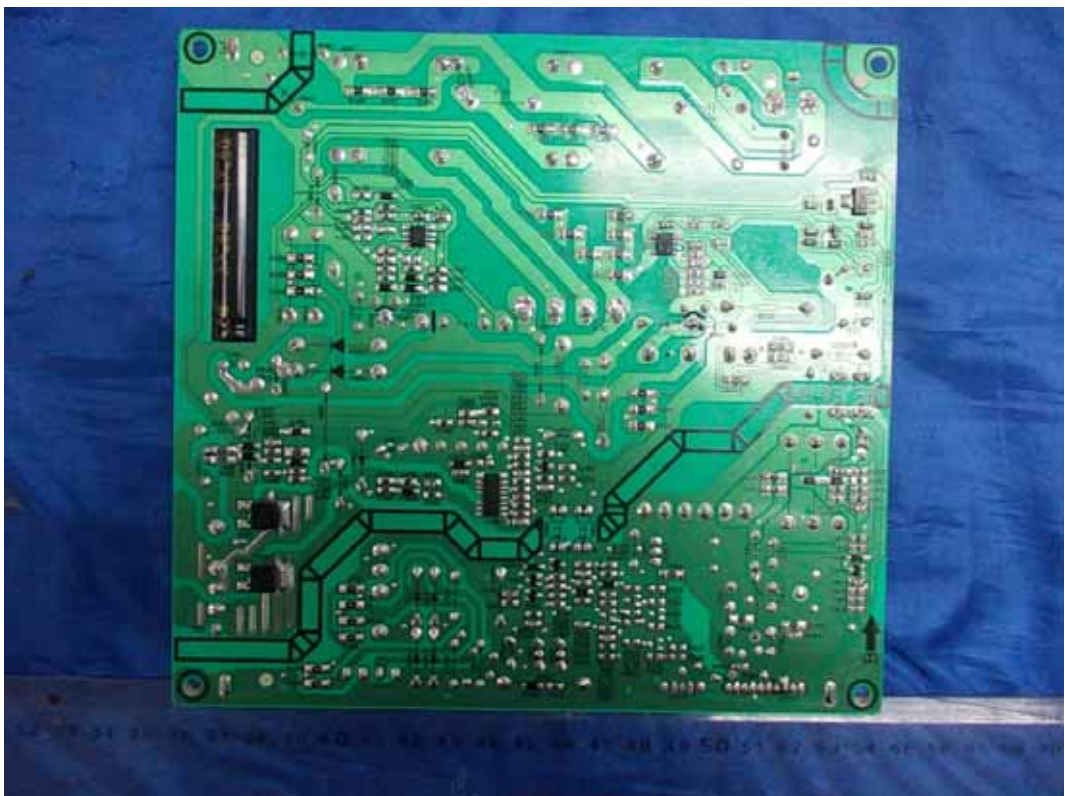
FIGURE 4 LED LCD TV (M/N: 46K366W) POWER BOARD (SOLDERED SIDE)
