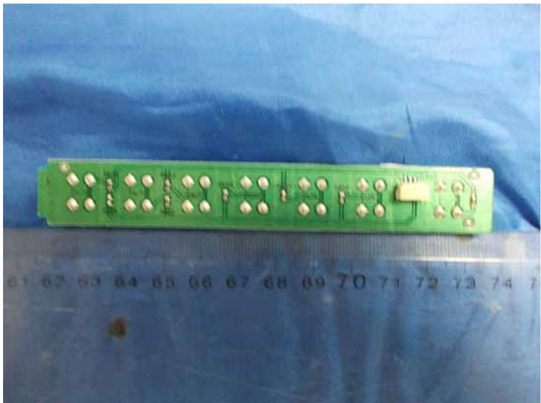
FIGURE 13 LED LCD TV (M/N: 46K366W) KEY BOARD (SOLDERED SIDE)
