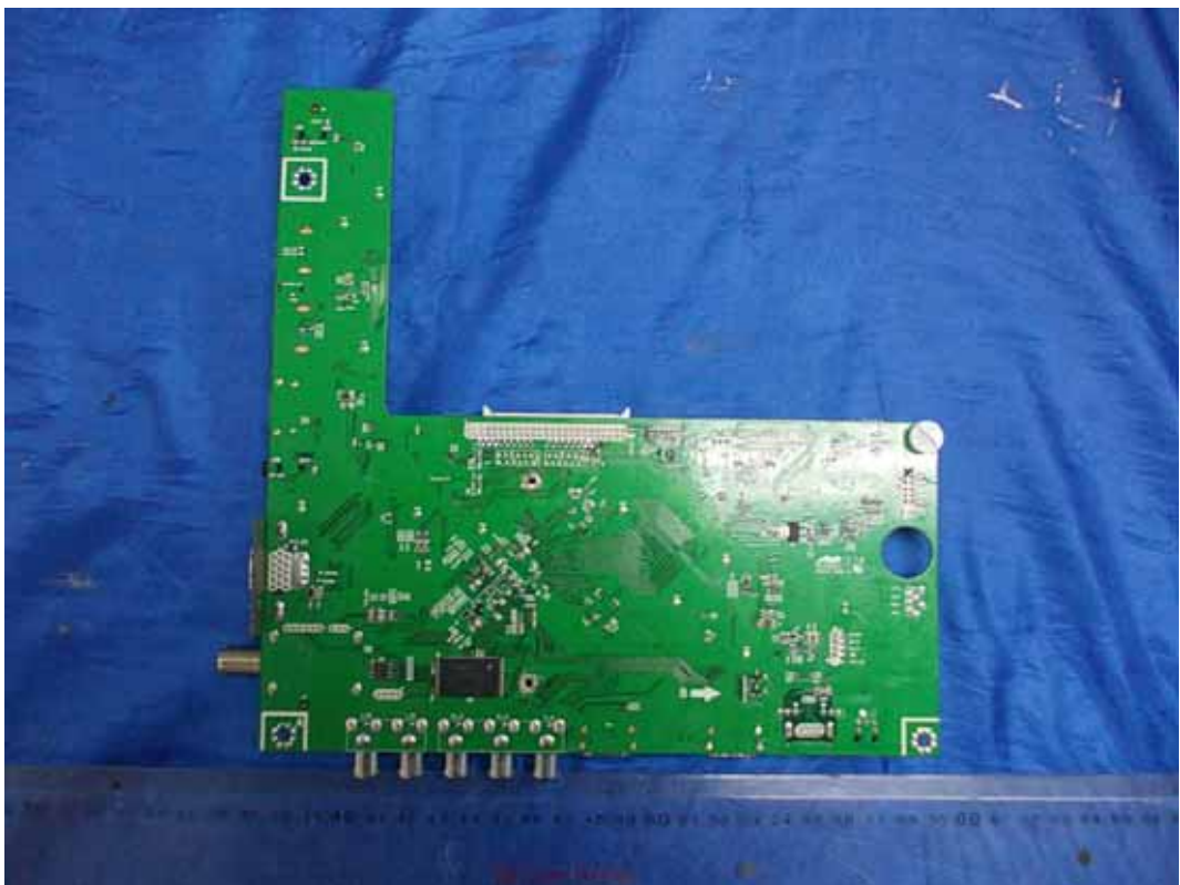
FIGURE 6 LED LCD TV (M/N: 46K366W) MAIN BOARD (SOLDERED SIDE)
