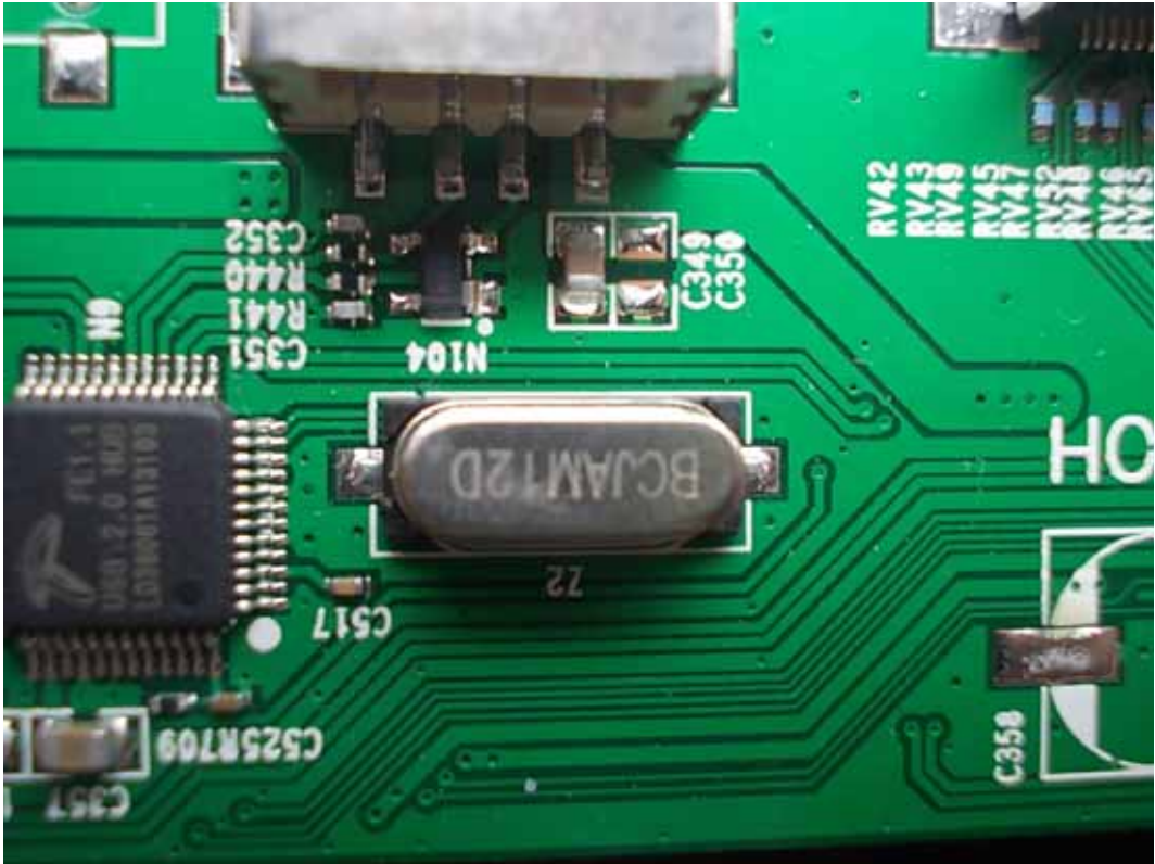
FIGURE 10 LED LCD TV (M/N: 46K366W) CRYSTAL #2 ON MAIN BOARD
