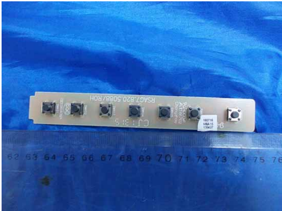
FIGURE 12 LED LCD TV (M/N: 46K366W) KEY BOARD (COMPONENT SIDE)
