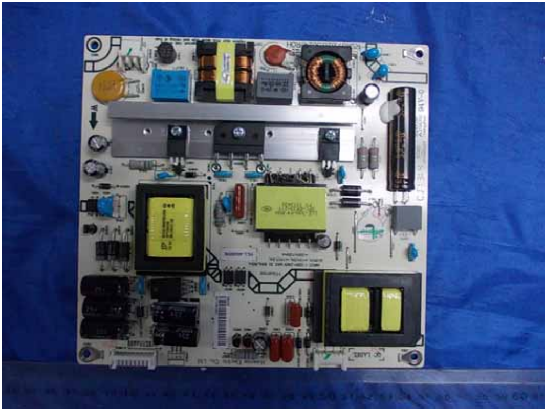
FIGURE 3 LED LCD TV (M/N: 46K366W) POWER BOARD (COMPONENT SIDE)
