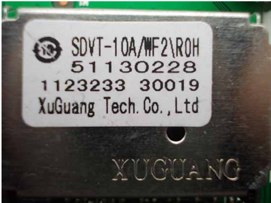
FIGURE 7 LED LCD TV (M/N: 46K366W) TUNER ON MAIN BOARD
