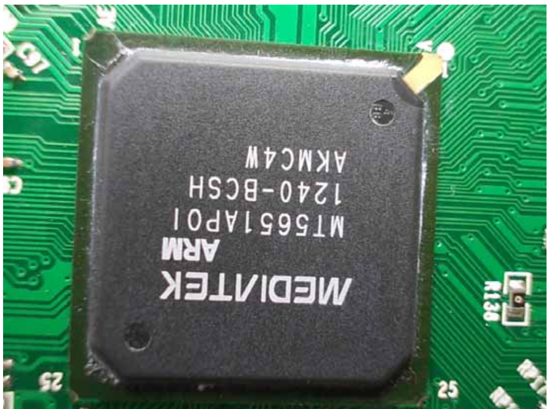
FIGURE 8 LED LCD TV (M/N: 46K366W) CHIP ON MAIN BOARD
