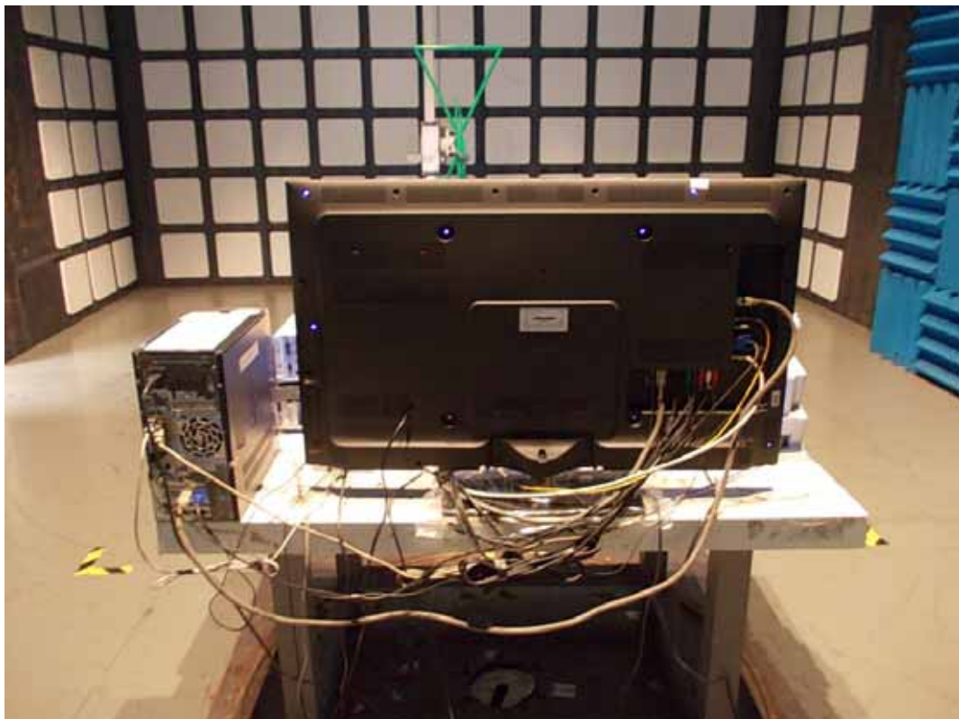
BACK VIEW OF RADIATED EMISSION TEST
