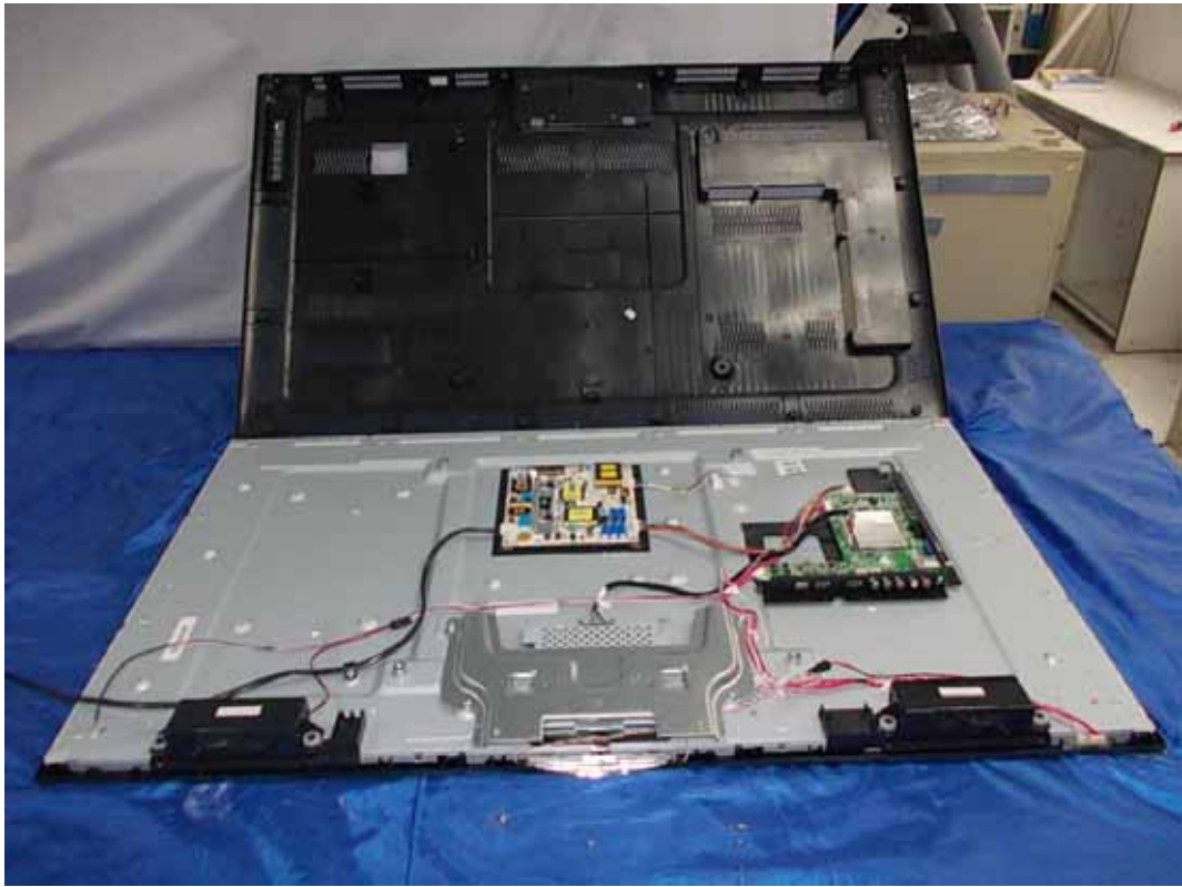
FIGURE 1 LED LCD TV (M/N: LTDN46K360MUS) COVER REMOVED
