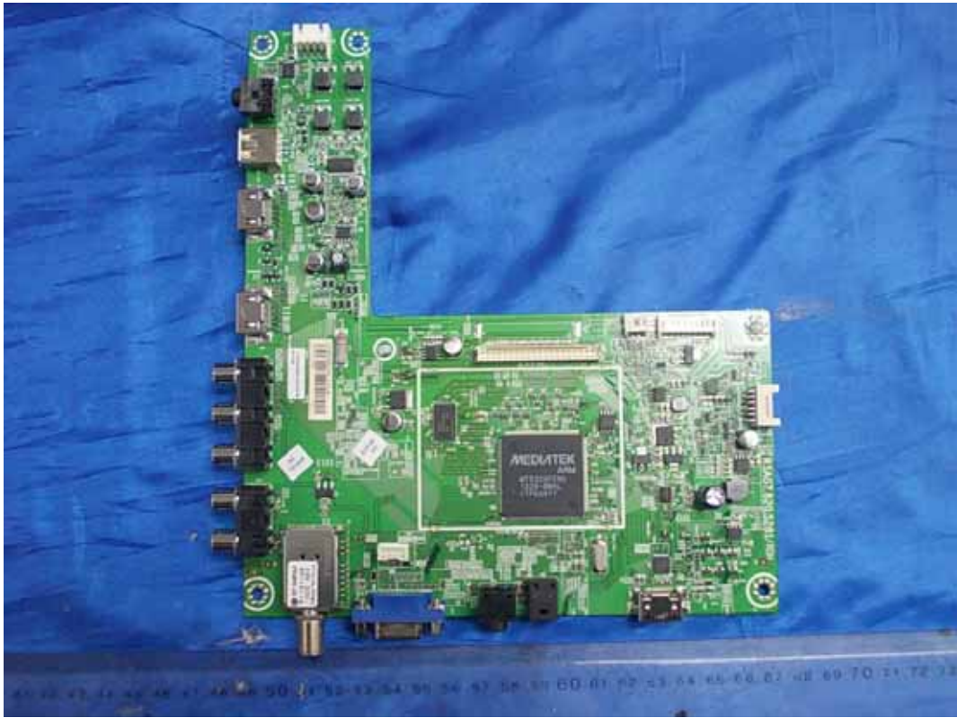
FIGURE 5 LED LCD TV (M/N: LTDN46K360MUS) MAIN BOARD (COMPONENT SIDE)
