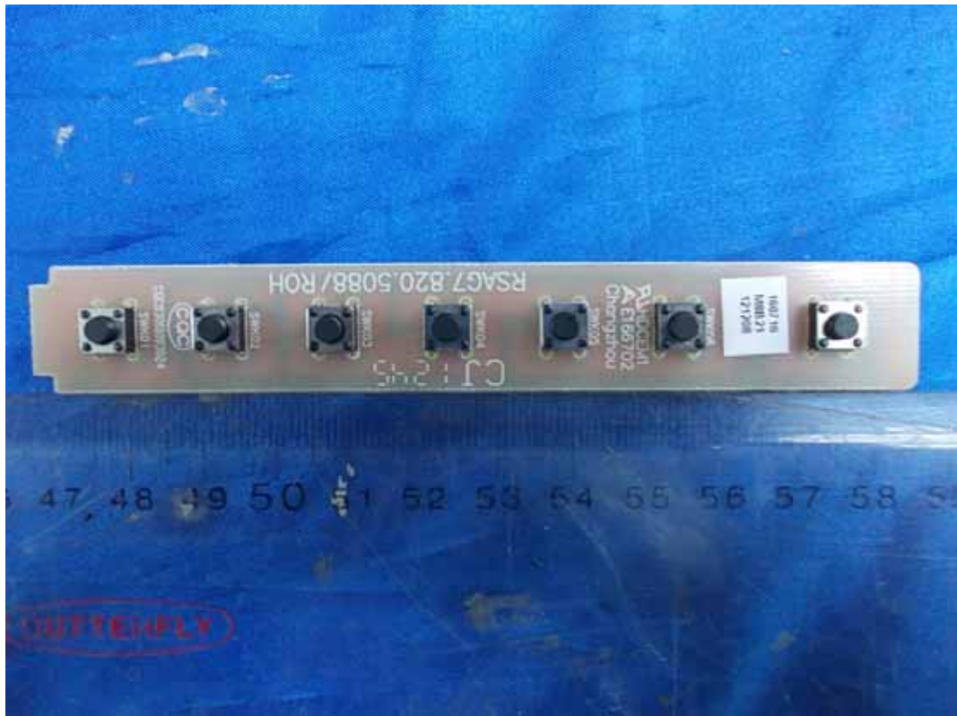
FIGURE 10 LED LCD TV (M/N: LTDN46K360MUS) KEY BOARD (COMPONENT SIDE)
