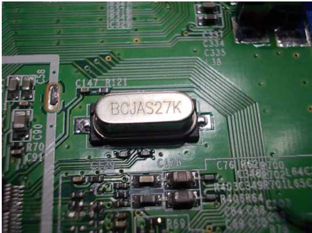
FIGURE 9 LED LCD TV (M/N: LTDN46K360MUS) CRYSTAL #1 ON MAIN BOARD
