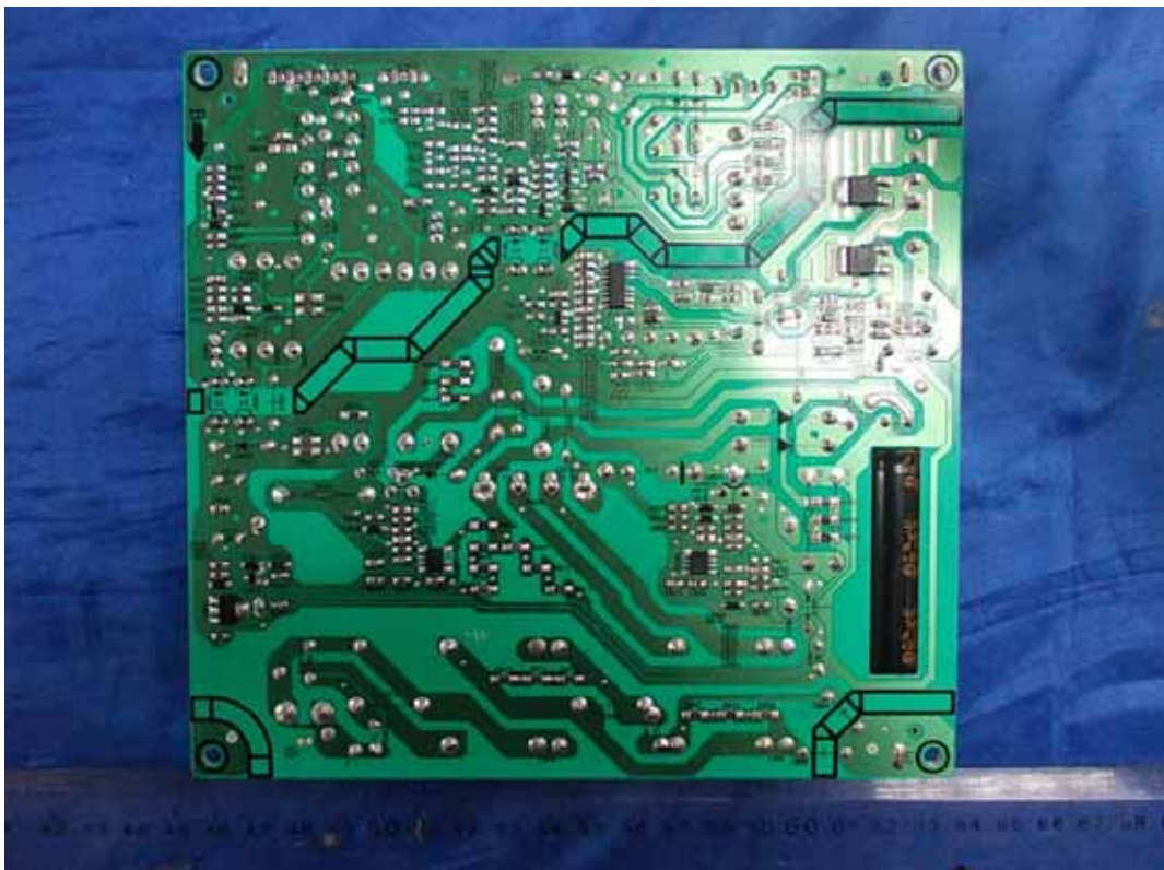
FIGURE 4 LED LCD TV (M/N: LTDN46K360MUS) POWER BOARD (SOLDERED SIDE)
