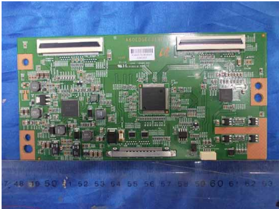
FIGURE 14 LED LCD TV (M/N: LTDN46K360MUS) LCD PANEL CONTROL BOARD (COMPONENT SIDE)
