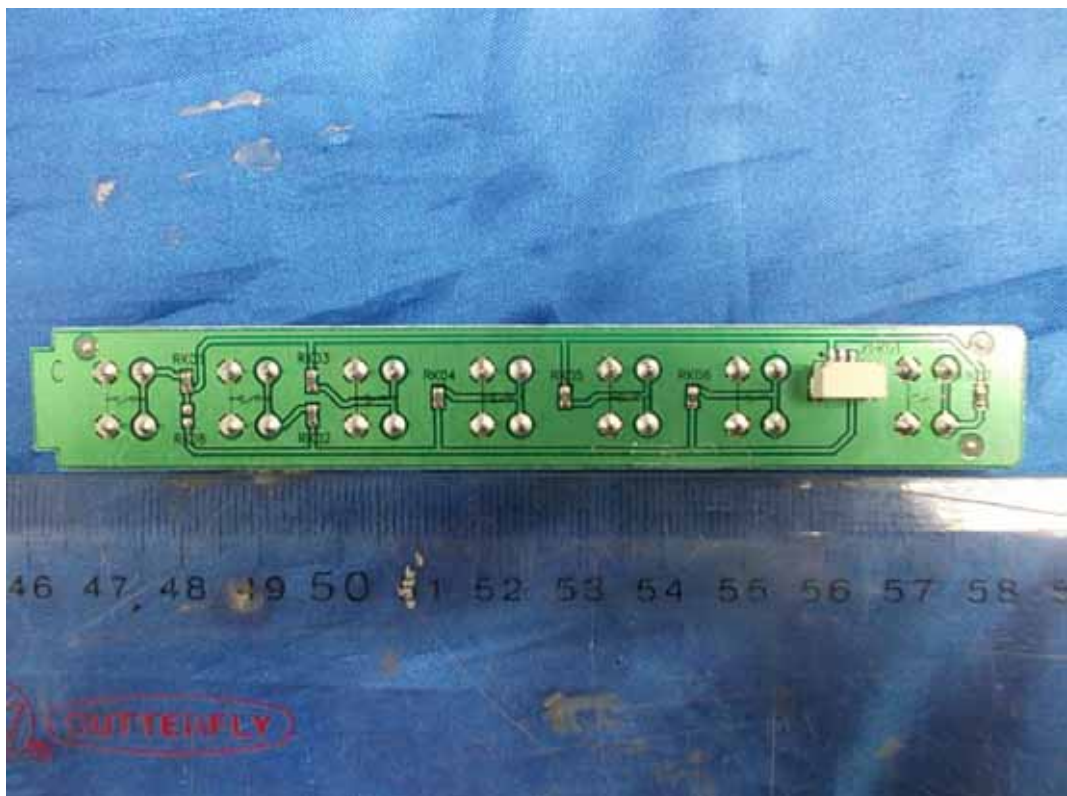
FIGURE 11 LED LCD TV (M/N: LTDN46K360MUS) KEY BOARD (SOLDERED SIDE)
