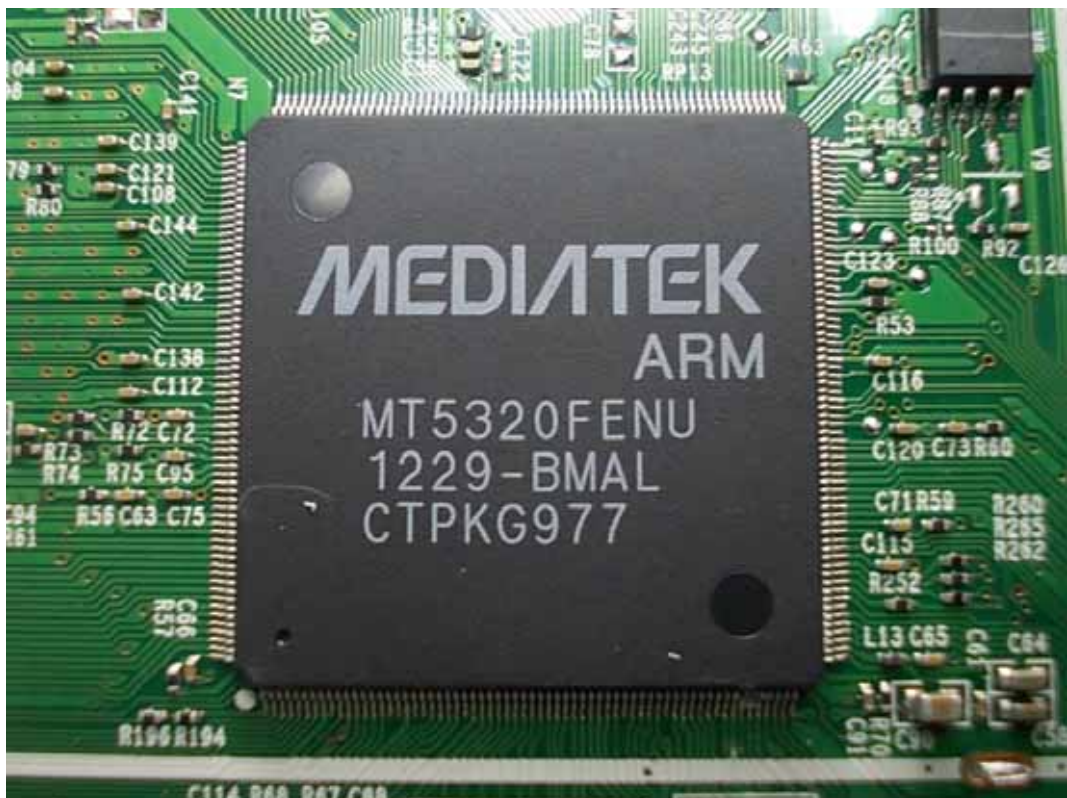
FIGURE 8 LED LCD TV (M/N: LTDN46K360MUS) CHIP #1 ON MAIN BOARD
