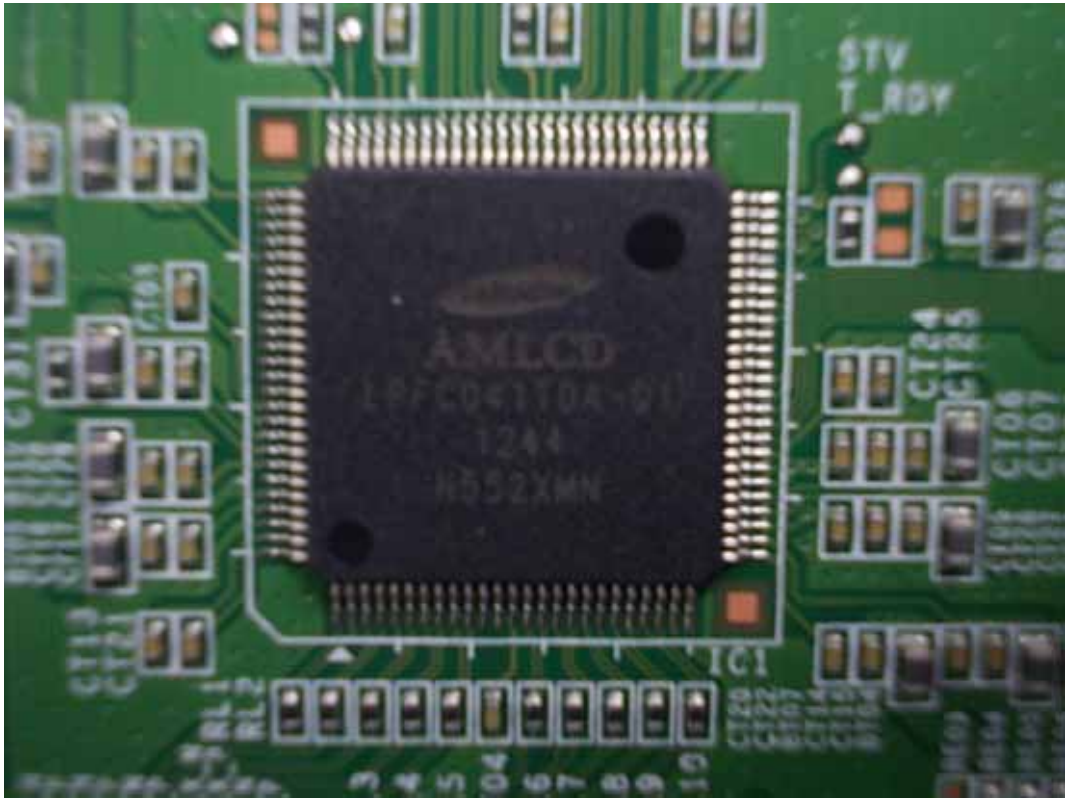
FIGURE 16 LED LCD TV (M/N: LTDN46K360MUS) CHIP ON LCD PANEL CONTROL BOARD
