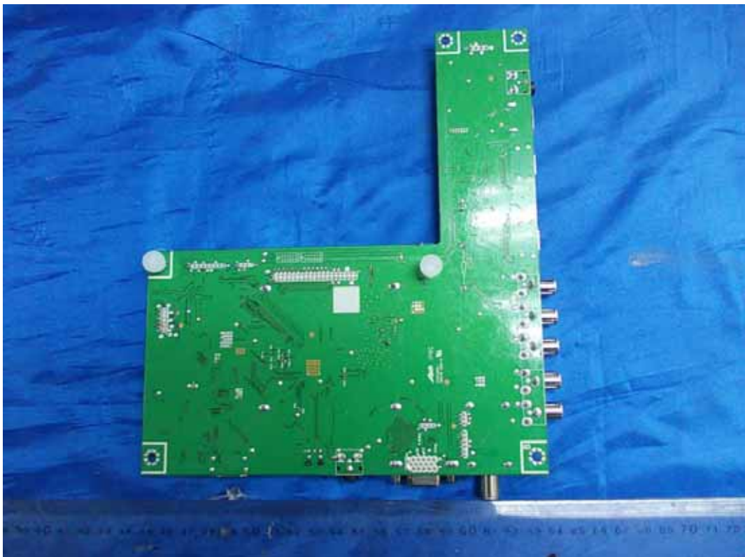
FIGURE 6 LED LCD TV (M/N: LTDN46K360MUS) MAIN BOARD (SOLDERED SIDE)
