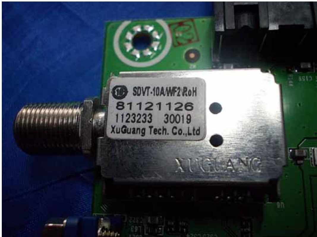
FIGURE 7 LED LCD TV (M/N: LTDN46K360MUS) TUNER ON MAIN BOARD
