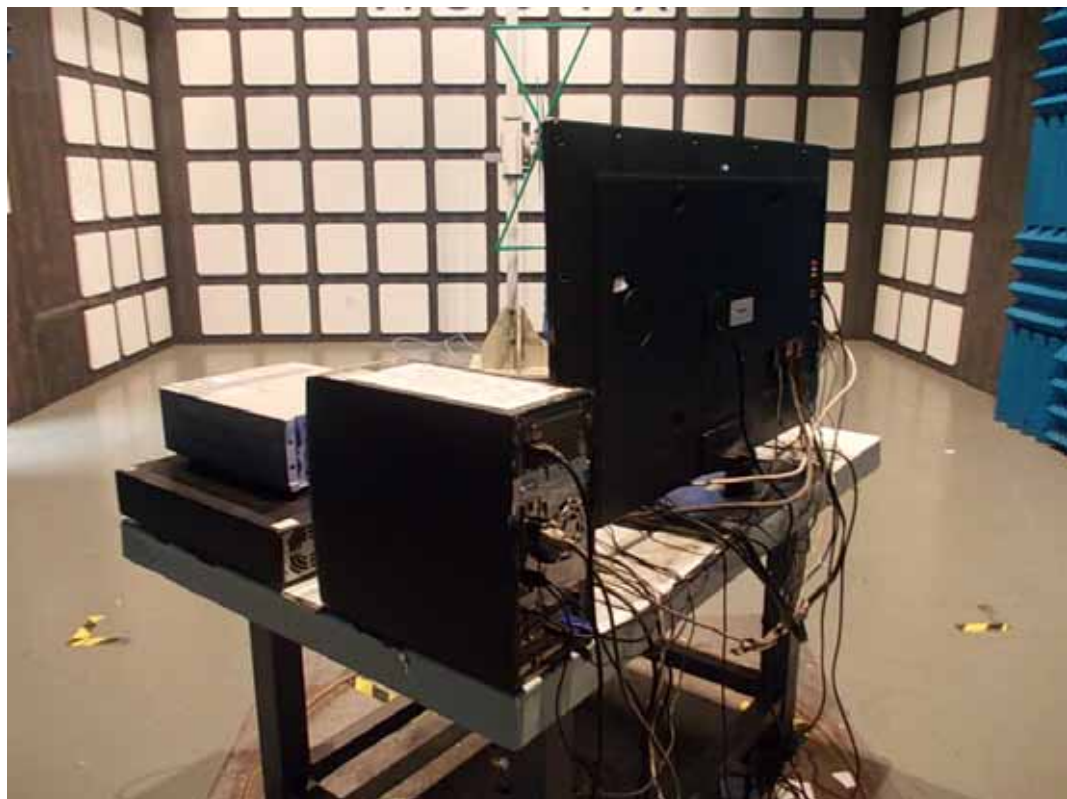
SETUP WITH MAXIMUM DETECTED EMISSION AT VERTICAL POLARIZATION (TEST MODE: USB PLAY)
