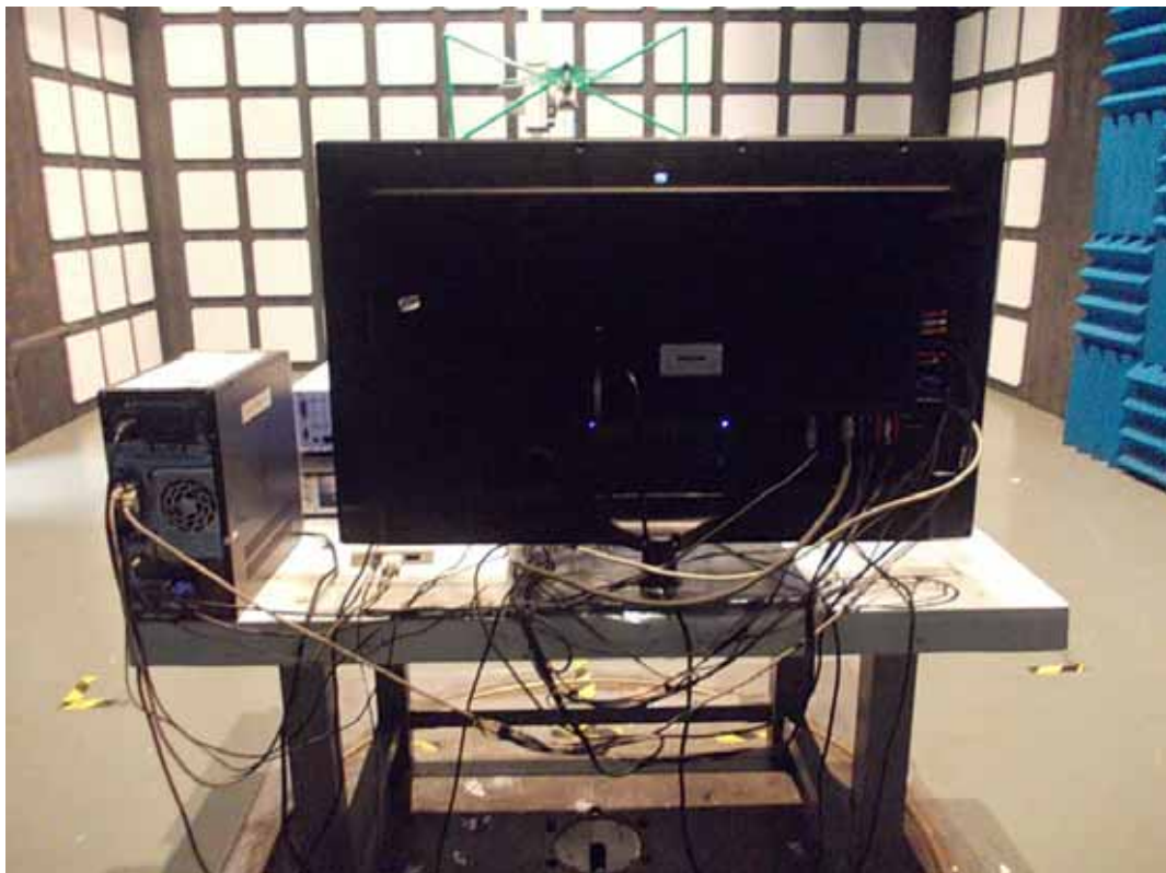
BACK VIEW OF RADIATED EMISSION TEST
