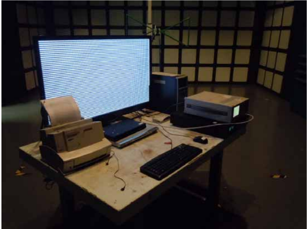
SETUP WITH MAXIMUM DETECTED EMISSION AT HORIZONTAL POLARIZATION (TEST MODE: D-SUB 1024*768@60Hz)
