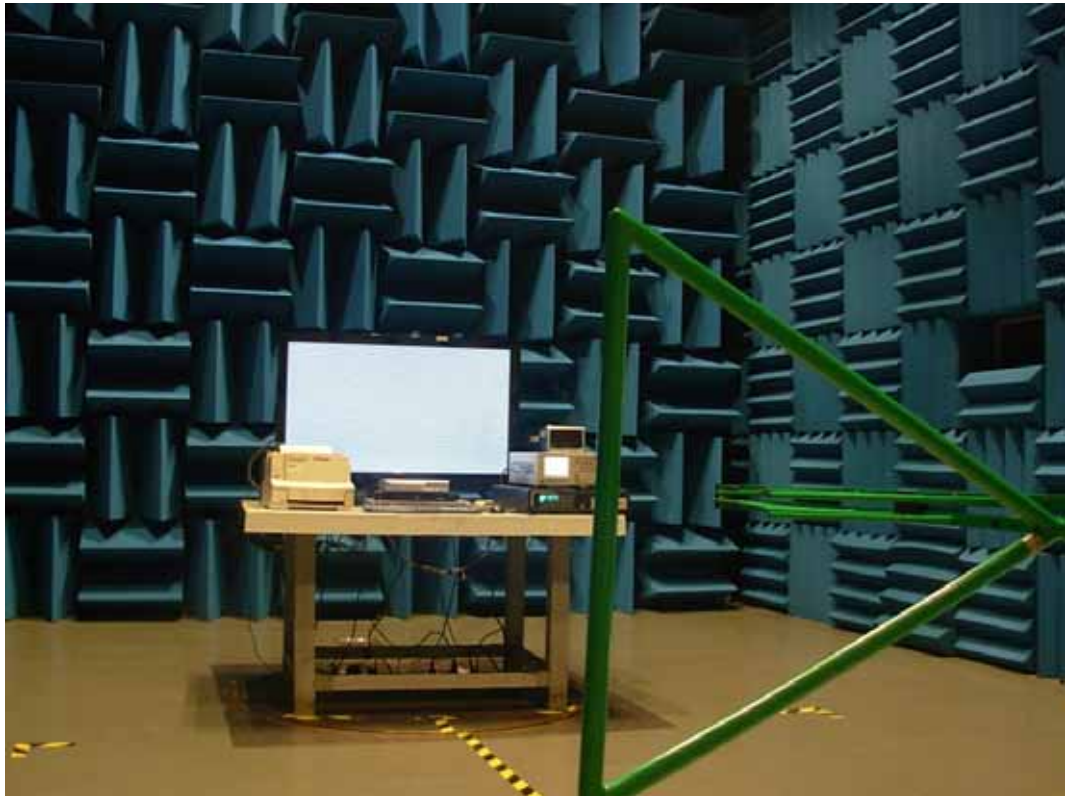
FRONT VIEW OF RADIATED EMISSION TEST
