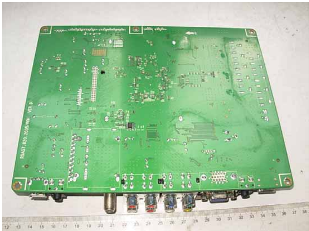
FIGURE 6 LCD TV (M/N: LTDN46V86US) MAIN BOARD (SOLDERED SIDE)
