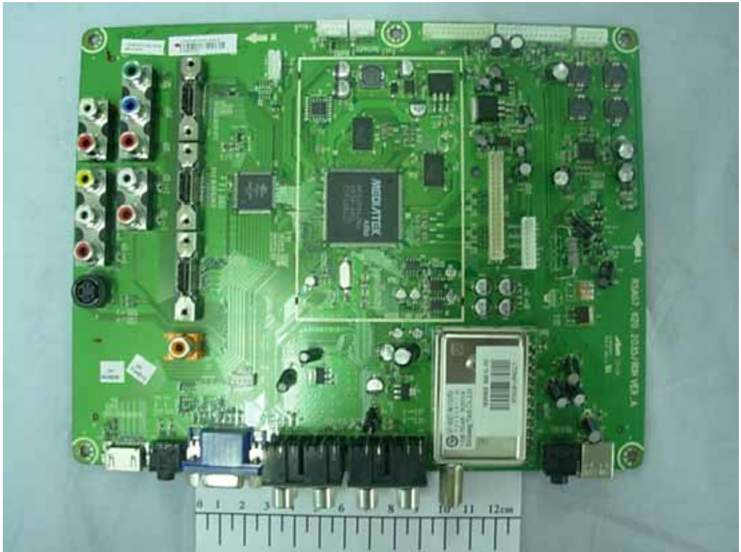
FIGURE 12 LCD TV (M/N: 47LC55S240V87) MAIN BOARD (COMPONENT SIDE)
