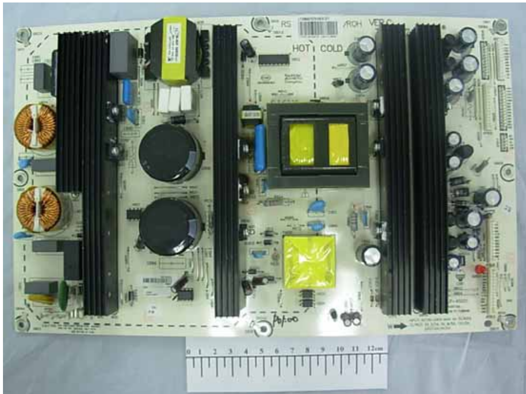
FIGURE 10 LCD TV (M/N: 47LC55S240V87) POWER BOARD (COMPONENT SIDE)
