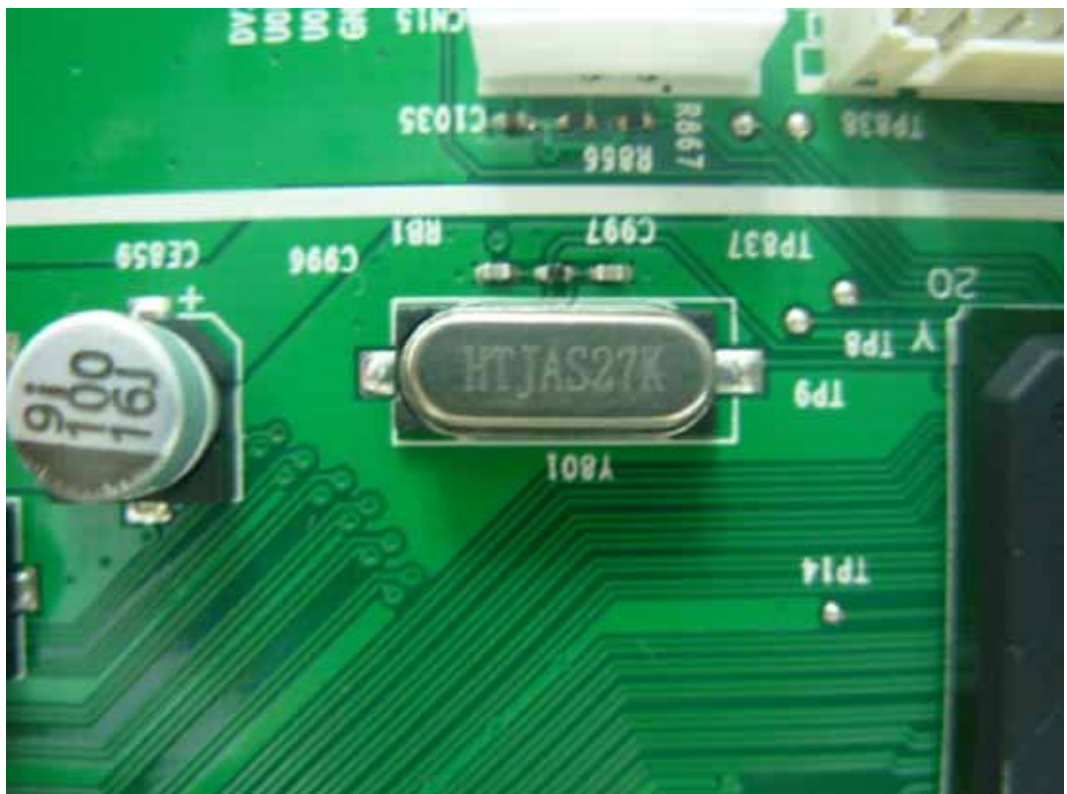
FIGURE 21 LCD TV (M/N: 47LC55S240V87) CRYSTAL ON LCD PANEL CONTROL BOARD
