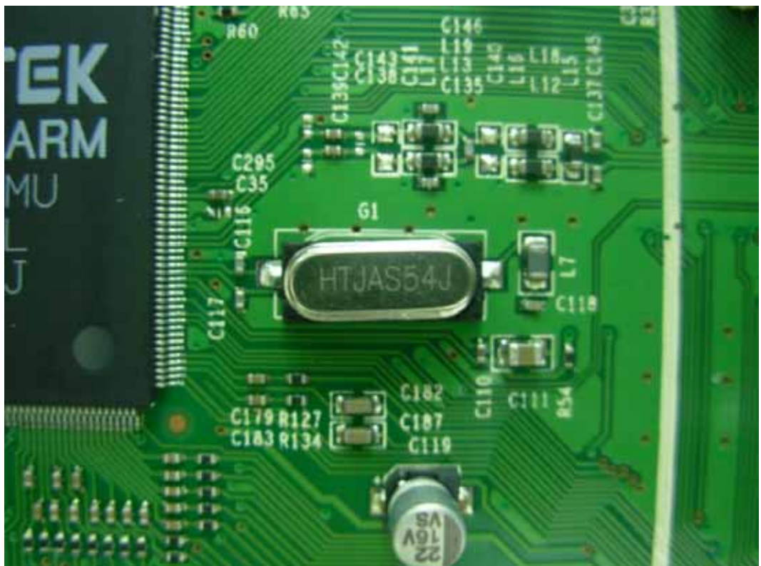
FIGURE 17 LCD TV (M/N: 47LC55S240V87) CRYSTAL ON MAIN BOARD
