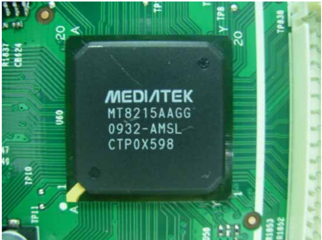
FIGURE 20 LCD TV (M/N: 47LC55S240V87) CHIP ON LCD PANEL CONTROL BOARD
