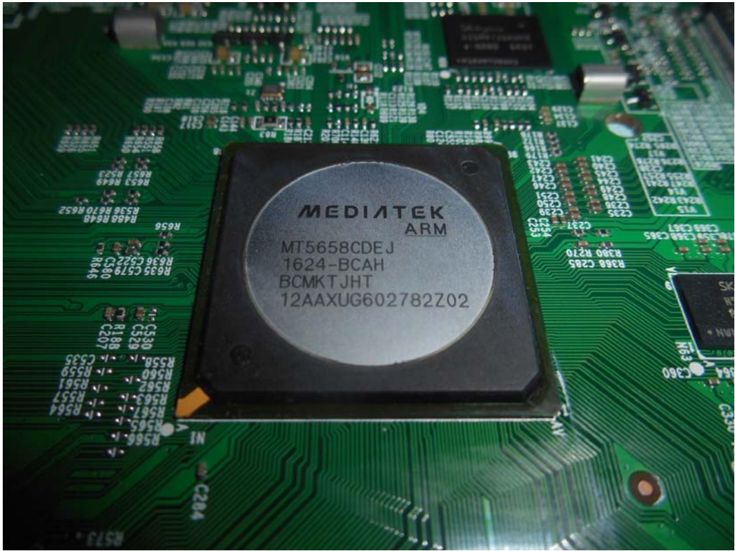
FIGURE 9 LED LCD TV (M/N: LC-43P7000U) CHIP AND CRYSTAL ON MAIN BOARD
