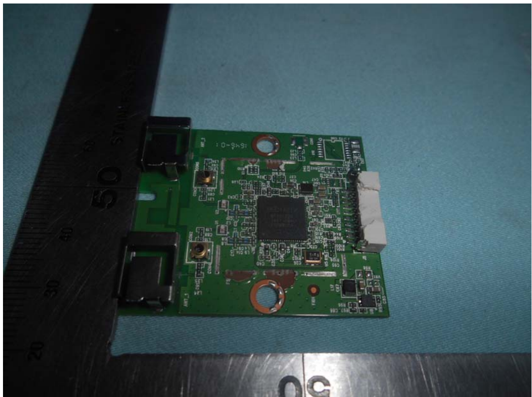
FIGURE 16 LED LCD TV (M/N: LC-43P7000U) CHIP AND CRYSTAL ON RF BOARD
