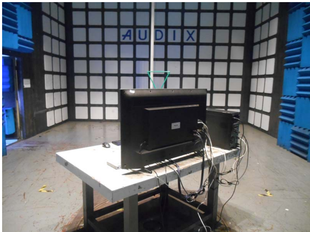
SETUP WITH MAXIMUM DETECTED EMISSION AT VERTICAL POLARIZATION (TEST MODE HDMI1 1280*1024@60Hz & 1kHz PLAYING)
