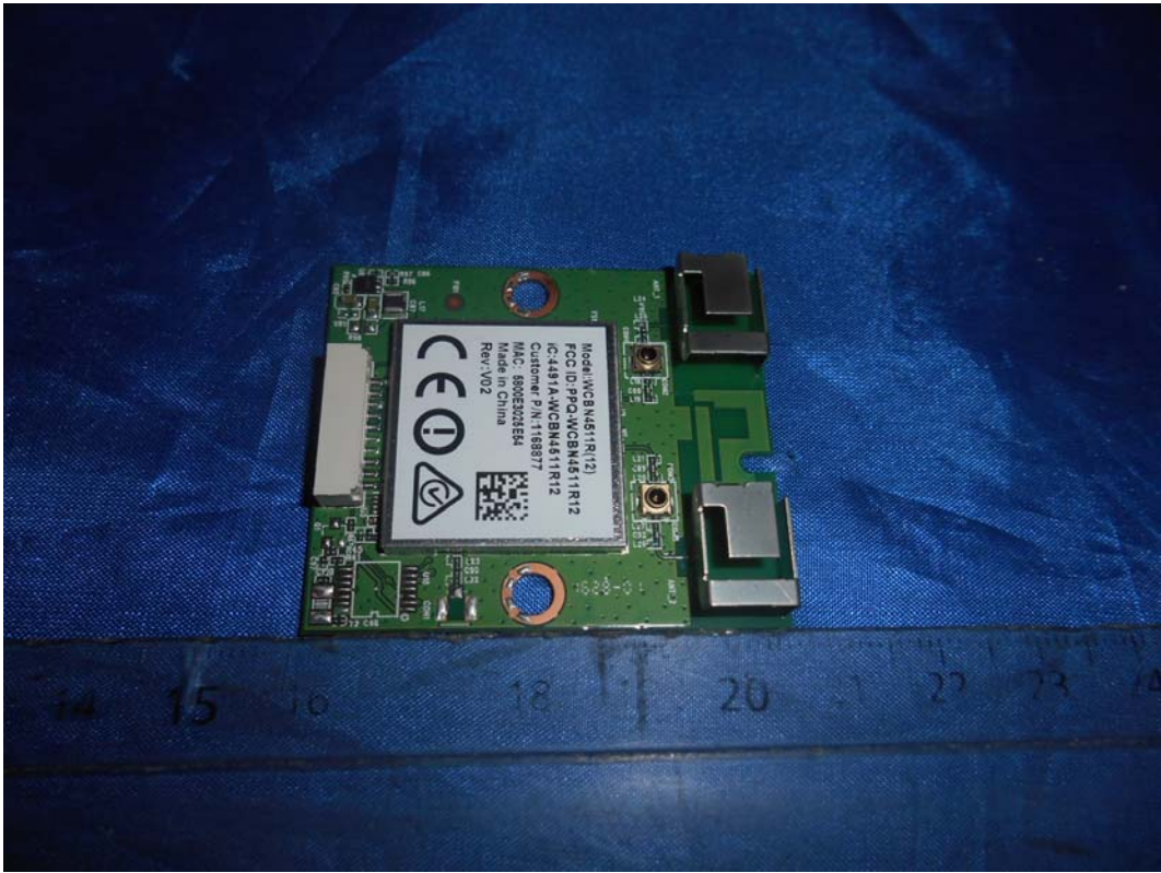
FIGURE 9 LED LCD TV (M/N: 43H6D) RF BOARD (COMPONENT SIDE)
