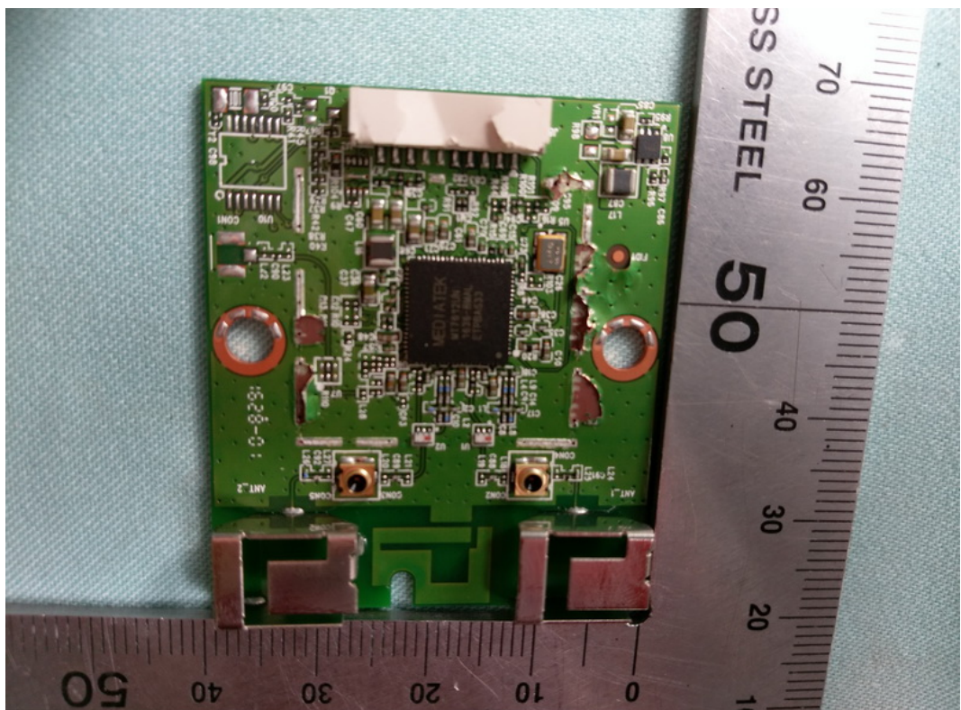
FIGURE 12 LED LCD TV (M/N: 43H6D) CHIP AND CRYSTAL ON RF BOARD
