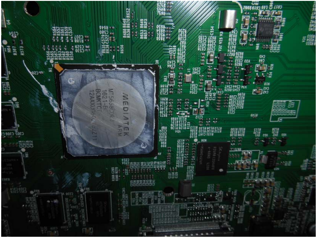
FIGURE 4 LED LCD TV (M/N: 43H6D) CHIP AND CRYSTAL ON MAIN BOARD
