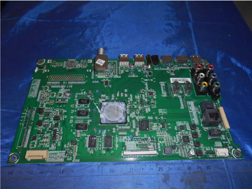
FIGURE 2 LED LCD TV (M/N: 43H6D) MAIN BOARD (COMPONENT SIDE)
