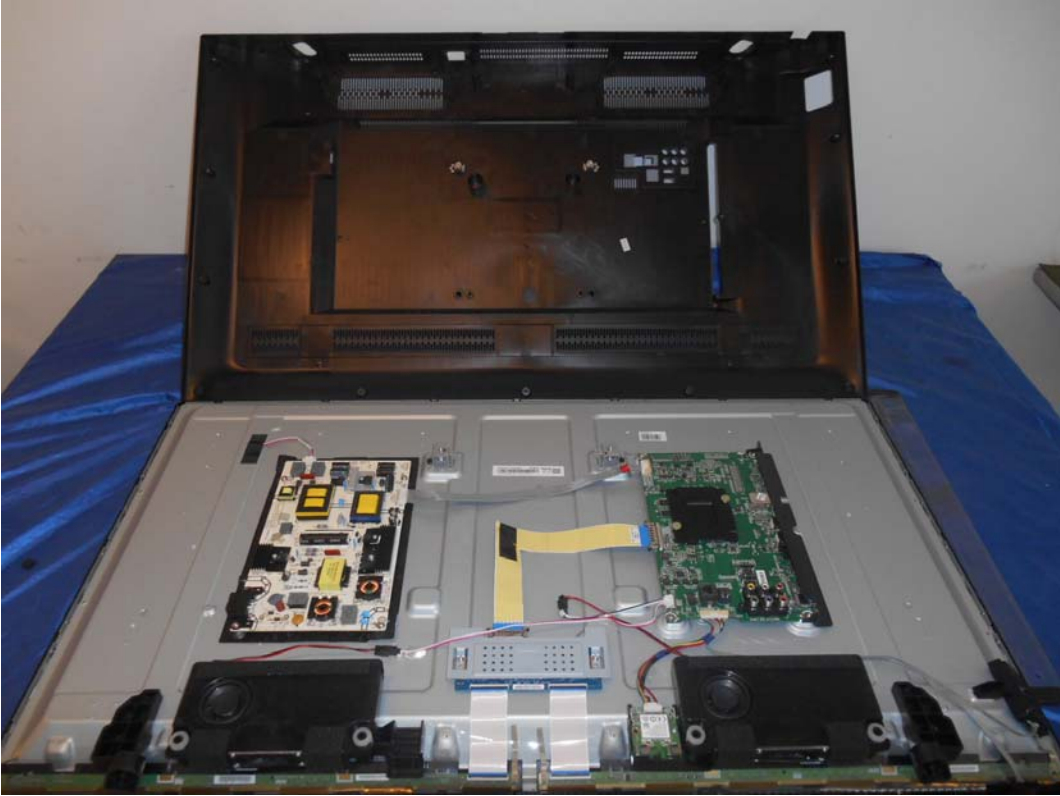
FIGURE 1 LED LCD TV (M/N: 43H6D) COVER REMOVED
