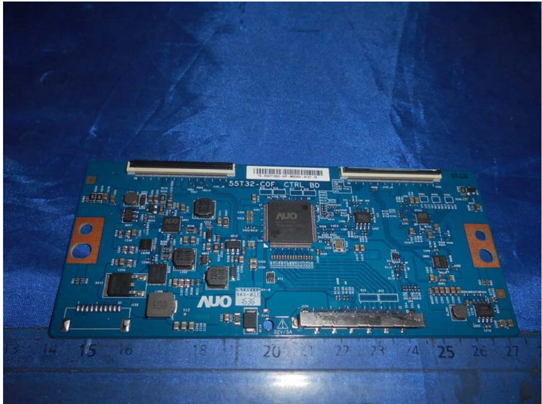
FIGURE 6 LED LCD TV (M/N: 43H6D) PANEL MAIN BOARD (COMPONENT SIDE)
