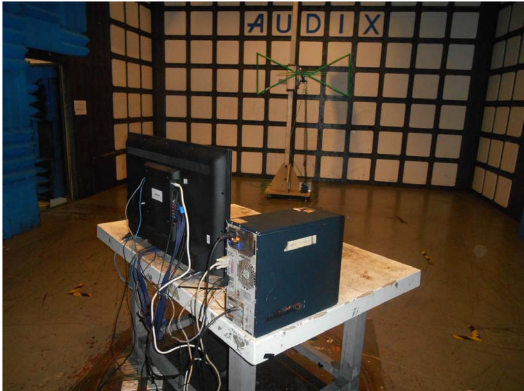
SETUP WITH MAXIMUM DETECTED EMISSION AT HORIZONTAL POLARIZATION (TEST MODE: HDMI 1920*1080@60HZ & 1KHZ PLAYING)
