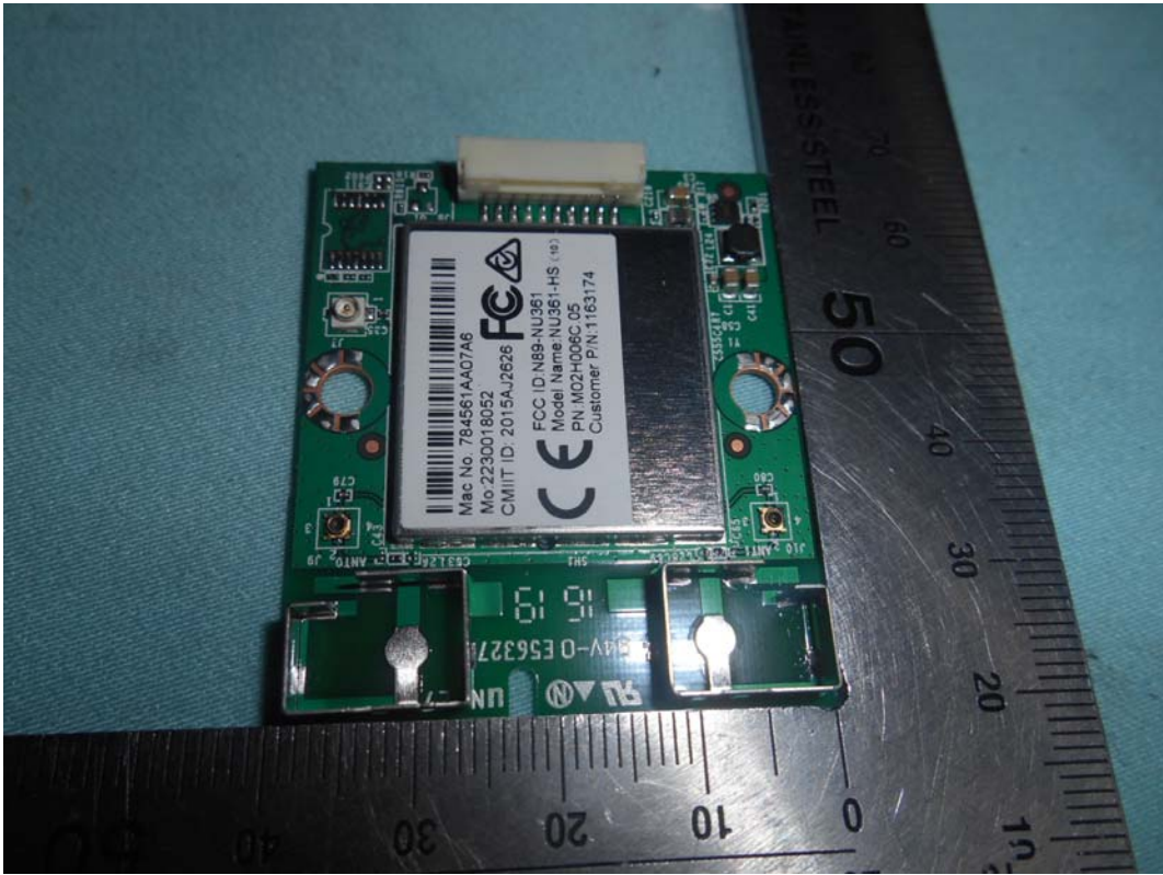
FIGURE 13 LED LCD TV (M/N: LC-43N6100U) RF BOARD (COMPONENT SIDE)
