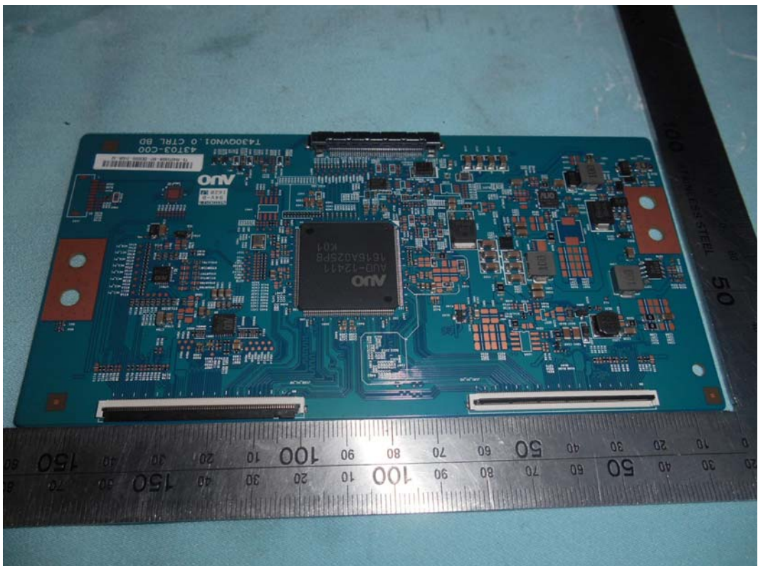
FIGURE 10 LED LCD TV (M/N: LC-43N6100U) PANEL BOARD (COMPONENT SIDE)
