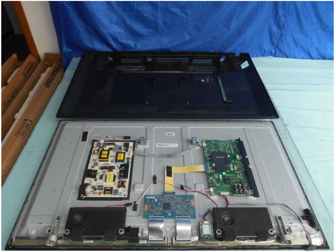
FIGURE 1 LED LCD TV (M/N: LC-43N6100U) COVER REMOVED
